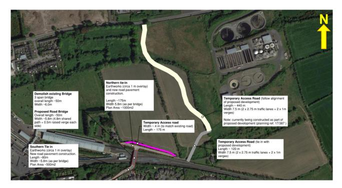
Figure 5-7: Option 1 – New bridge in existing location
