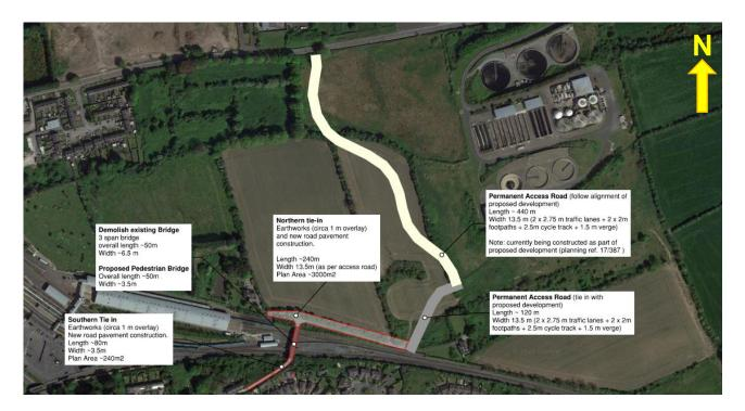
Figure 5-8: Option 5 – Pedestrian bridge with alternative access road from the north
