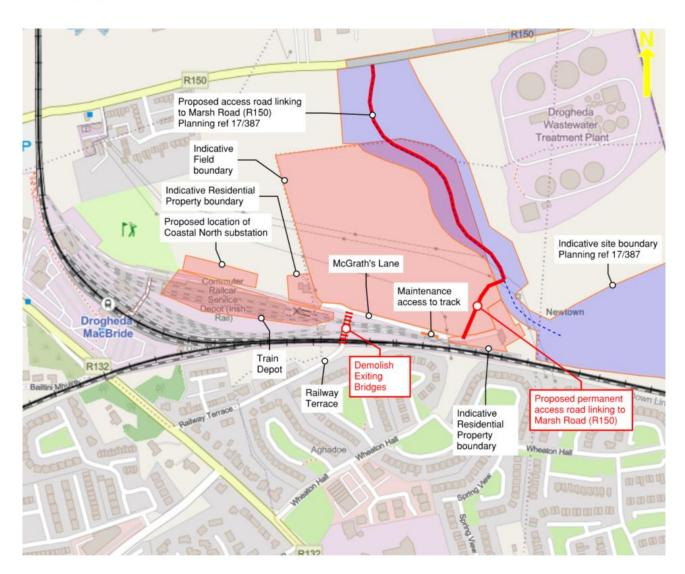
Figure 5-4: Plan view of proposed alternative access road from North
