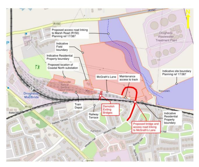
Figure 5-3: Plan view of proposed new bridge in new location
