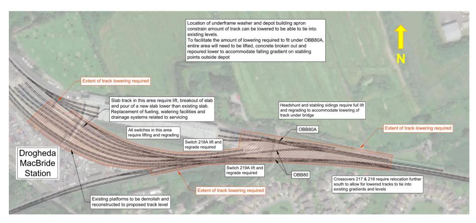
Figure 5-6: Plan view showing impact of track lowering at bridges
