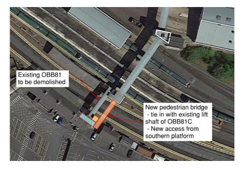
Figure 12: Plan of new bridge in revised location at OBB81
