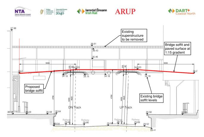
Figure 10: Elevation of proposed superstructure replacement at OBB81
