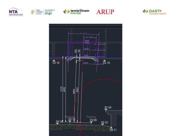
Figure 9: Pantograph envelope utilising a CWH of 4.400 m (UP-track looking north)
