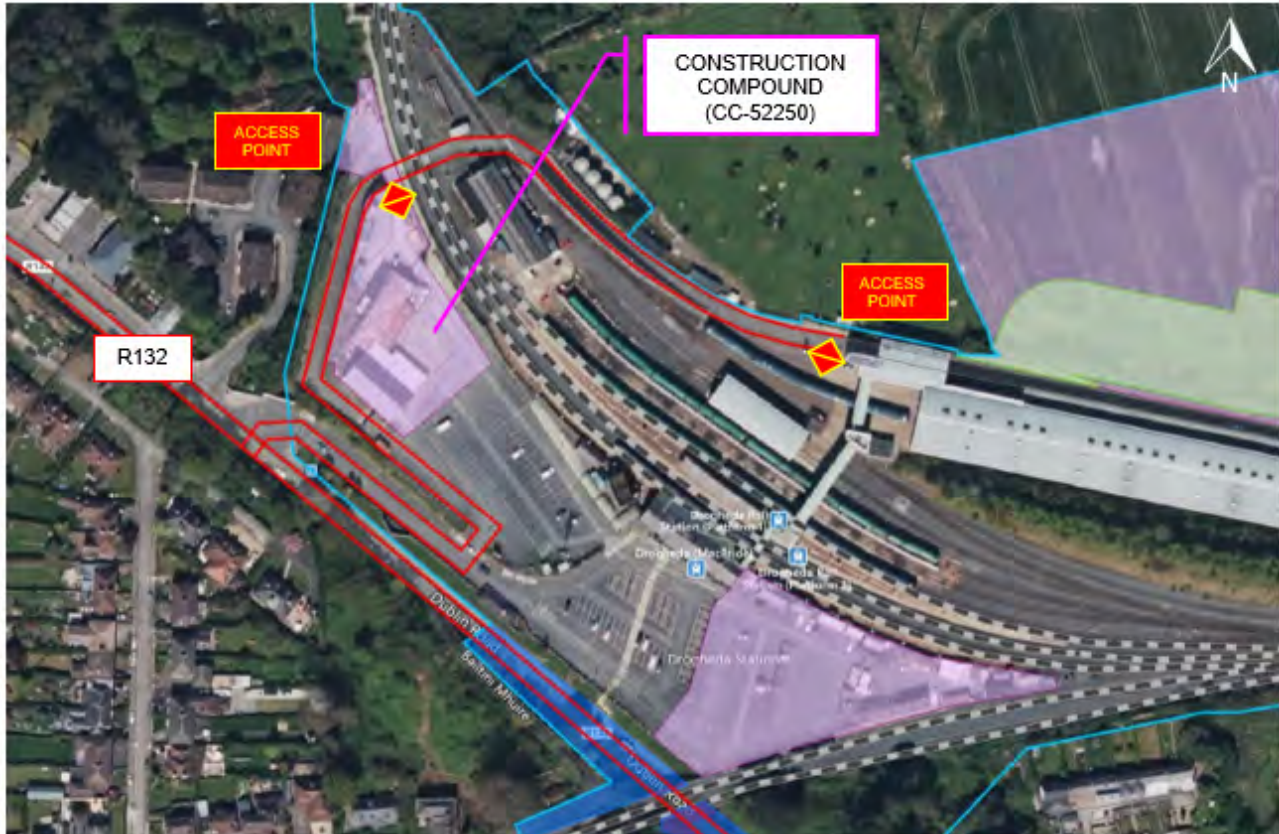
Image 1-26 Depot Construction Compound and Access Routes
