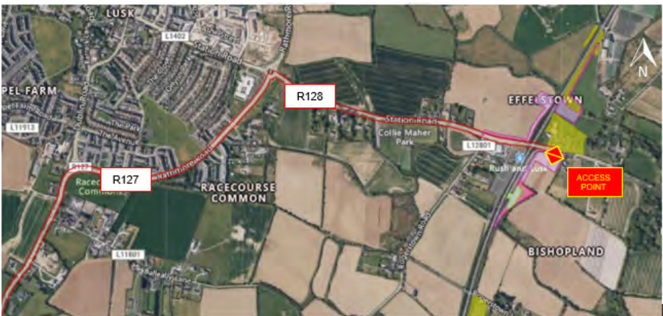
Image 1-7 Rush and Lusk Substation Construction Compound and Access Route
