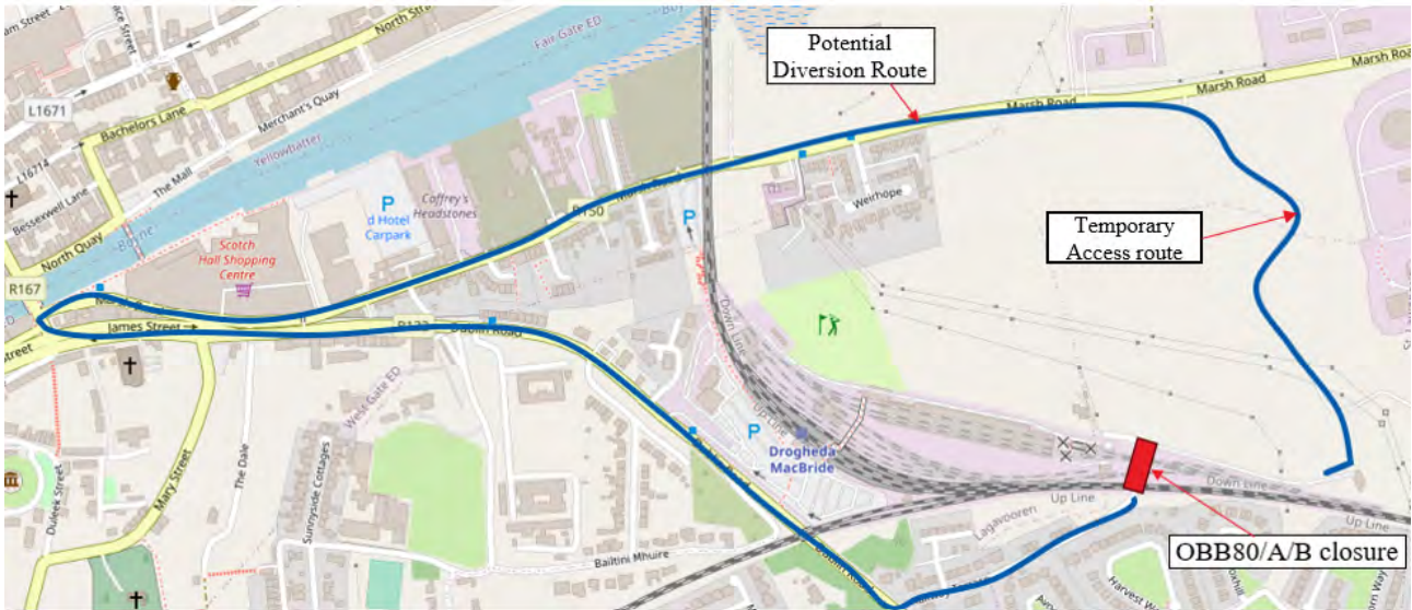
Image 1-32 Potential traffic diversion during OBB80/80A/80B replacement works
