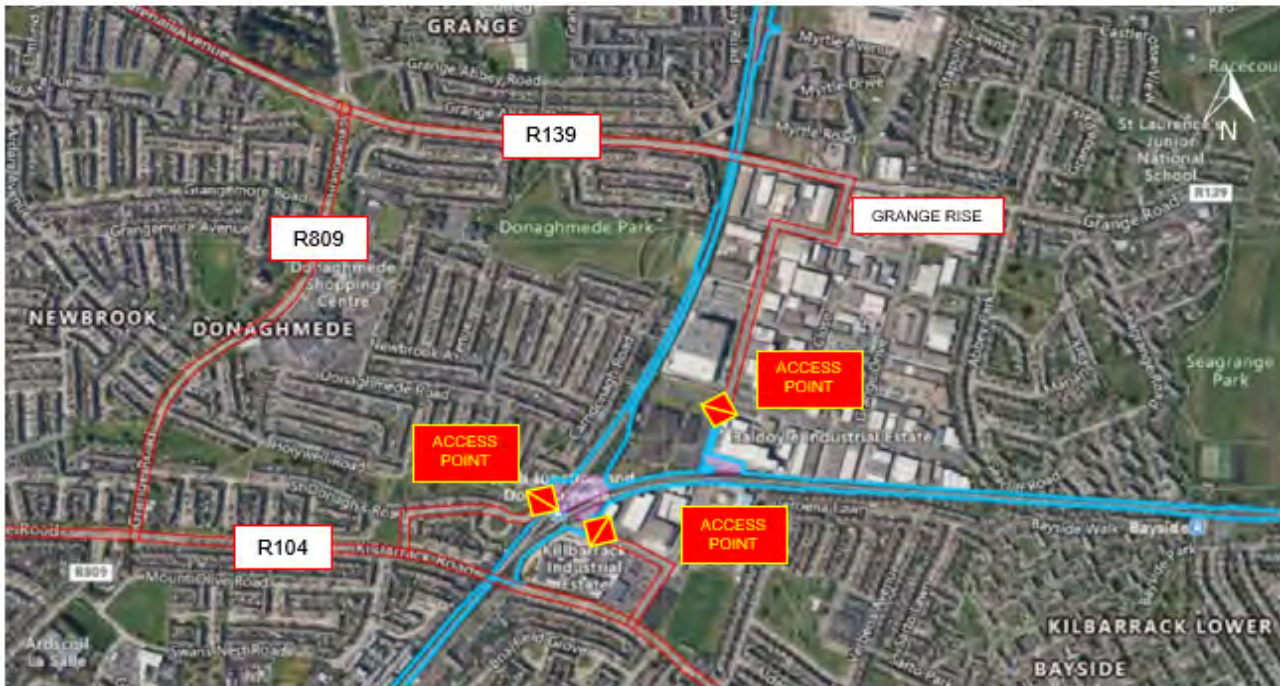
Image 1-2 Howth Junction Proposed Construction Compounds and Access Routes
