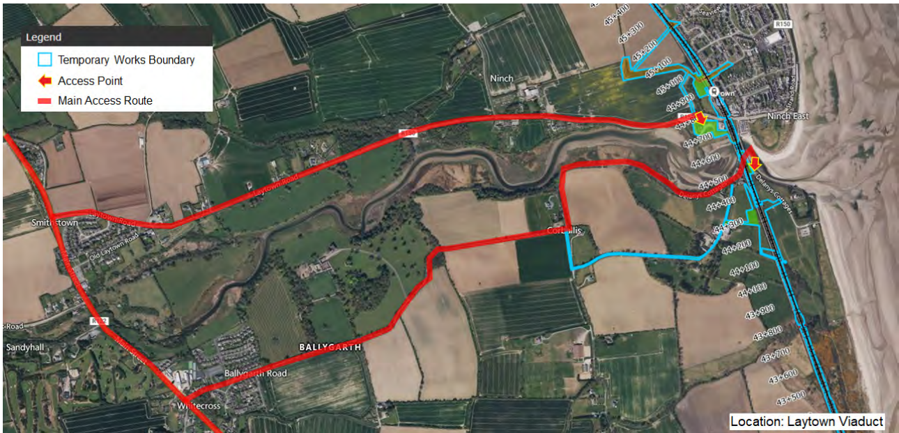
Image 1-17 Access for vehicles to UBB72 Construction Compounds
