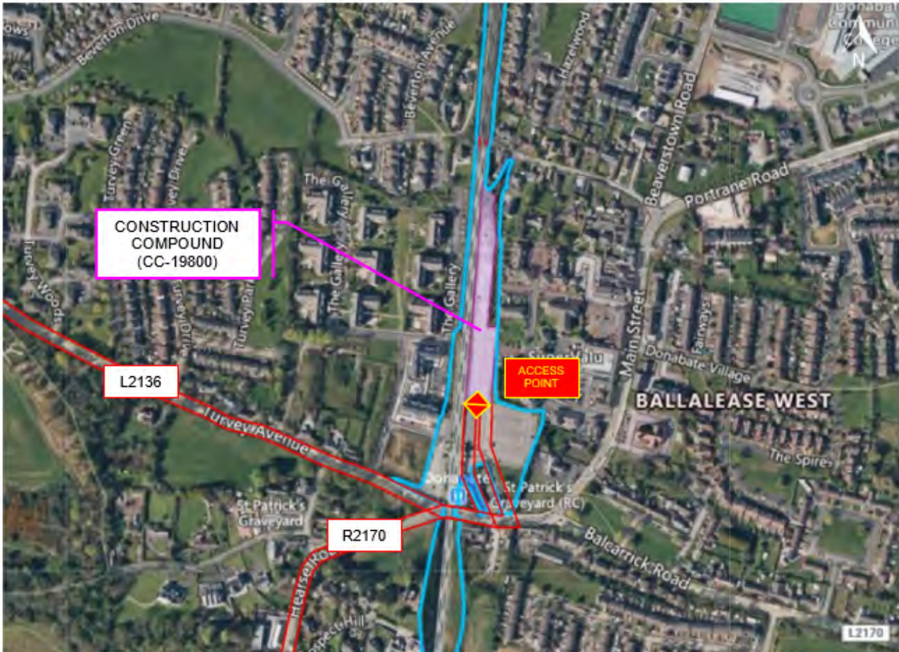
Image 1-14 Donabate Station Line-wide Construction Compound and Access Route
