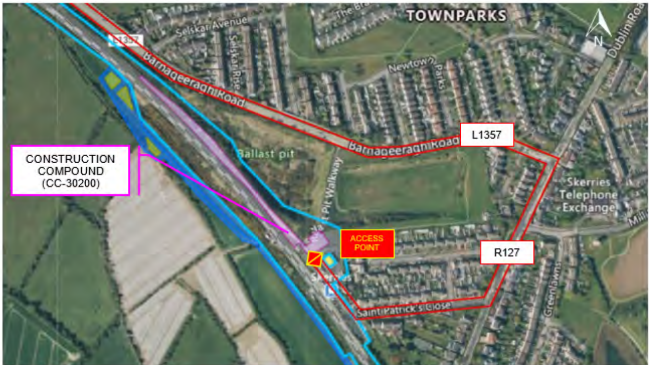
Image 1-15 Skerries Station Line-wide Construction Compound and Access Route
