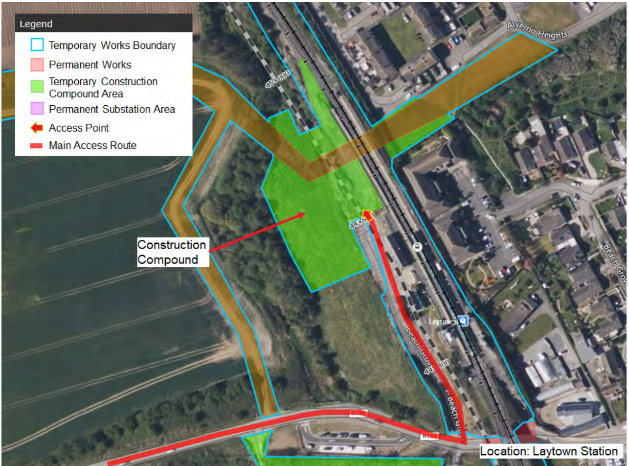
Image 1-21 Laytown Station Line-wide Construction Compound and Access Route
