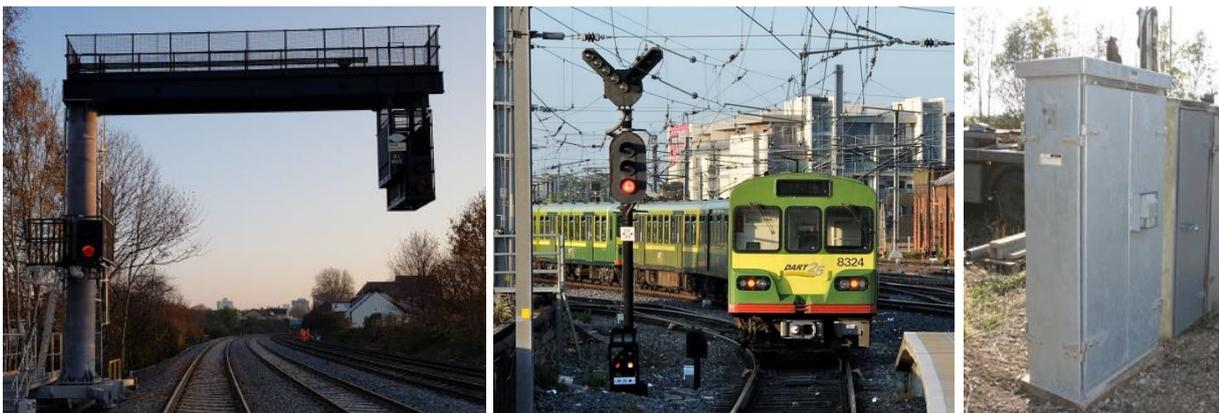
**Figure 4-3 Sample DART+ West signalling infrastructure (cantilever, signal, LOC, from left to right)**
