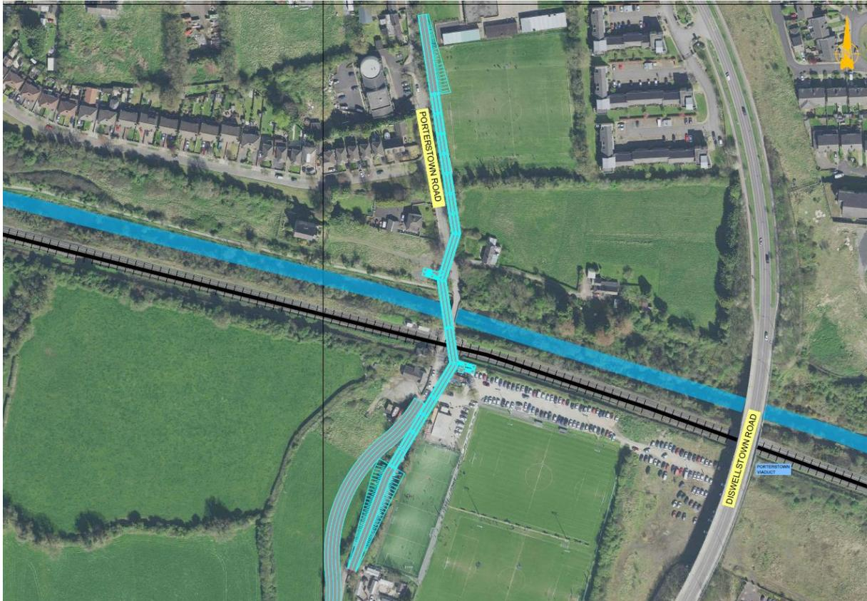
**Figure 3-74 Porterstown Option 3 – Pedestrian and Cycle Bridge – Straight Approach Ramp**
