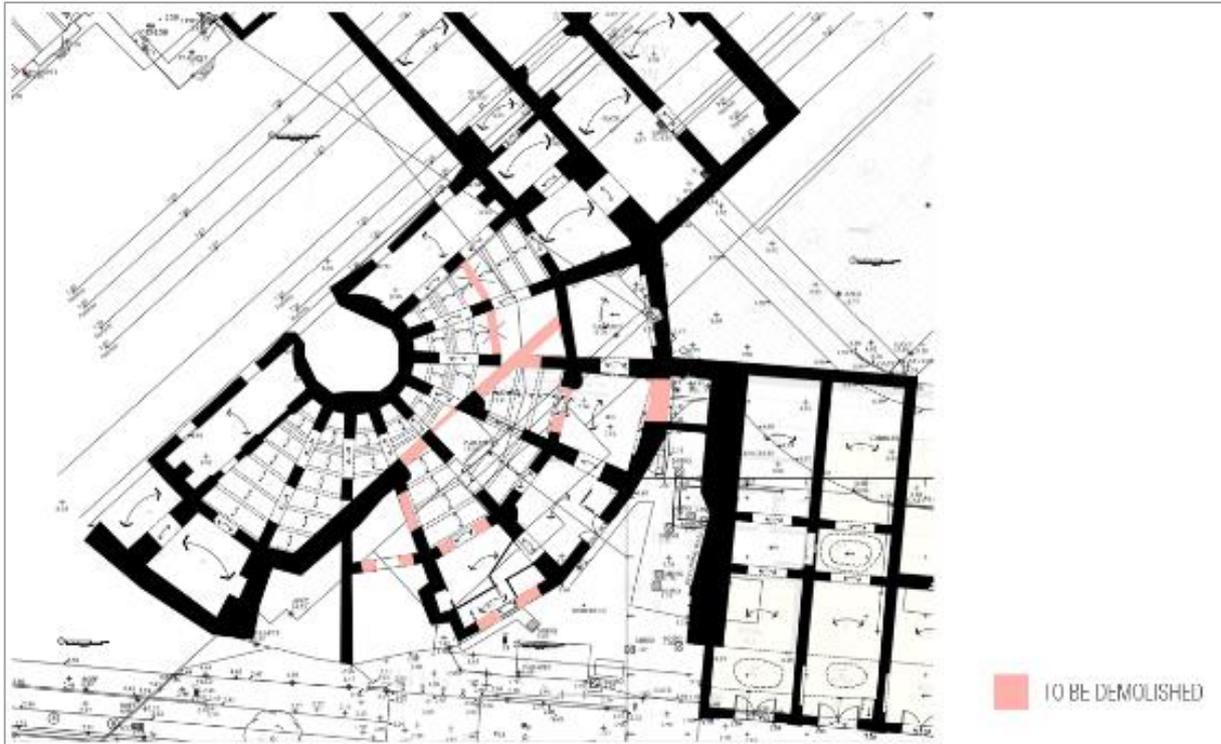
**Figure 3-130 Rotunda Building Structural Modifications Requirements**
