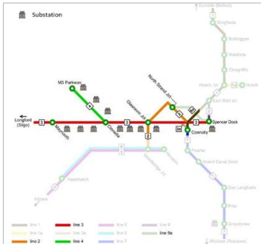
**Figure 3-6 Schematic Layout of Substations along DART+ West**
