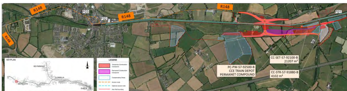
Figure 5-356 Millfarm compounds and haulage route
