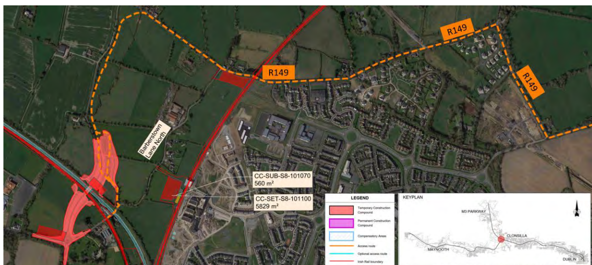
Figure 5-302 Barberstown level crossing compound and haulage route
