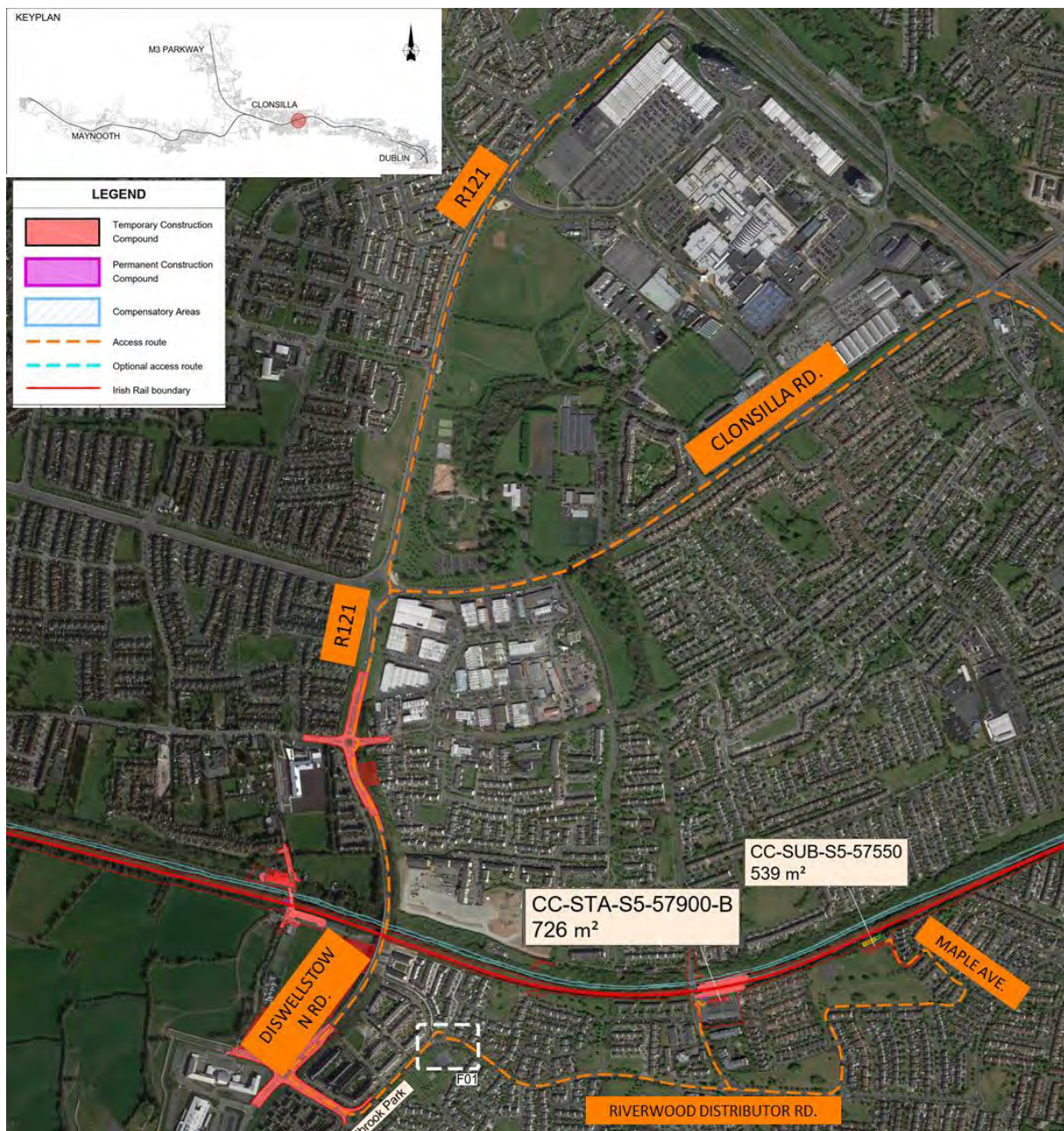
Figure 5-265 Coolmine substation construction compound and haulage route
