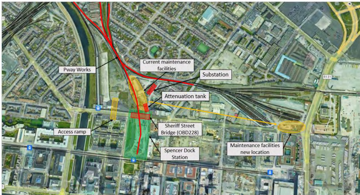
Figure 5-141 Proposed works within Spencer Dock area
