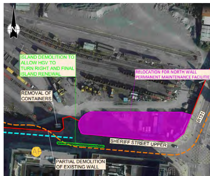
Figure 5-131 Traffic island demolition
