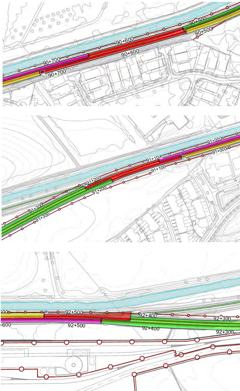
Figure 5-353 Connections at Ch 90+600, Ch 91+200 and Ch 92+500 (red)
