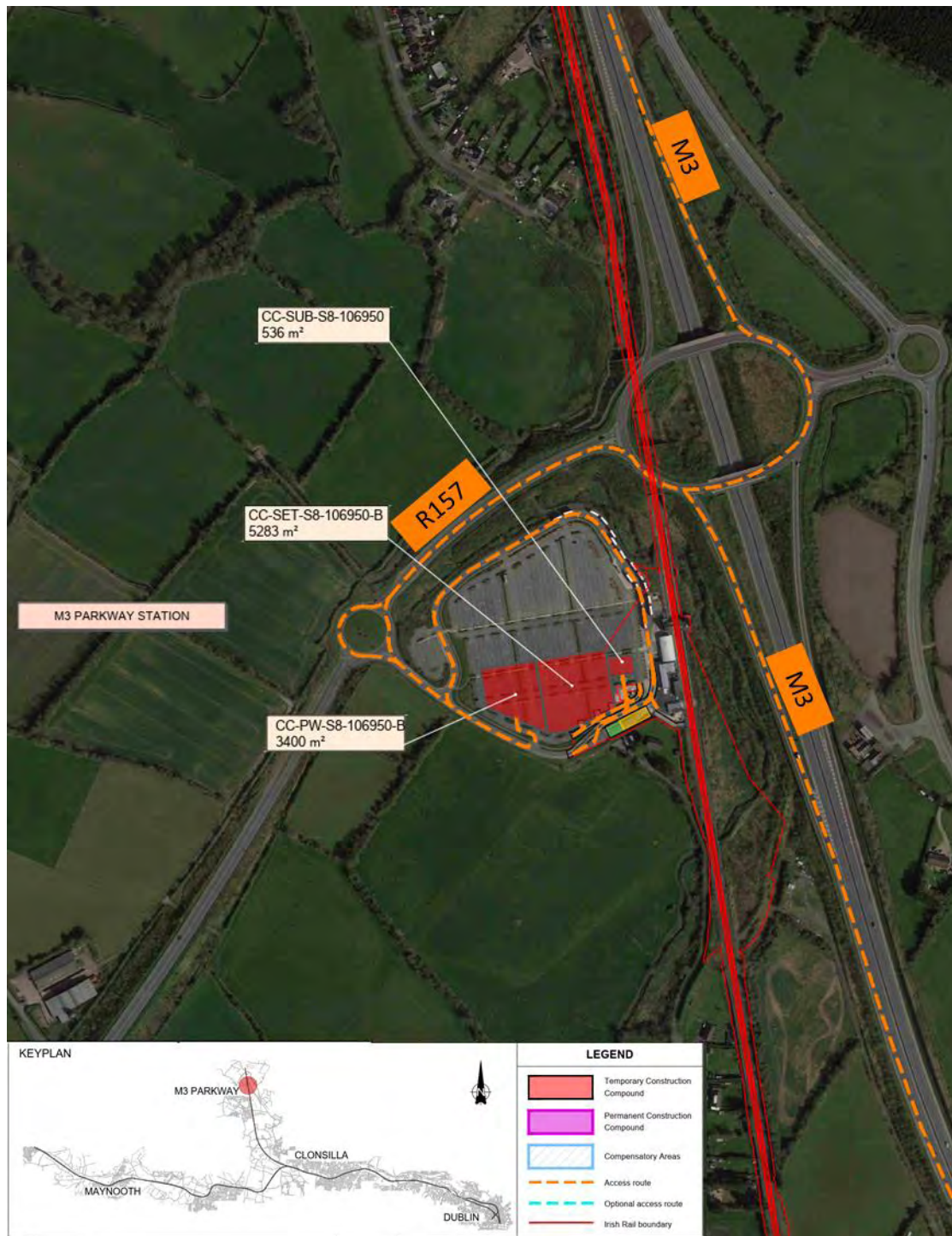
Figure 5-292 M3 Parkway substation compound and haulage route
