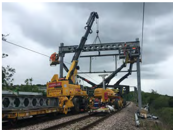
Figure 5-73 Rail-road vehicle examples - pile boring machinery (left) and crane (right)
