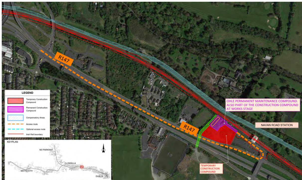
Figure 5-247 Navan Road Station compound and haulage route
