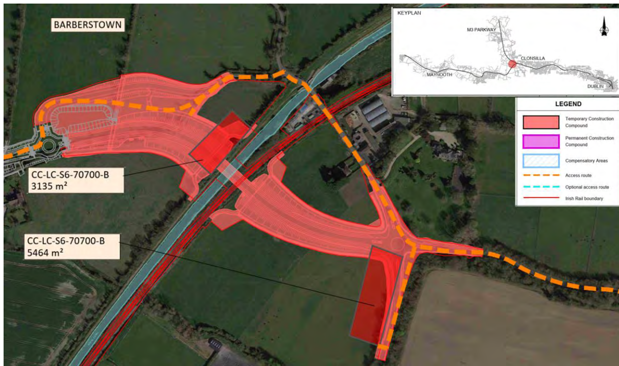
Figure 5-301 Barberstown level crossing compound
