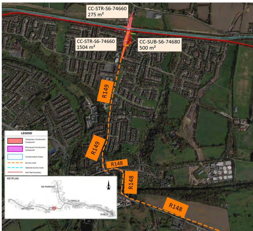
Figure 5-316 Leixlip Confey substation compound and haulage route
