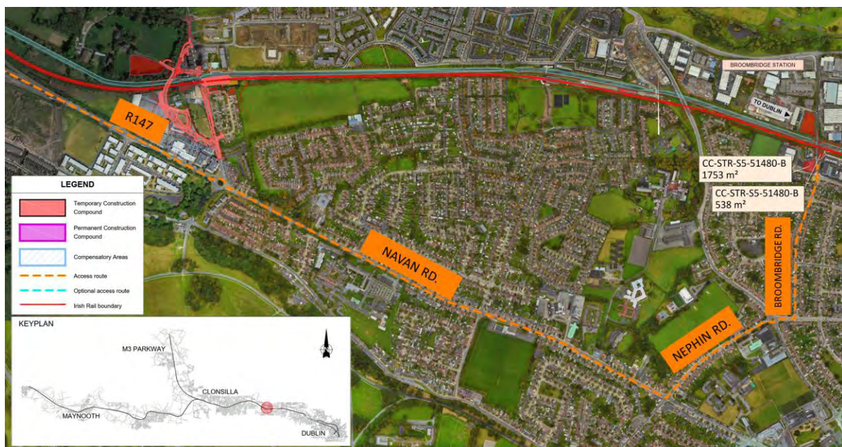
Figure 5-234 OBG5 compound and haulage route
