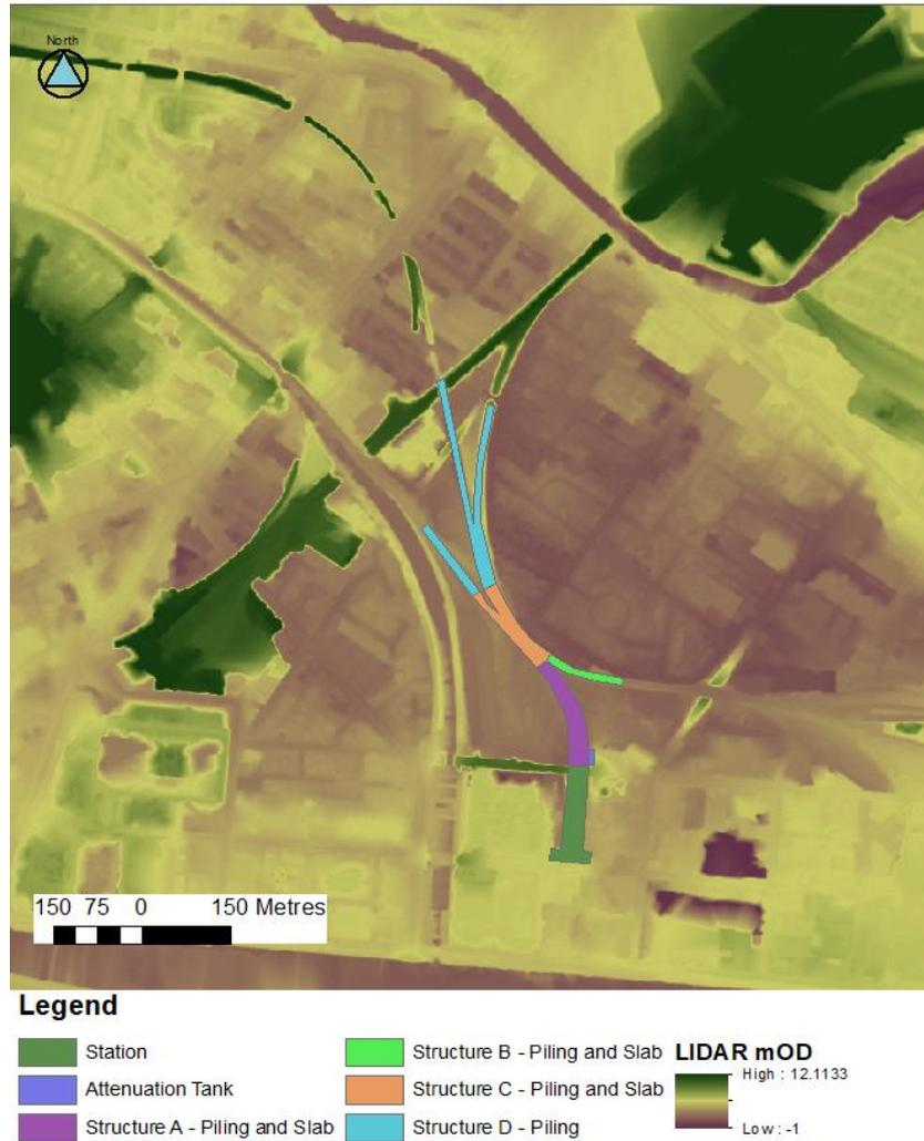
**Figure 11-3 Topography and Piling Requirements in Zone B**
