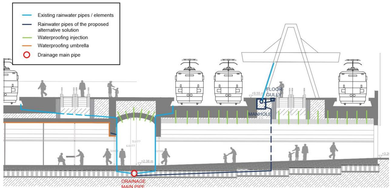
Figure 69 – Rainwater drainage system. Proposed solution
