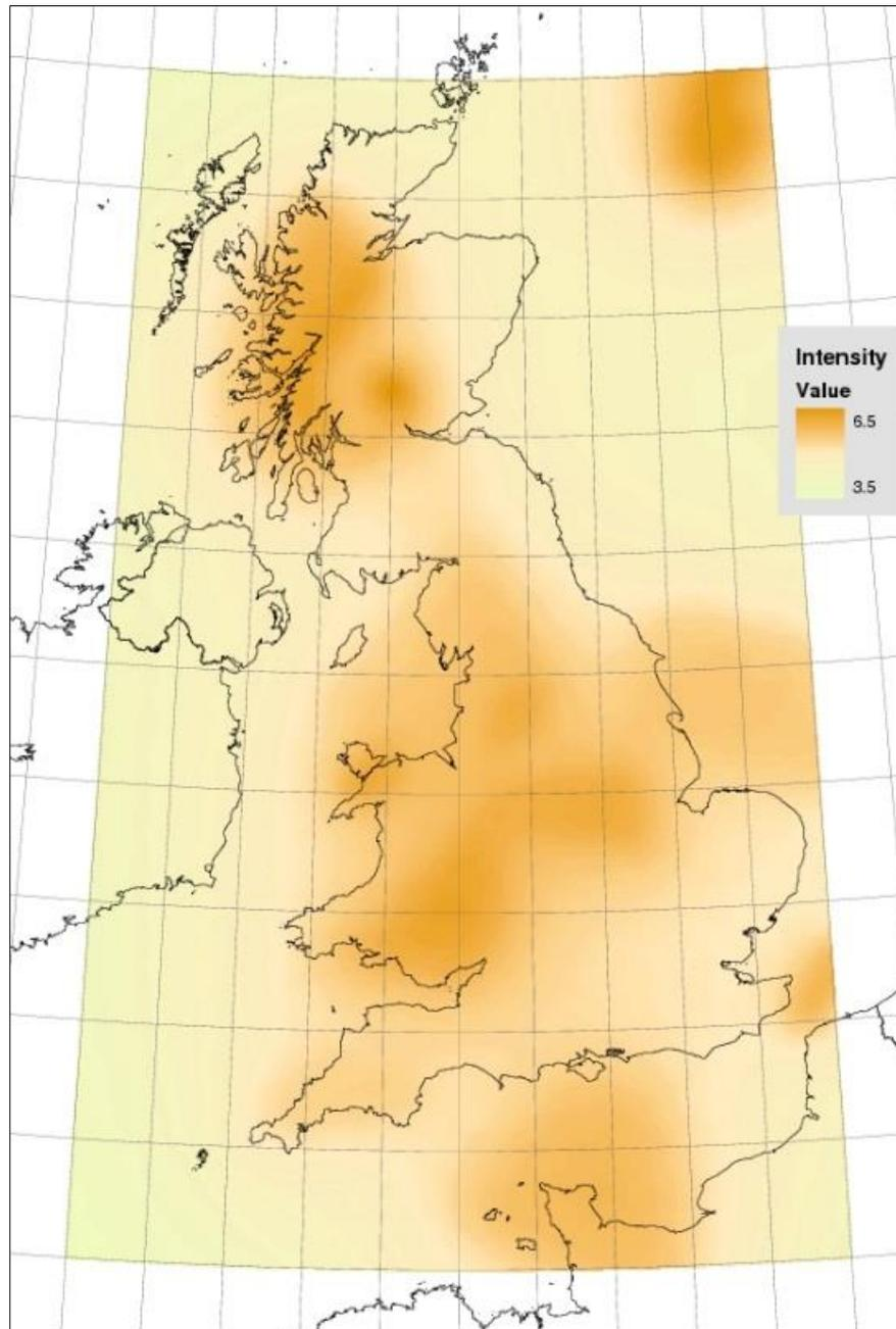
**Figure 37 – The expected intensity (EMS) of earthquake shaking with a 10% probability of being exceeded over 50-year period in the UK. (Source: Musson and Winter (1996))**
