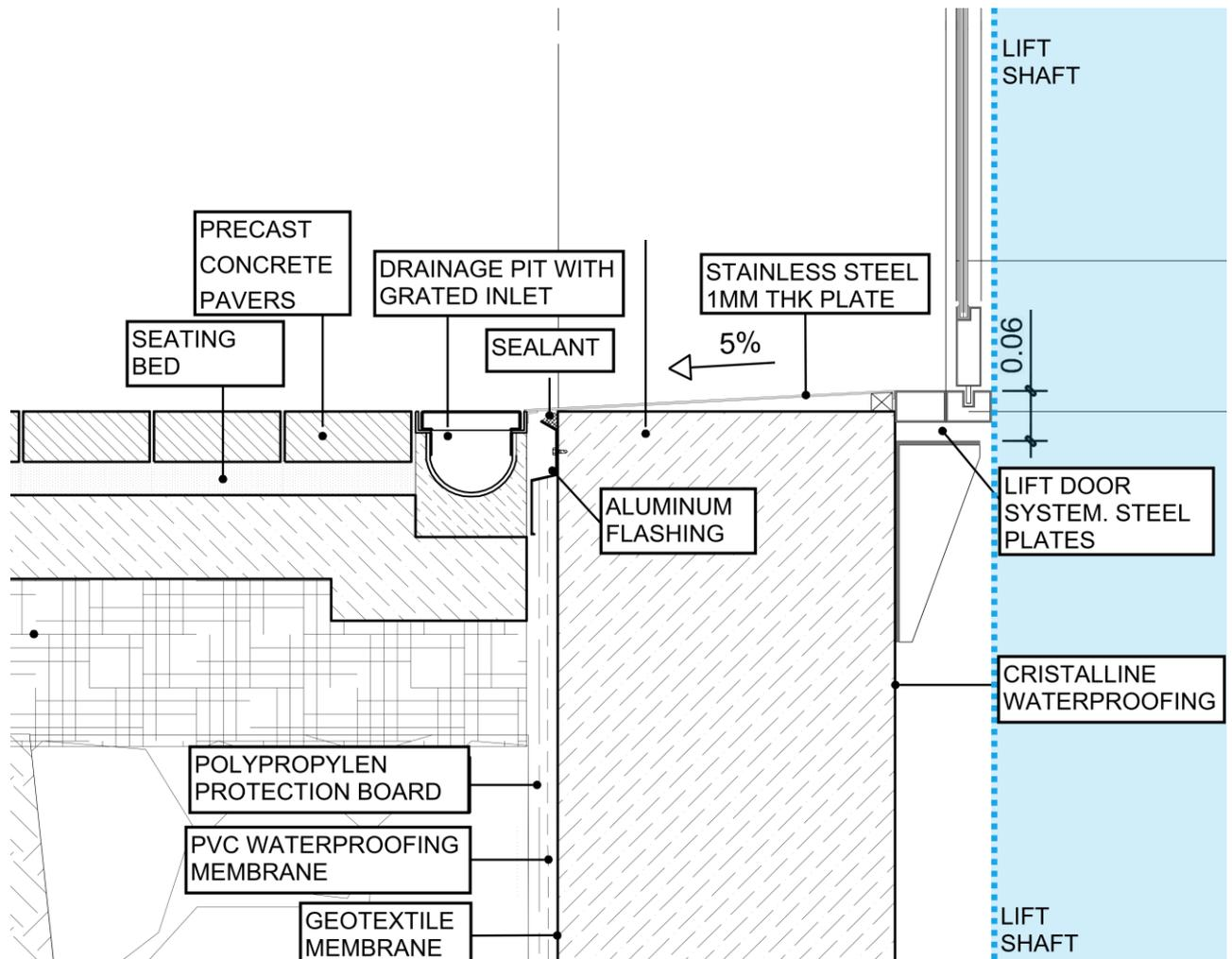
Figure 36. Waterproofing lift detail example that will be adapted to the details of the project
