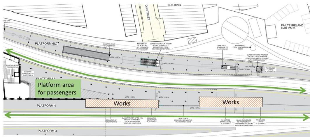
Figure 43 - Works and platform operation coexist
