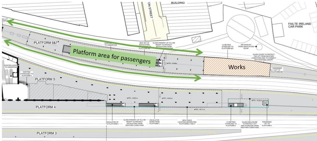
Figure 41 - Phase one: works on stairs and lift
