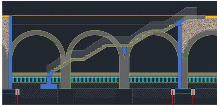
Figure 46. Sketch showing the structural solution for a void containing a staircase
