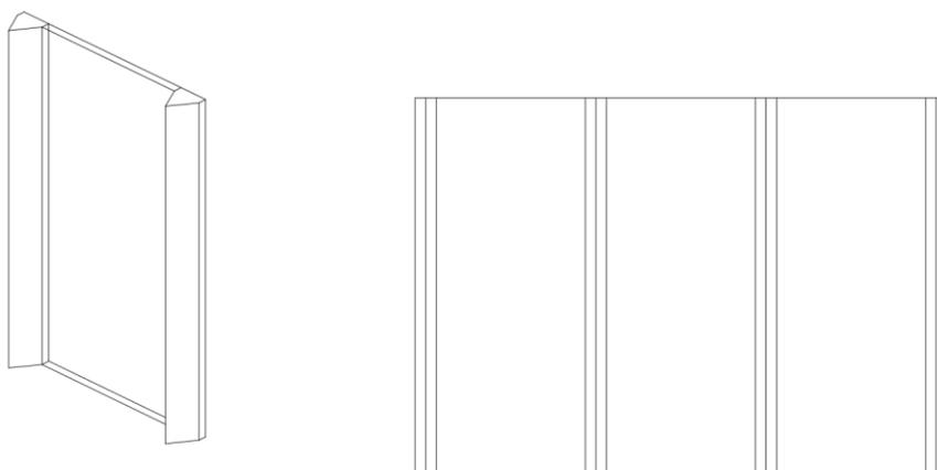
Figure 53. Axonometric and elevation view of vertical lamellas
