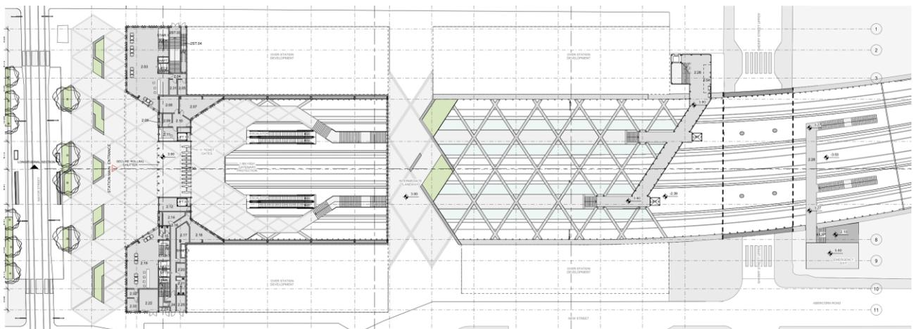
**Figure 37. Functional layout of the proposed station at street level**
