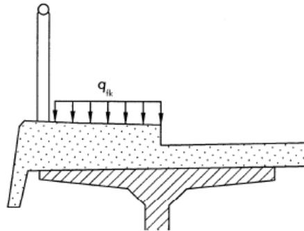
Figure 83. Characteristic load on a footway (or cycle track). Source: IS EN 1991-2
