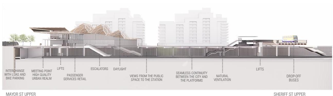
Figure 27. Graphic illustrating the section and the primary elements of the proposed station
