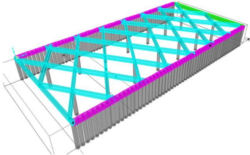
**Figure 91. Structural numerical model of shoring system over Zone D**
