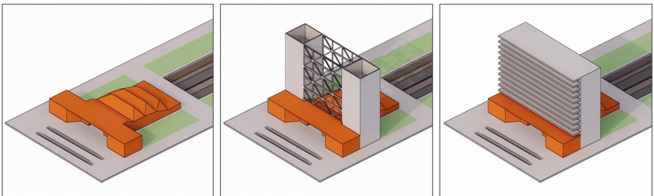
**Figure 24. Schematic representation of the landmark building structure that will be needed to bridge the station entrance**
