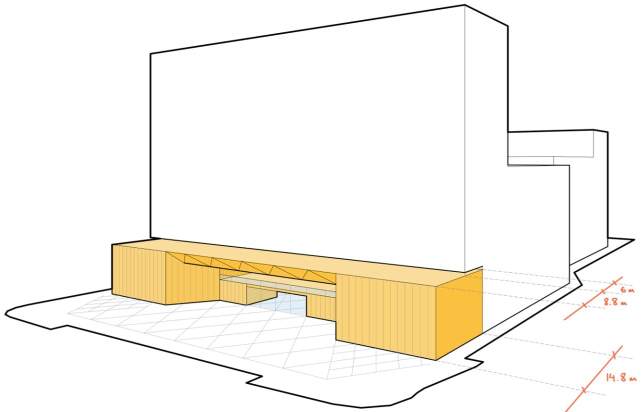
Figure 23. Dimensions of the alignment of the station with the alignment of the future landmark building.
