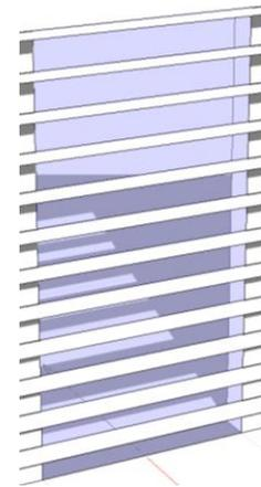
Possible shading device: Horizontal blades
