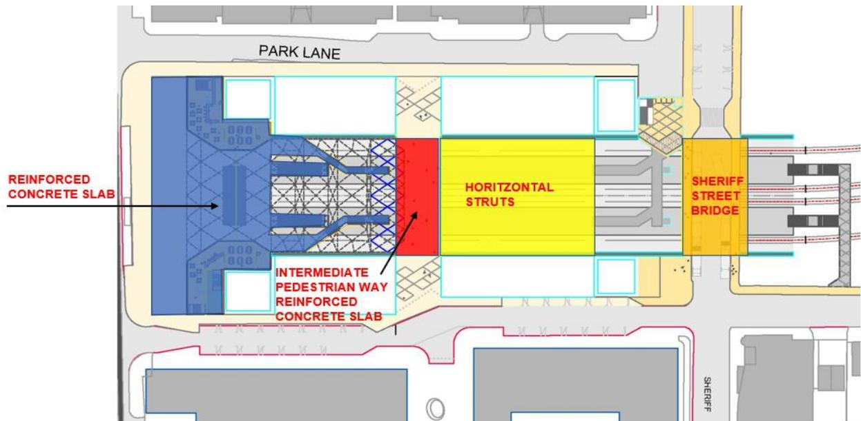
**Figure 70. Ground Level slabs typologies**
