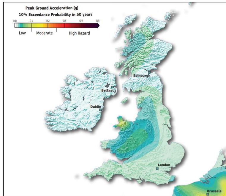
Figure 76. Peak ground acceleration [g] 10% exceedance probability in 50 years. (Source: SHARE European Seismic Hazard Map for Peak Ground Acceleration, 10% Exceedance in 50 years)
