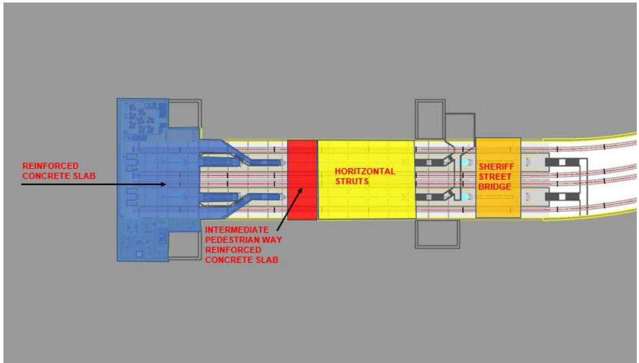
**Figure 73. Platform Level. Slabs typologies**
