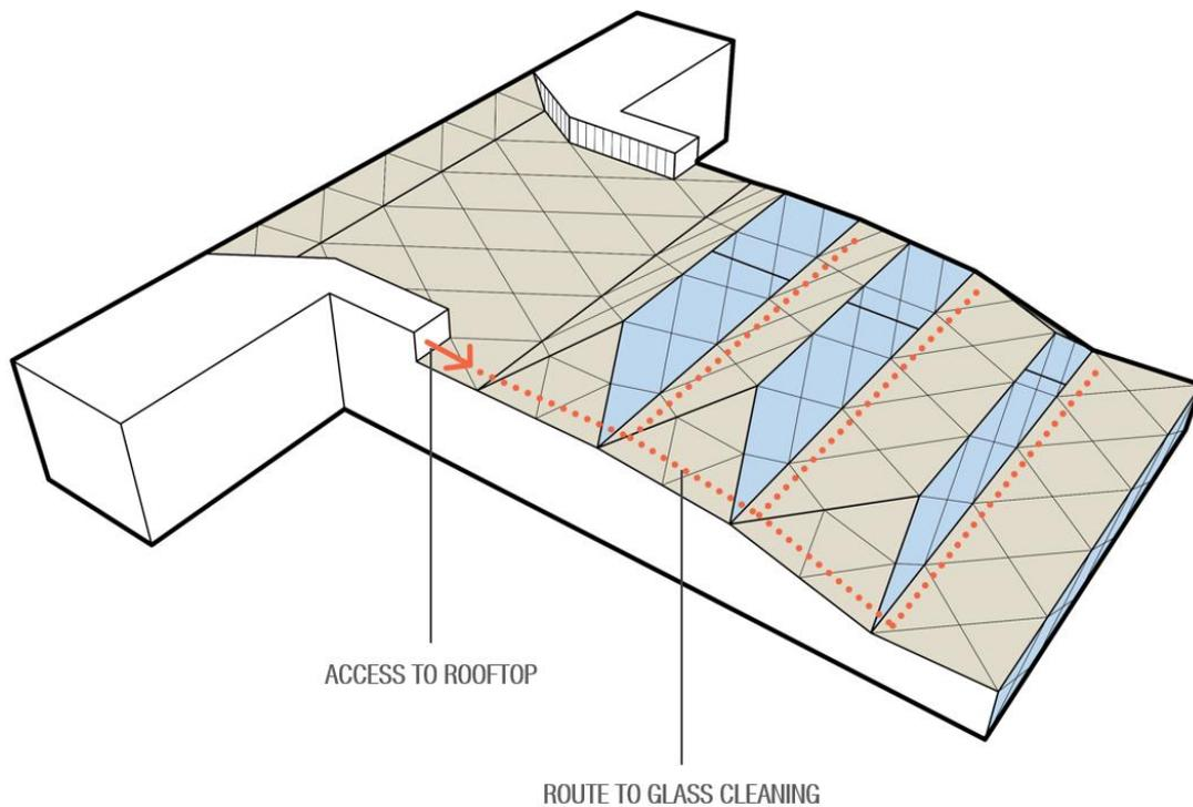
**Figure 44. Diagram of the roof maintenance routes**
