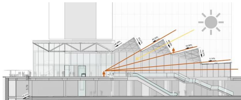
**Figure 41. Diagram showing the gables adaptation to the passengers' views.**
