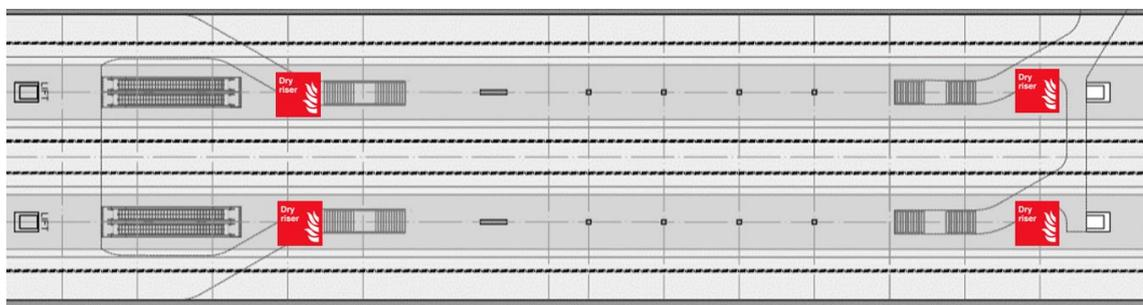
Figure 92 Dry risers on the platform.
