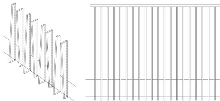
**Figure 50. Axonometric and elevation view of the balustrade design**
