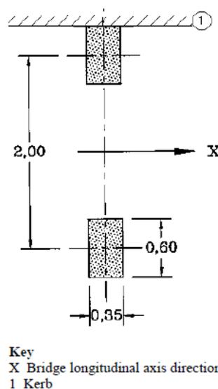
Figure 82. Application of load model 2. Source: IS EN 1991-2. LM2 is derived from I.S. EN 1991: Eurocode 1, Action on Structures
