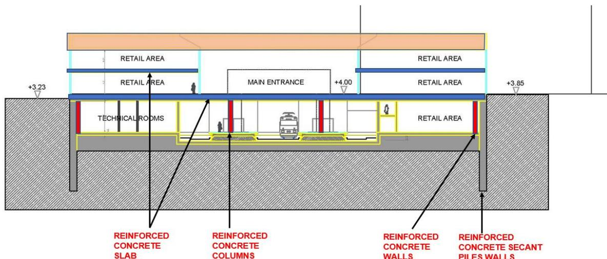
Figure 72. Cross section. Structural systems
