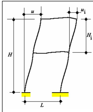
Figure 85. Definition of Horizontal displacements. Source: I.S. EN-1990-2002+A1-2005, A.1.4.3
