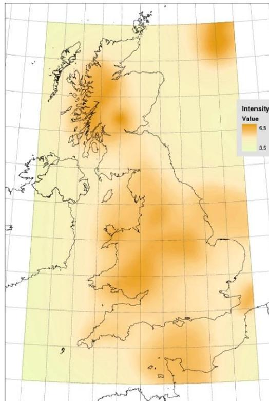
**Figure 75. The expected intensity (EMS) of earthquake shaking with a 10% probability of being exceeded over 50-year period in the UK. (Source: Musson and Winter (1996))**
