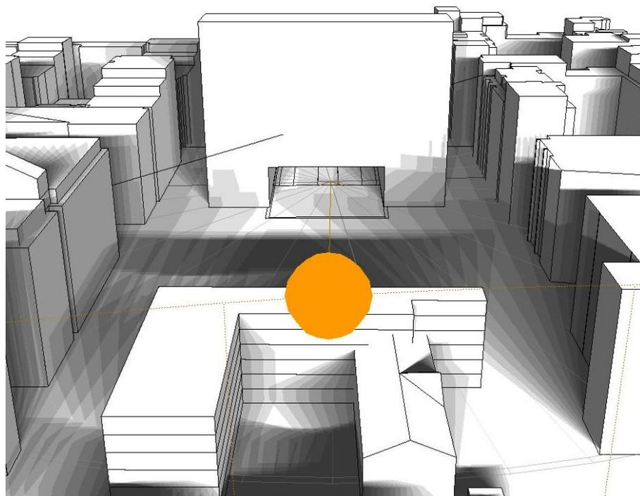
**Figure 102. Front view of the proposal for the 21<sup>st</sup> of December, on the winter solstice, when the sun has its lower height of the year.**
