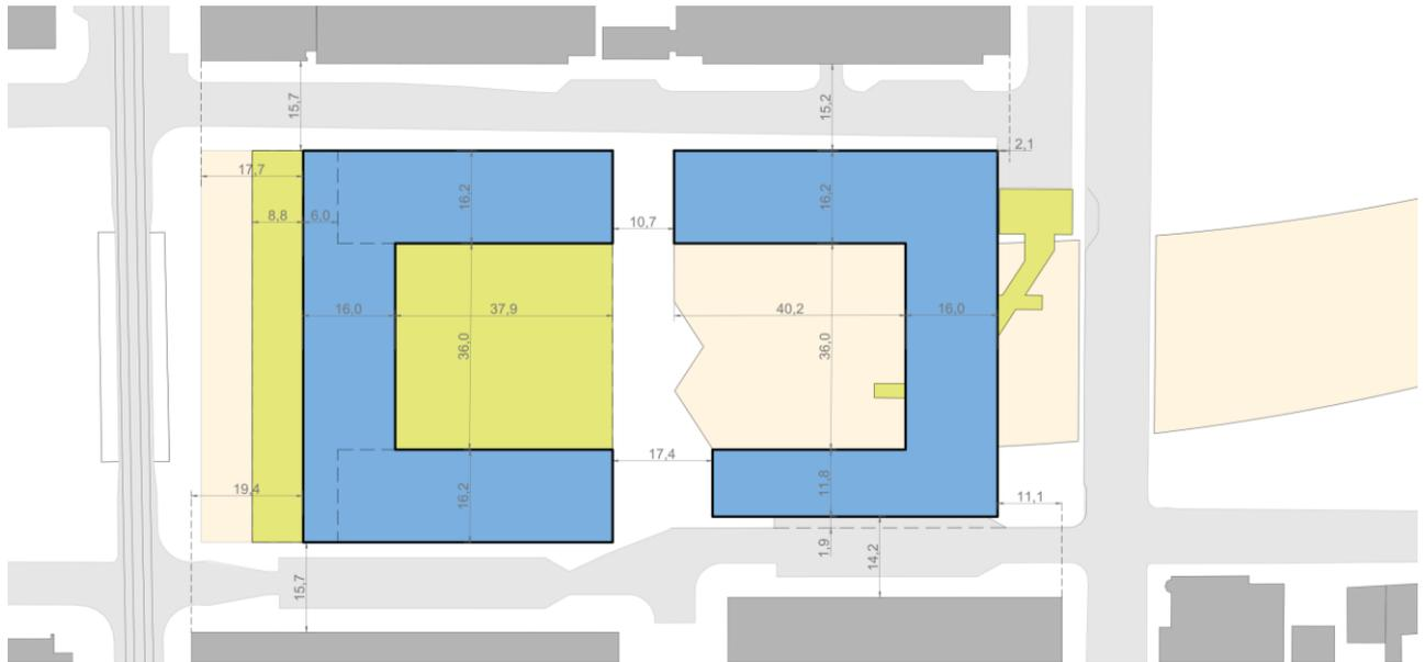
Figure 22. Dimensions and alignments of a possible configuration of the OSD (blue) integrated with the station design (green).
