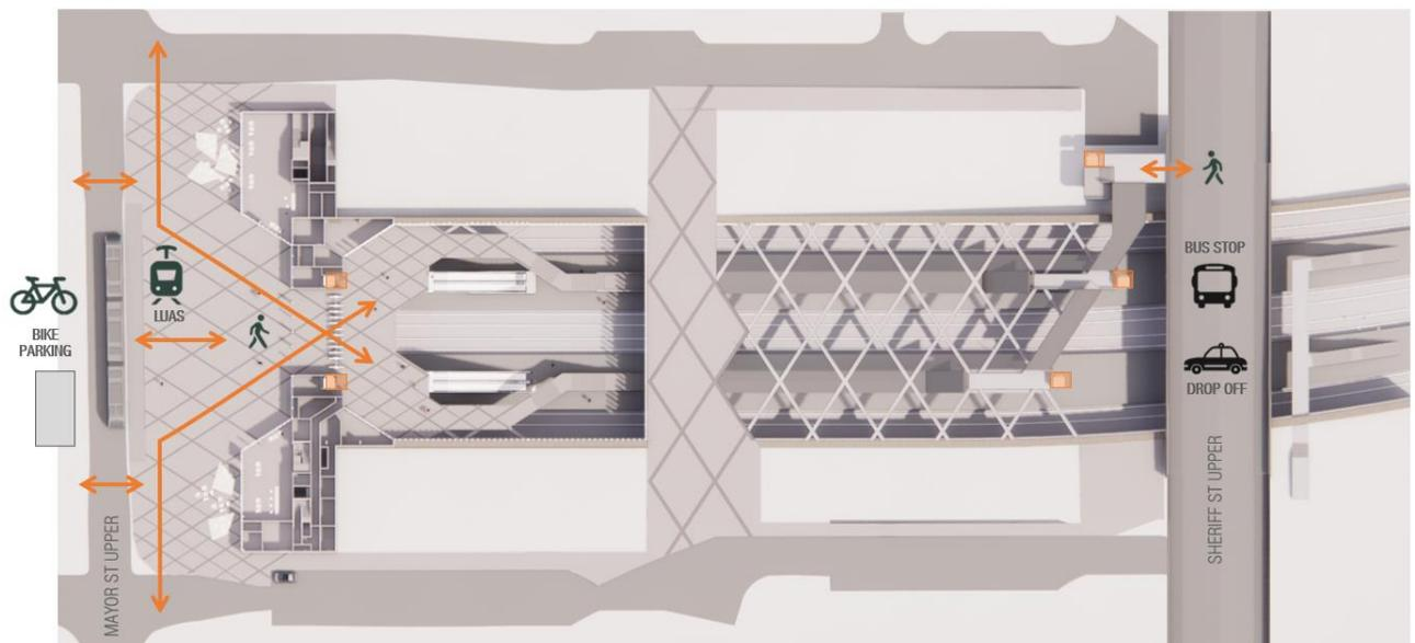
Figure 26. Diagram showing the intermodality and accesses to Spencer Dock Station
