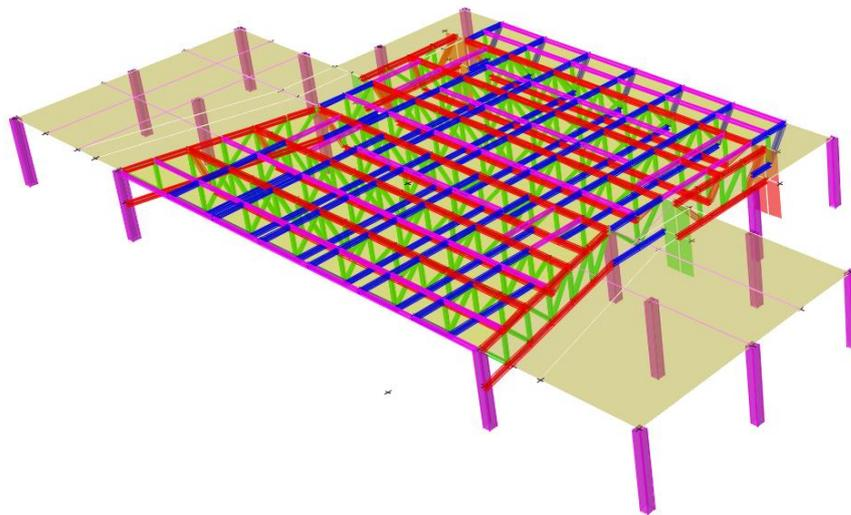
**Figure 88. Structural numerical model of roof steel structure over Zone A**
