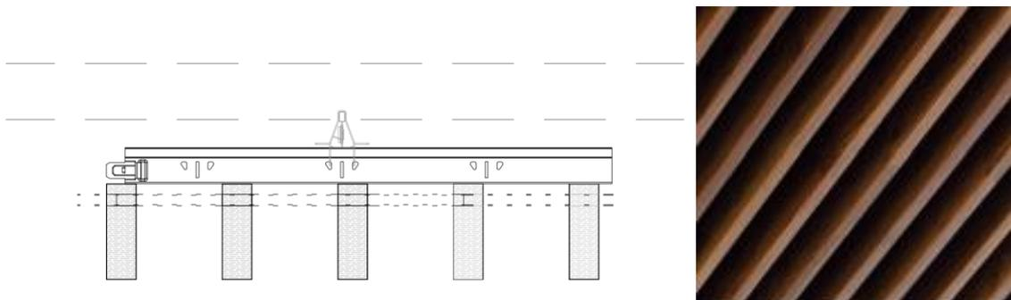
**Figure 49. Section detail of timber ceiling. Photo of timber ceiling**
