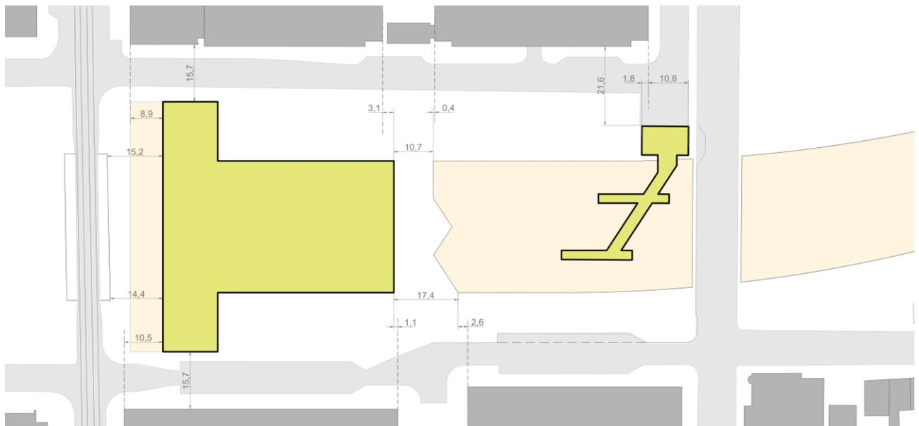
Figure 21. Spencer Dock Station alignments. Above ground station footprint
