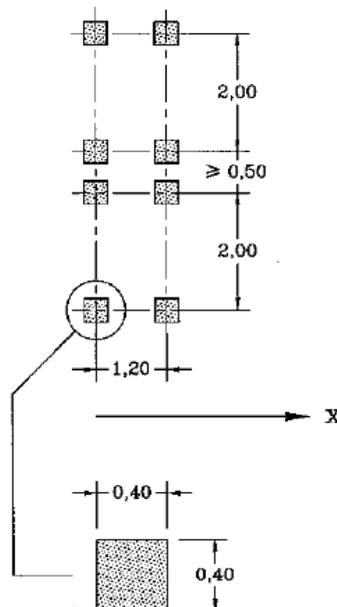
**Figure 80. Application of tandem systems for local verifications. Source: IS EN 1991-2**
