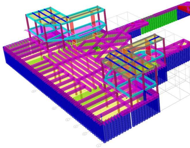
**Figure 87. Structural numerical model of reinforced concrete structure of Zone A and B**
