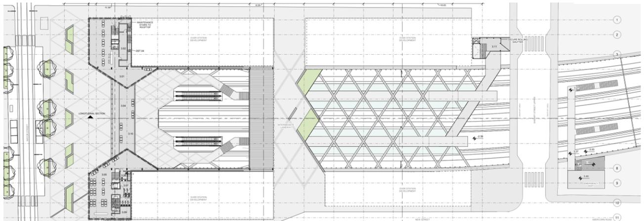
Figure 38. Functional layout of the proposed station at first floor level
