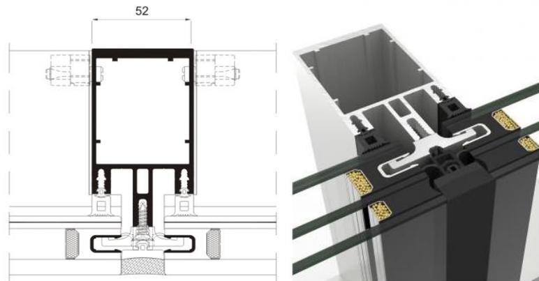
Figure 62. Section and photo detail of curtain wall.
