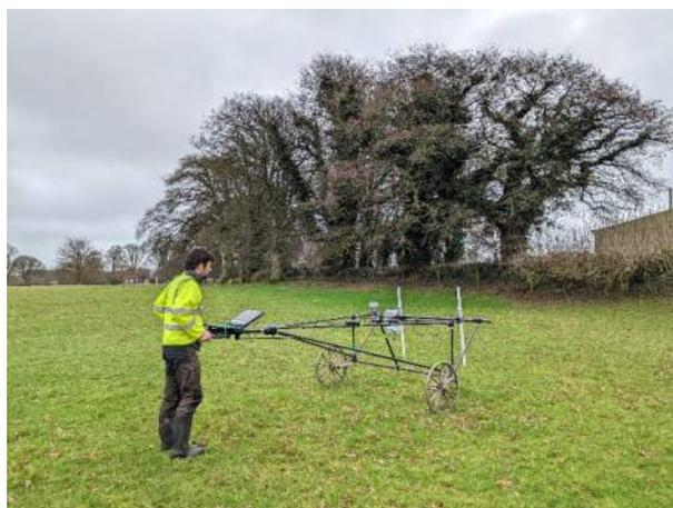
Bartington Grad 601-single axis dual sensor gradiometer.
