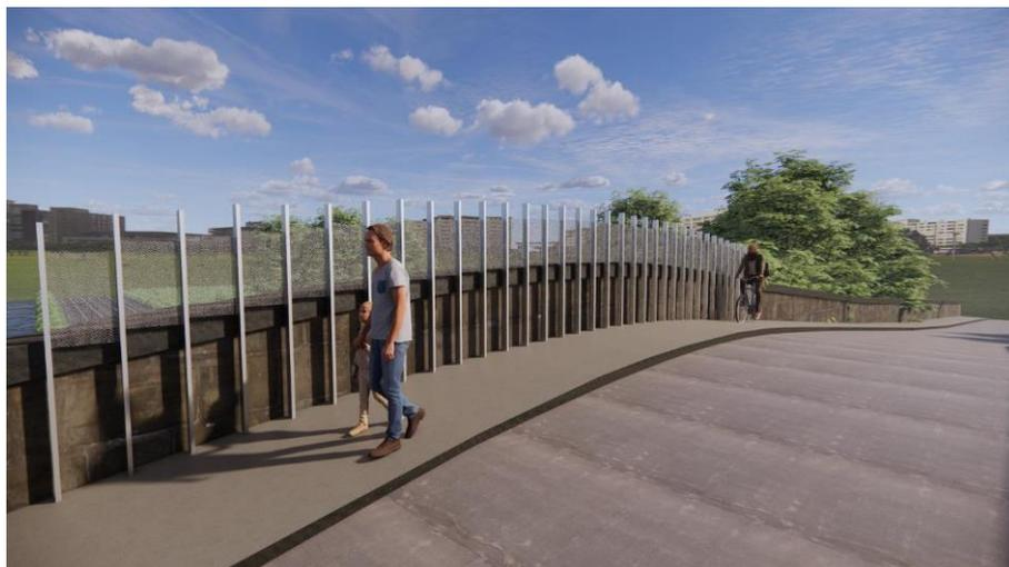
**Figure 29** – Render of design proposal to increase the parapet height to 1800mm with mesh about 1200mm.
