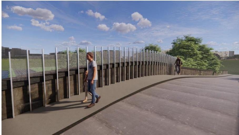
**Figure 29** – Render of design proposal to increase the parapet height to 1800mm with mesh about 1200mm.
