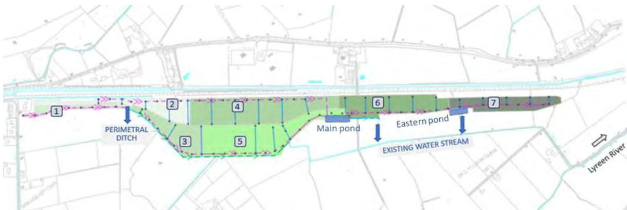
**Figure 4-252 Surface drainage sub catchments**
