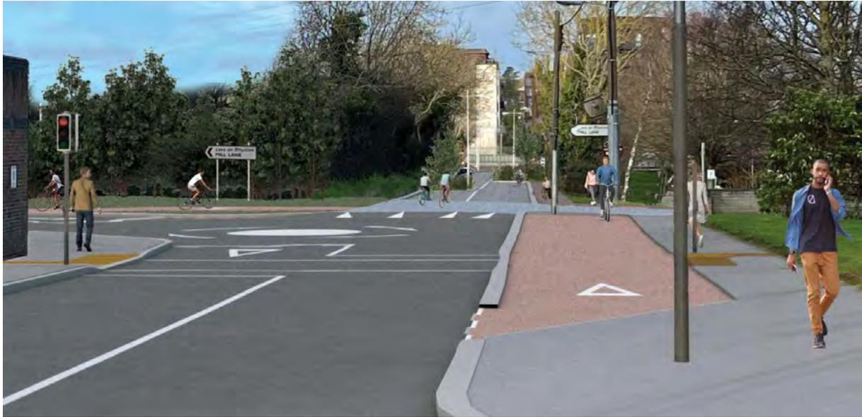
**Figure 4-142 Detail of cycletrack/footway segregation – Ashtown level crossing**
