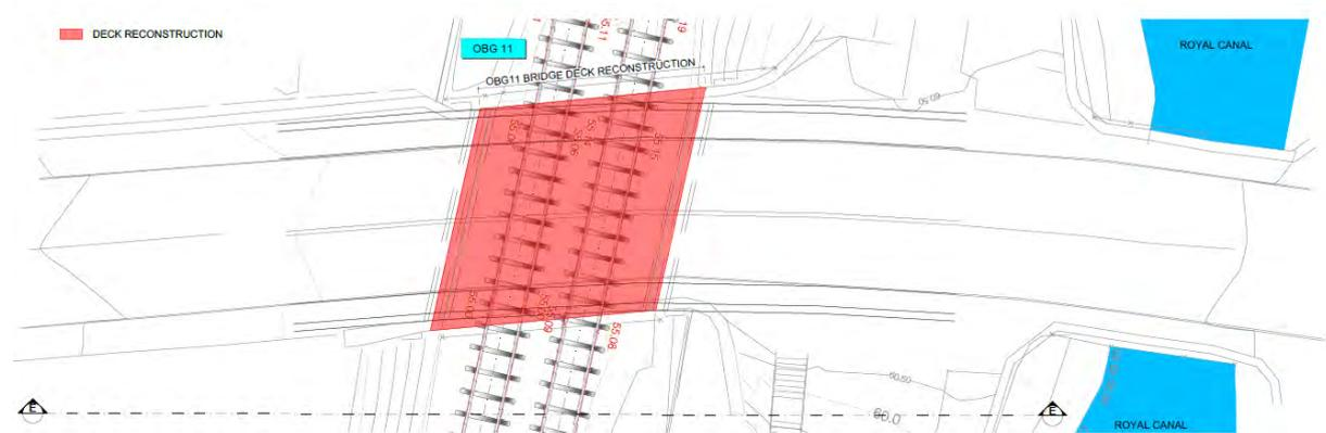
Figure 4-158 Deck reconstruction of OBG11 - Plan view
