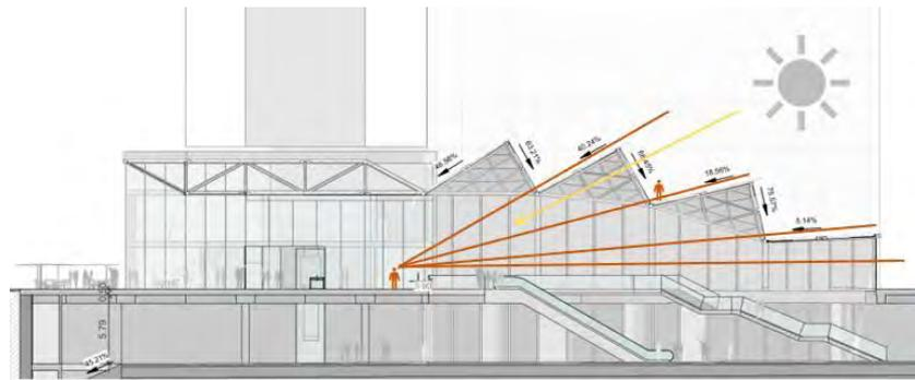
**Figure 4-105 Adaption of gable inclination to passenger sightlines**
