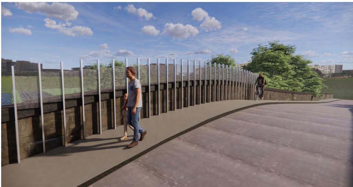
**Figure 4-45 Design intent for parapet heightening on bridges - 3D image**
