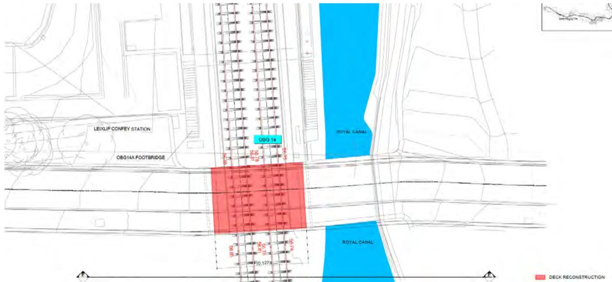
**Figure 4-196 Deck reconstruction of OBG14 - Plan view**
