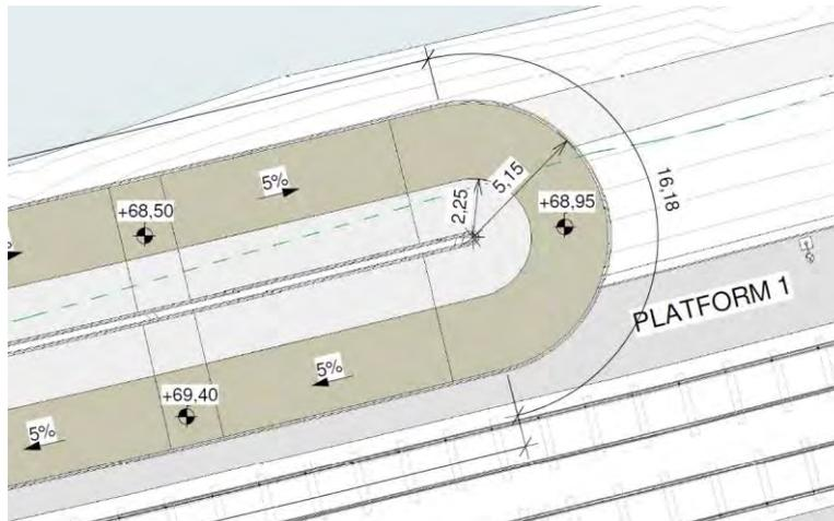
**Figure 4-170 Details of radii on Coolmine bridge/ramp**
