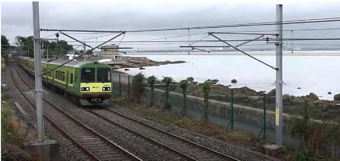
**Figure 4-23 Current DART cantilever layout**
