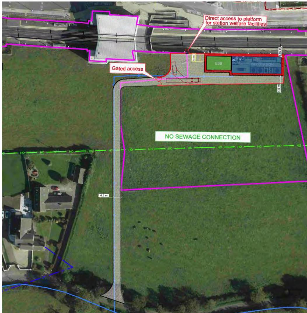
**Figure 4-185 Location details and utilities in Hansfield Substation**
