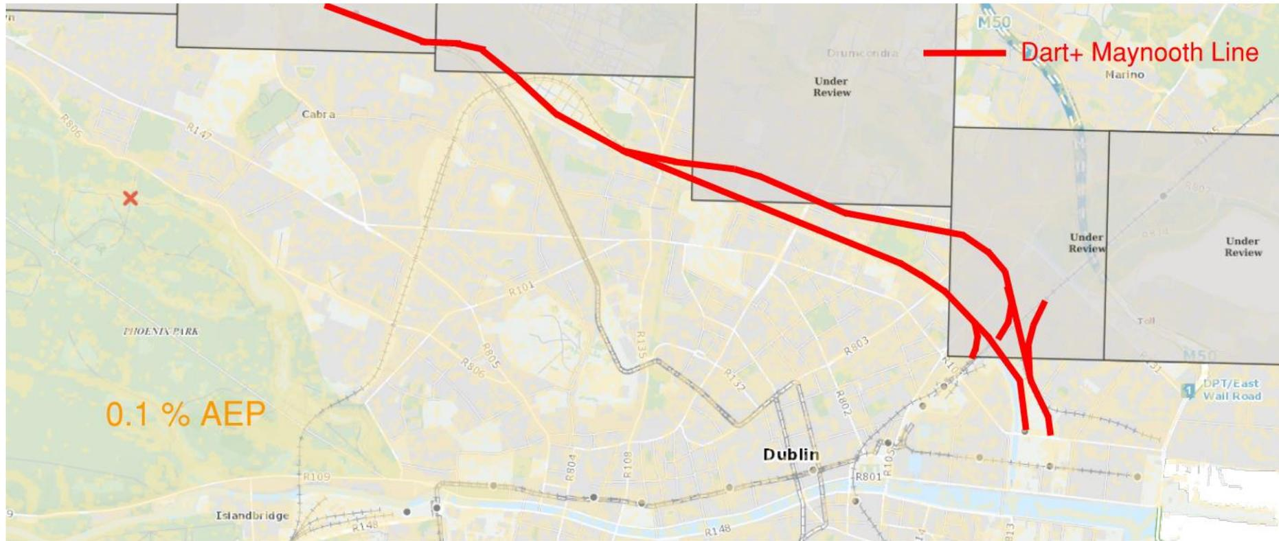
CFRAMS Pluvial Flood Mapping. ROD annotations in red indicating development corridor.
