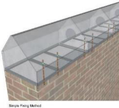
Figure 4-32 GRP Parapet Extension
