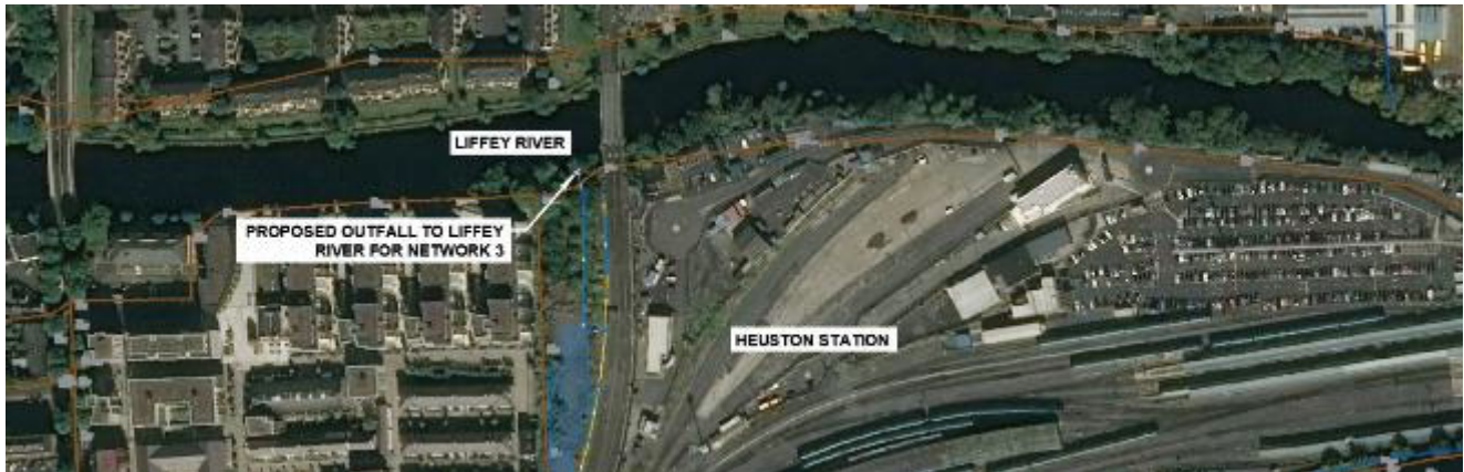
Figure 4-92 Proposed Outfall for Network 3
