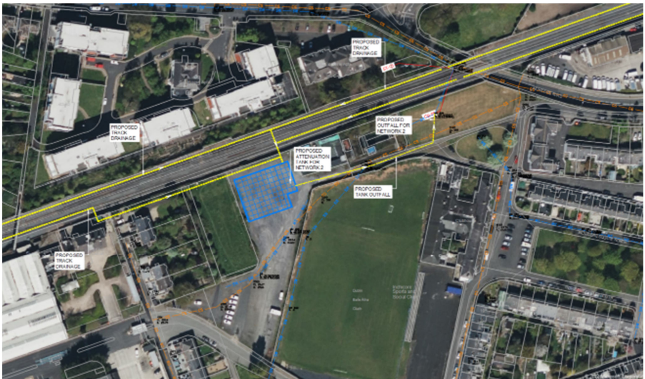
Figure 4-88 Proposed Outfall for Network 2
