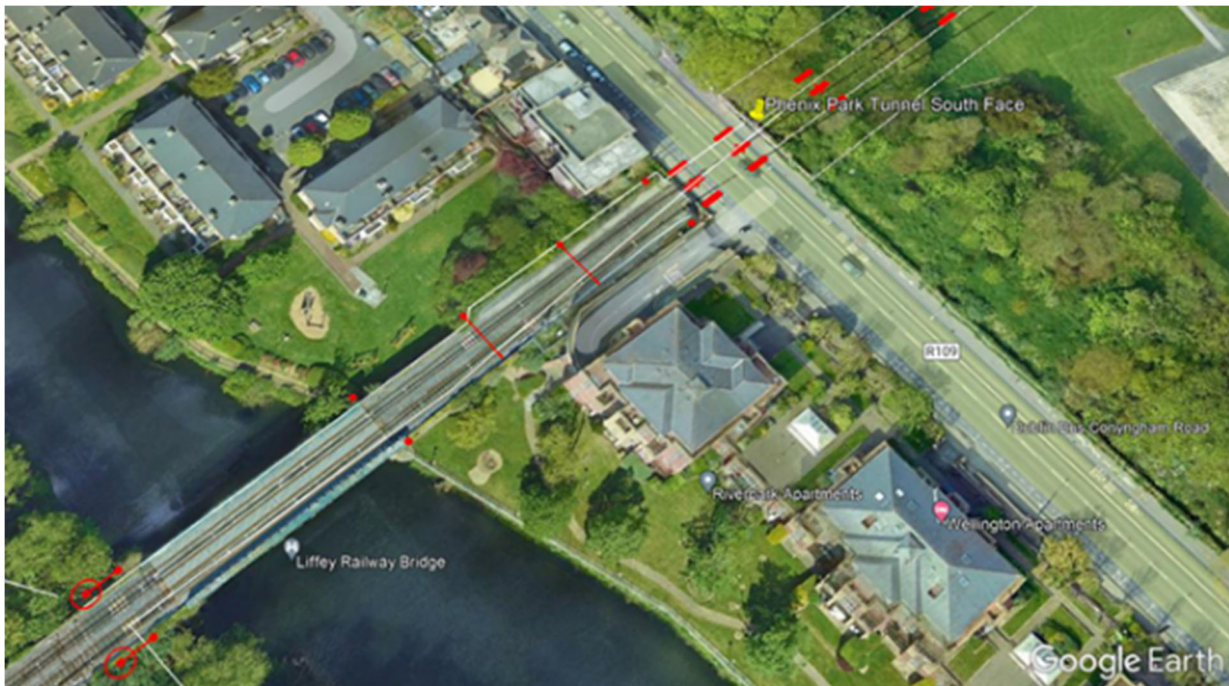
Figure 4-144 OHLE Mast Position for Liffey Bridge (UBO1) and Conyngham Road Bridge (OBO2)
