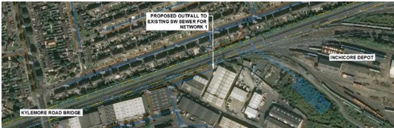
Figure 4-84 Proposed Outfall for Network 1
