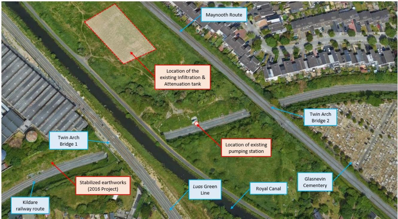
Figure 6-5 Location of the Twin Arch Bridges (OBO8 & OBO9) and existing drainage systems in the vicinity of Royal Canal.
