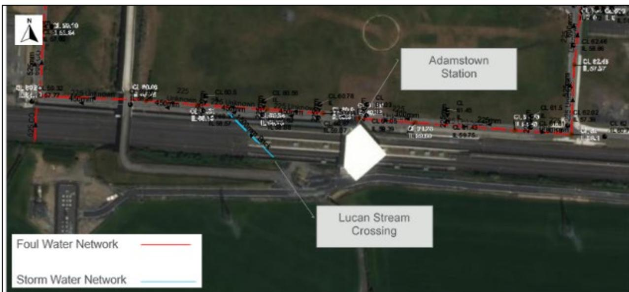
Figure 3-22 IW GIS Database – Storm and Foul Network in the vicinity of Lucan Stream Crossing the Railway
