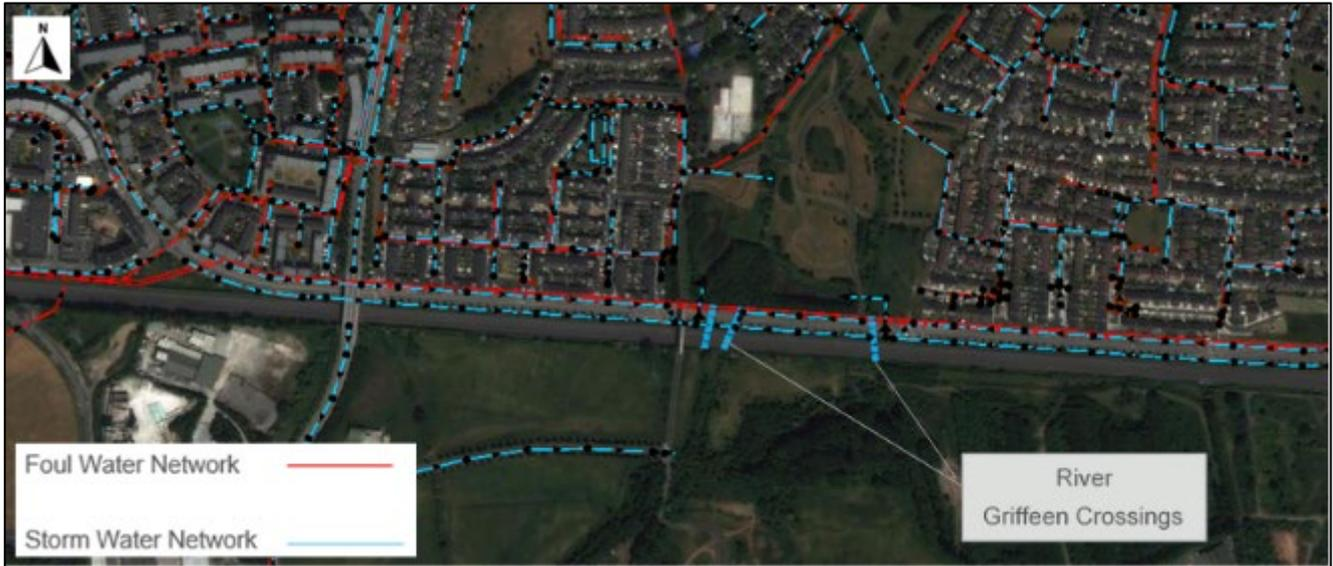
Figure 3-23 IW GIS Database – Storm and Foul Network in the vicinity of River Griffeen Crossing the Railway
