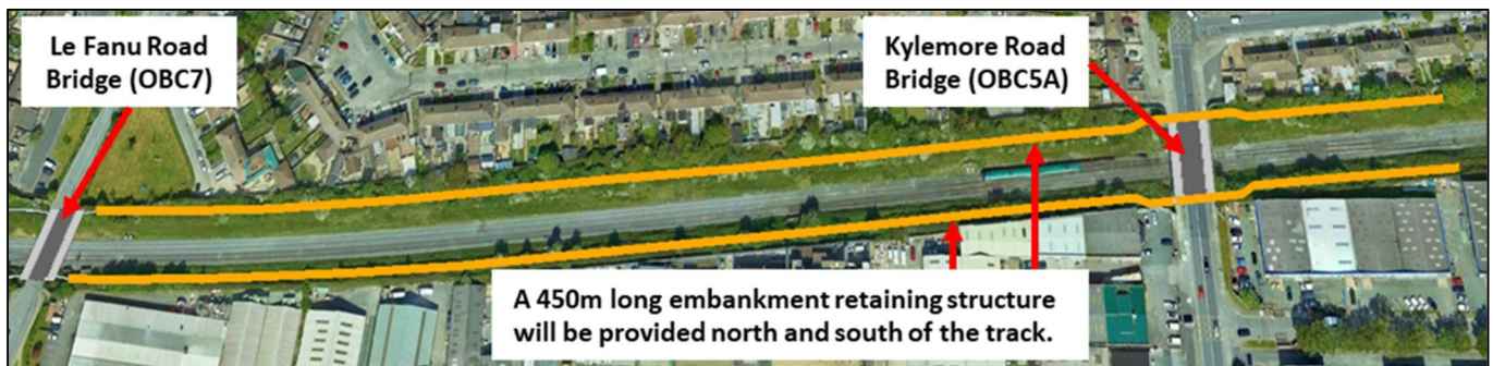
Figure 5-4 Proposed Retaining Wall Locations
