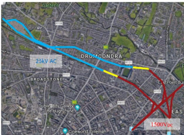
Figure 20. Phase 1: Install 25kV AC on new lines AC - Neutral Zone for Hazelhatch and Maynooth Lines
