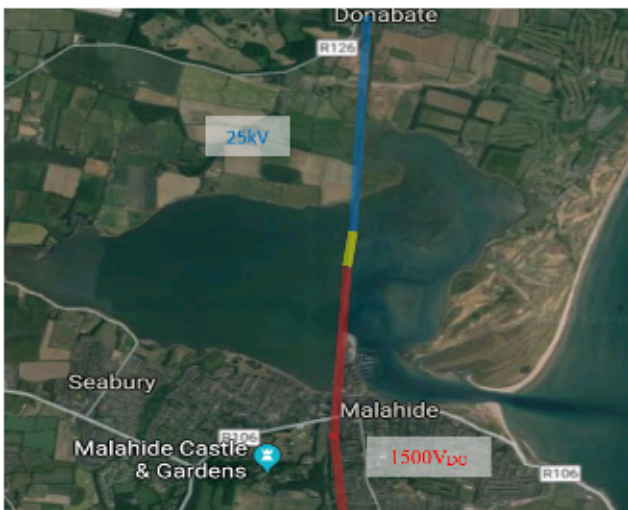
Figure 21. Phase 1: Install 25kV AC on new lines AC - Neutral Zone for Malahide to Drogheda Lines
