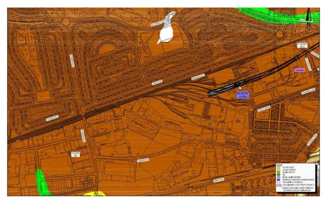
Figure 26: Quaternary Geology Map - Kylemore Road - Inchicore with alignment of original DART Underground overlaid
