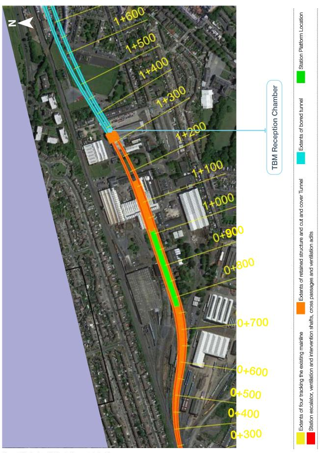
Figure 72: Option 1F Portal Layout at Inchicore
