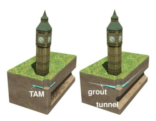
Figure 41: Example of Compensation Grouting and the use of TAMs to control ground movements
