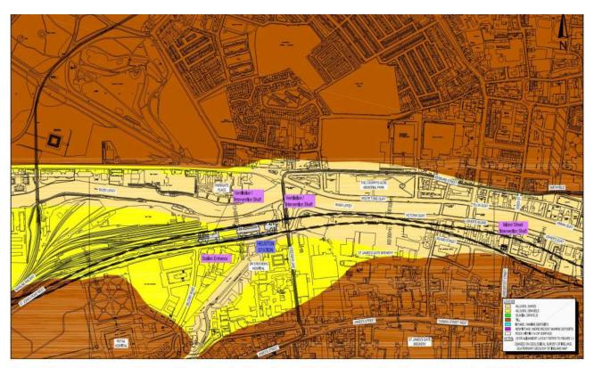
Figure 28: Quaternary Geology Map - Islandbridge - East of Watling Street with alignment of original DART Underground overlaid
