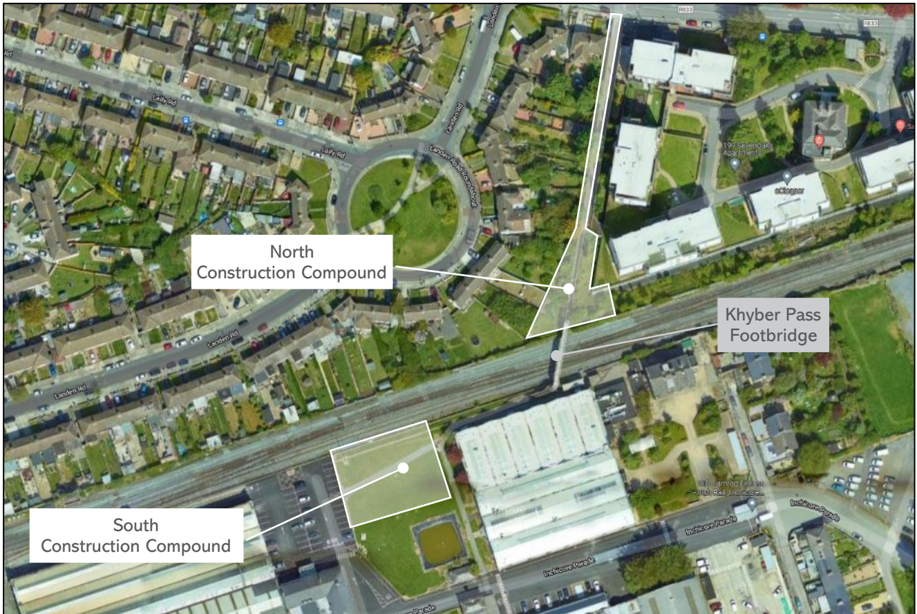
Figure 7-23 Khyber Pass Footbridge Preferred Construction Compound Locations
