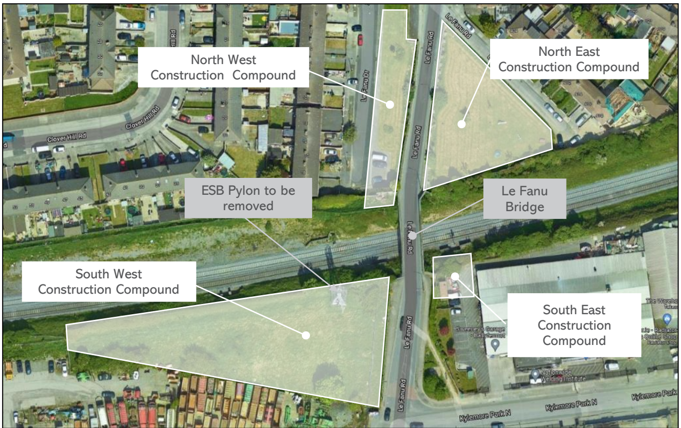
Figure 7-8 Le Fanu Bridge - Preferred Construction Compound Location
