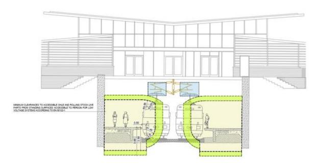
Figure 7-15 Example OHLE system in station area with clearance
