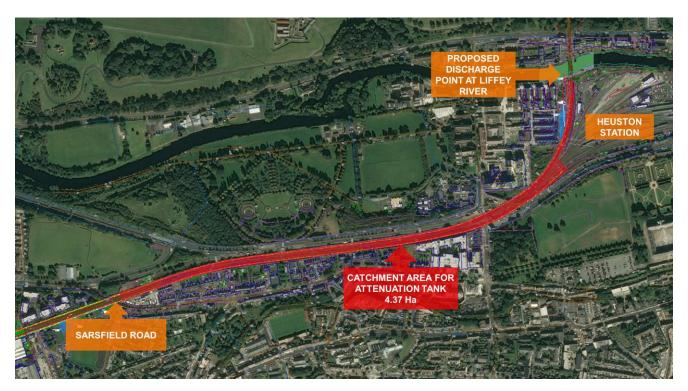
Figure 4-5:- Catchment area for the proposed attenuation tank
