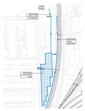
Figure 7-16 Proposed Track Drainage Layout at Heuston West
