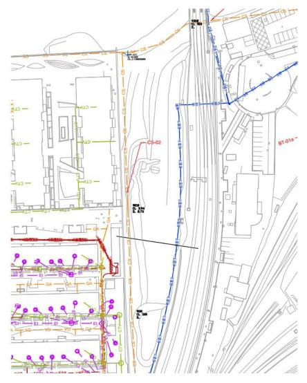
Figure 4-1 Utilities beneath Proposed Heuston West Station
