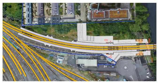
Figure 5-7 Station Option C – underpass with stairs and lifts
