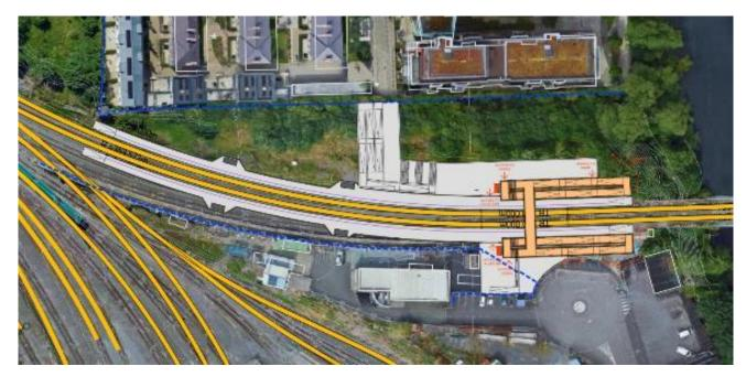
Figure 5-3 Station Option B – footbridge with ramp and stairs
