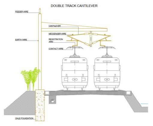
Figure 7-14 Typical OHLE arrangement in two track open route – Facing East.
