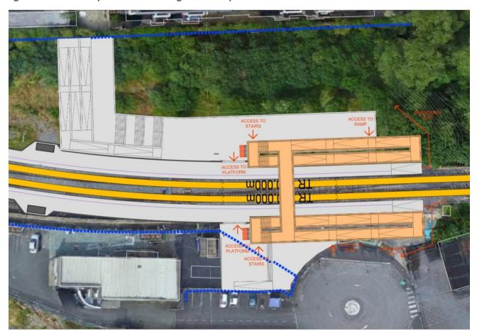
Figure 5-4 Station Option B. Access details
