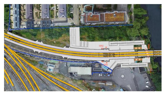
Figure 5-11 Station Option E – underpass with ramp and stairs
