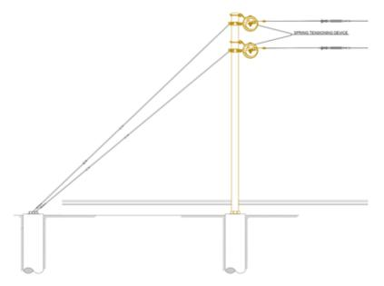
Figure 3-2 Typical anchor structure
