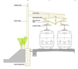
Figure 3-1 Typical OHLE Arrangements in 2-Track Section – on entry to the East of the Station
