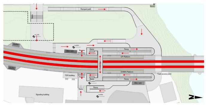
Figure 7-2 Proposed Heuston West Station Plan & Detailed Access Routes
