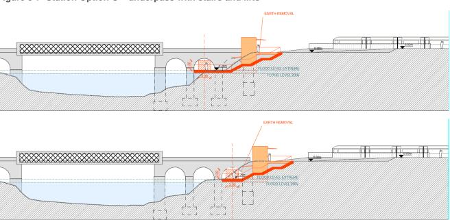
Figure 5-8 Station Option C - underpass with stairs and lifts - cross section options
