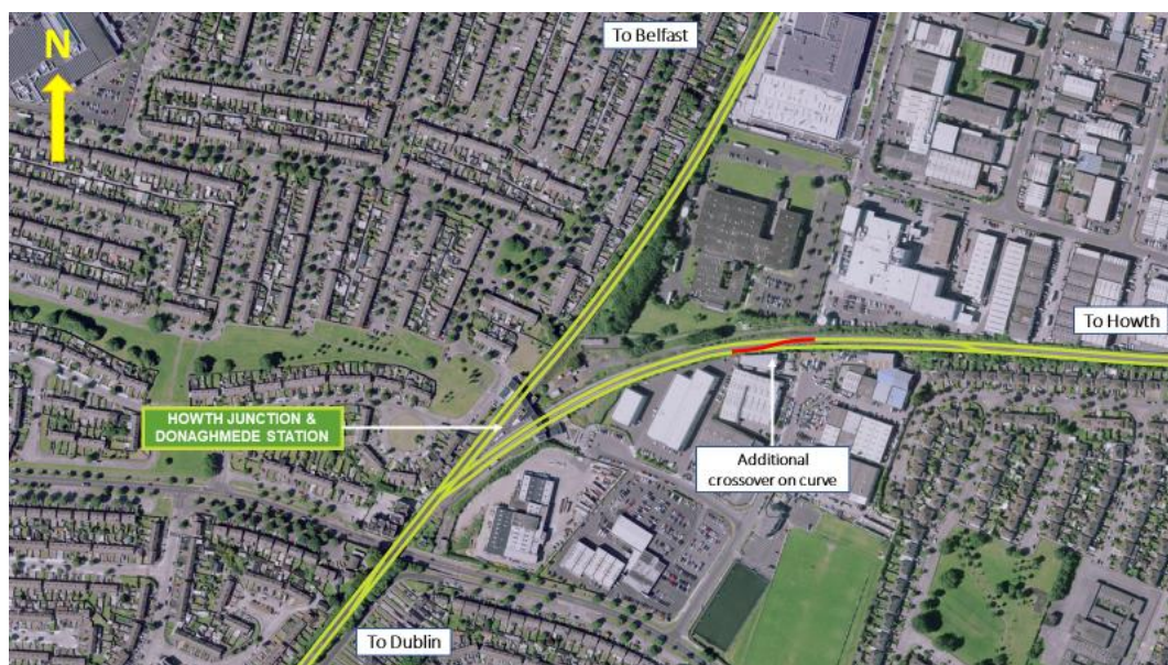
Figure 5-3: Aerial view of Option 2 (green indicates existing track and red indicates new track)
