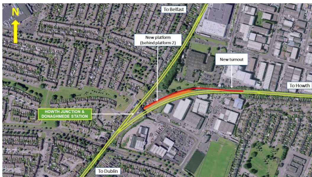
Figure 5-15: Aerial view of Option 7a (blue indicates existing track and red indicates new track)
