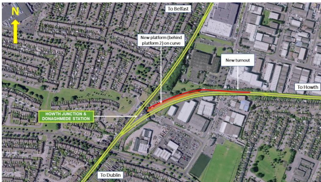
Figure 5-11: Aerial view of Option 6 (green indicates existing track and red indicates new track)
