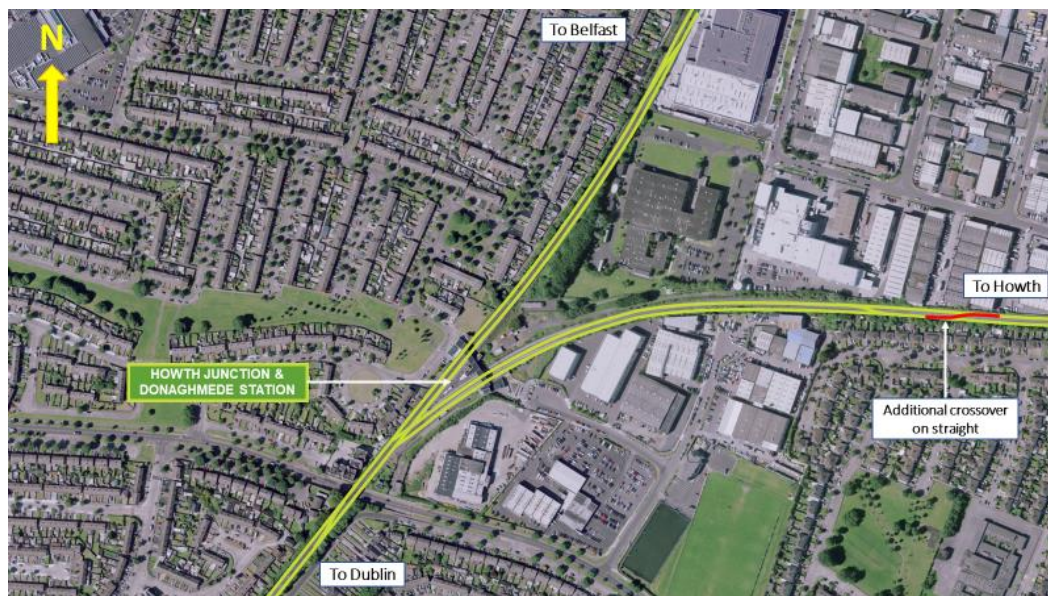
Figure 5-1: Aerial view of Option 1 (green indicates existing track and red indicates new track)
