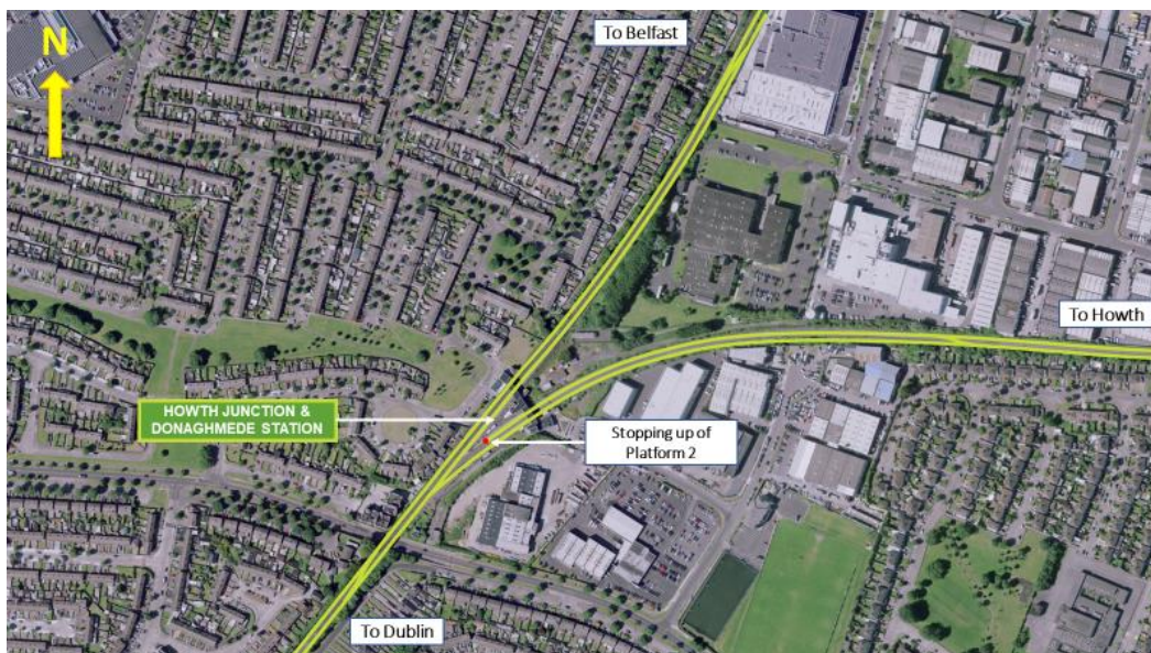
Figure 5-7: Aerial view of Option 4 (green indicates existing track and red indicates new track)
