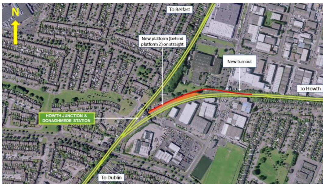
Figure 5-13: Aerial view of Option 7 (green indicates existing track and red indicates new track)
