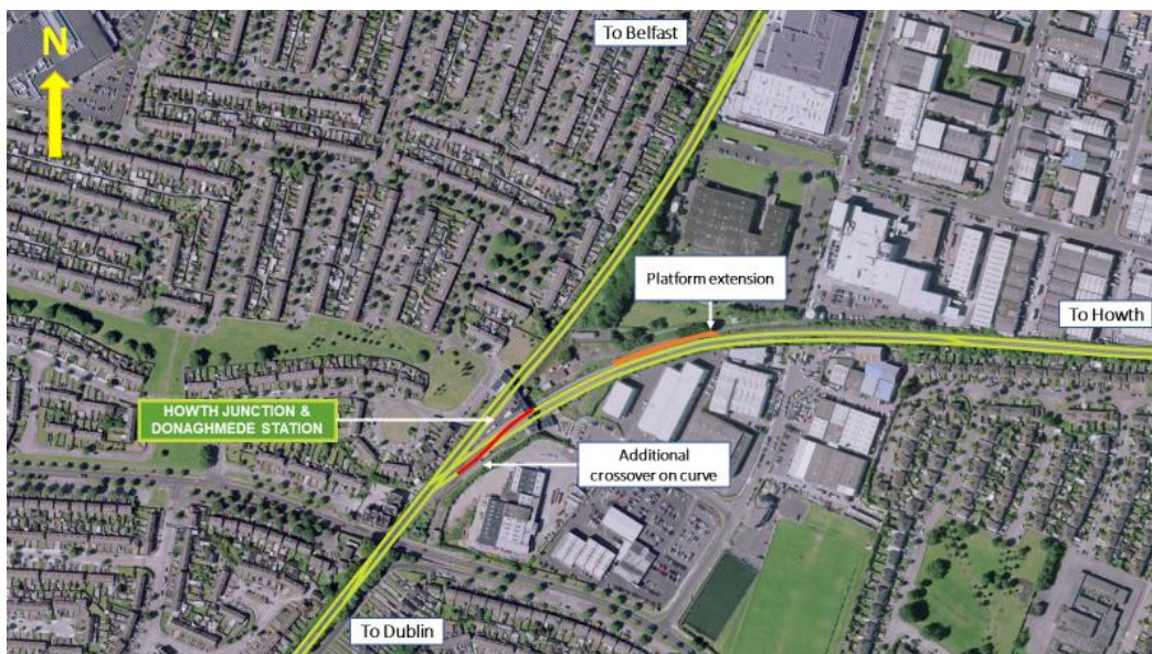
Figure 5-5: Aerial view of Option 3 (green indicates existing track and red indicates new track)
