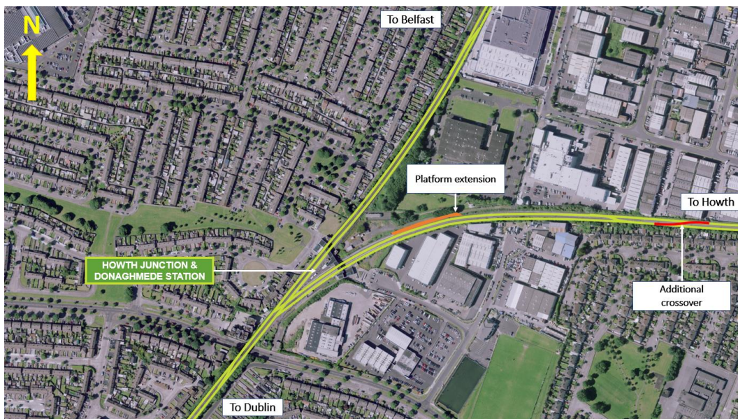
Figure 5-9: Aerial view of Option 5 (green indicates existing track and red indicates new track)
