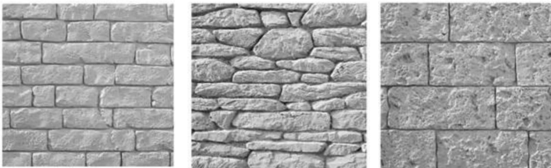
Figure 7-3 Examples of Architectural Concrete Finishes and/or Limestone Cladding
