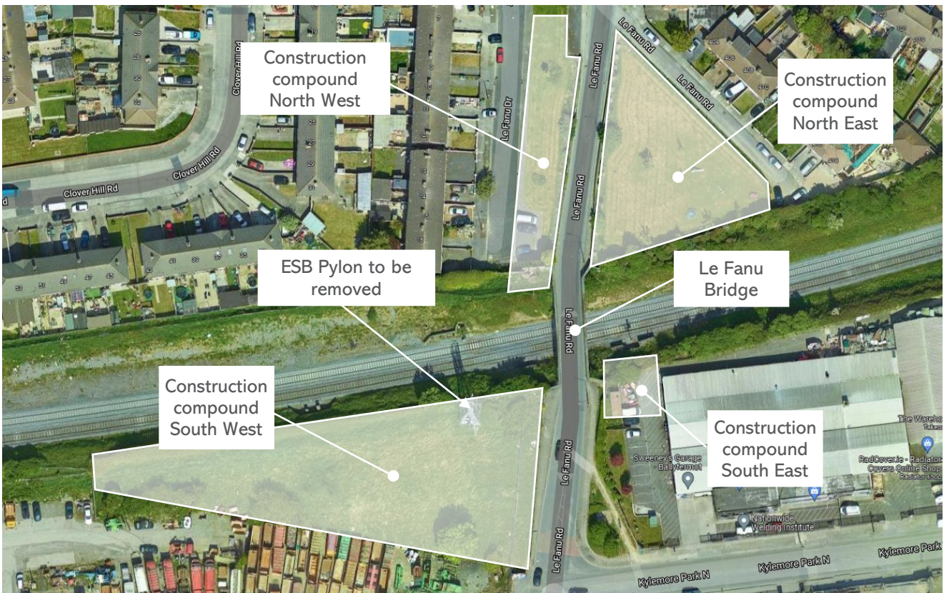
Figure 5-11 Le Fanu Bridge Construction Compounds
