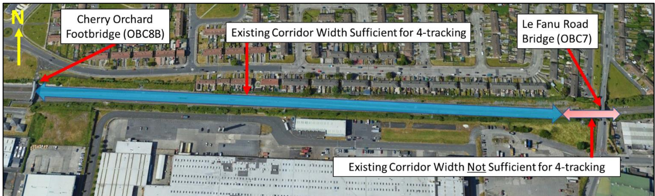
Figure 4-2 Rail Corridor Width
