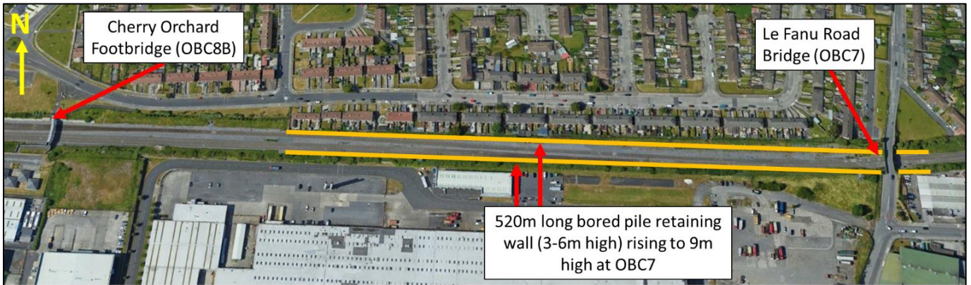
Figure 5-5 Indicative extent of retaining walls required within IE property
