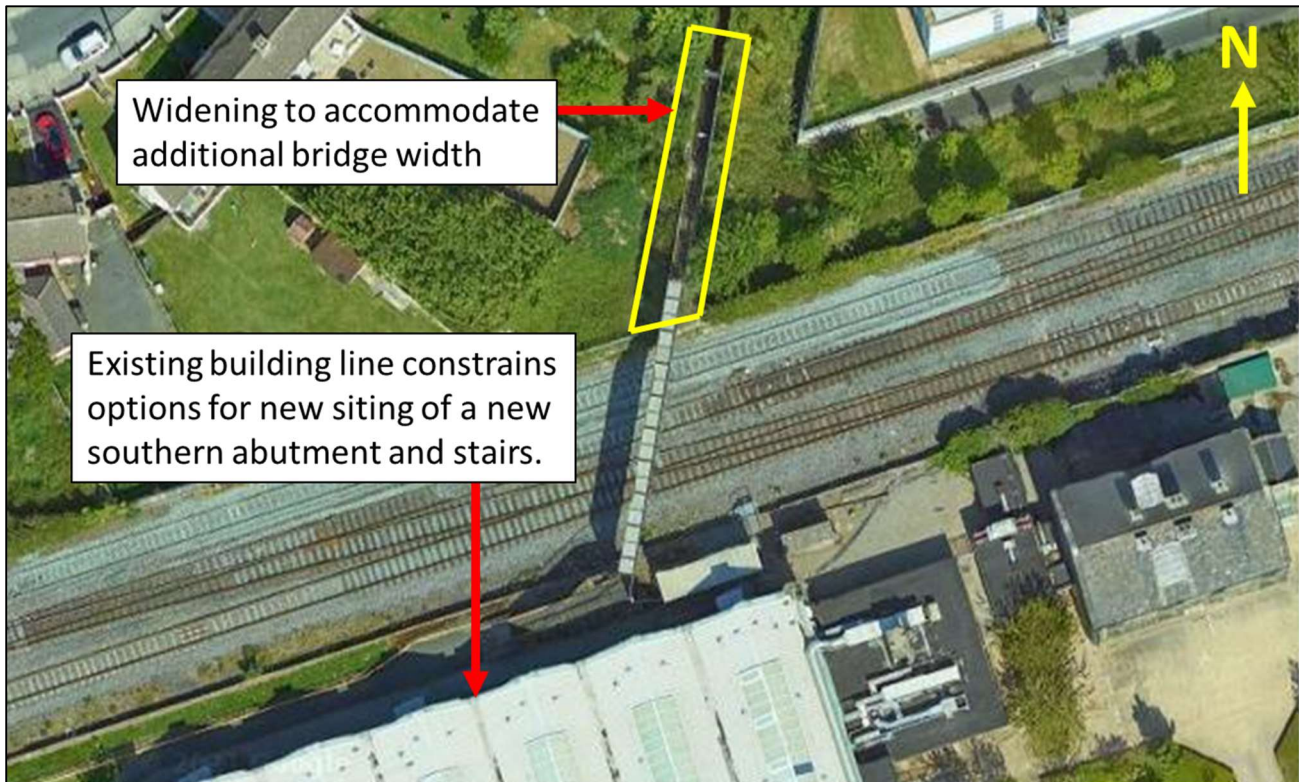
Figure 4-1 Existing pathway not sufficiently wide to provide ambulant disabled access
