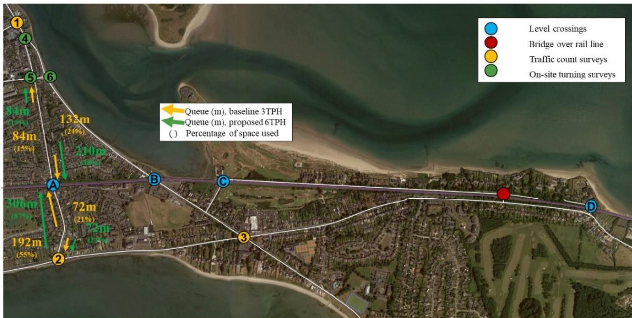
Figure 4-8 Comparison – Kilbarrack (917) Level Crossing and Dublin Road/Baldoyle Road Junction SB Arm Queue Length Modelling Results – PM Peak
