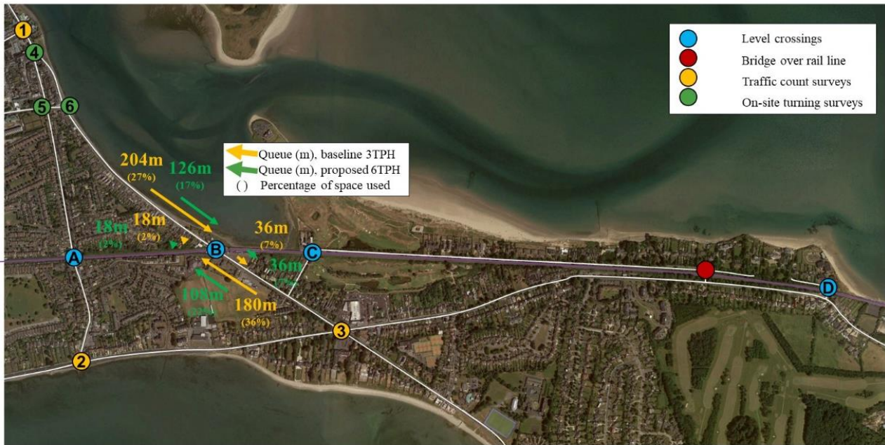
Figure 4-14 Comparison – Sutton (916) Level Crossing and Sutton Cross Junction SB Arm Queue Length Modelling Results – PM Peak
