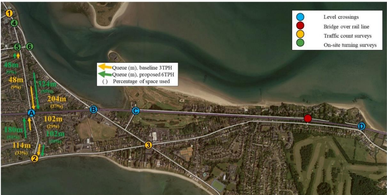
Figure 4-7 Comparison – Kilbarrack (917) Level Crossing and Dublin Road/Baldoyle Road Junction SB Arm Queue Length Modelling Results – AM Peak
