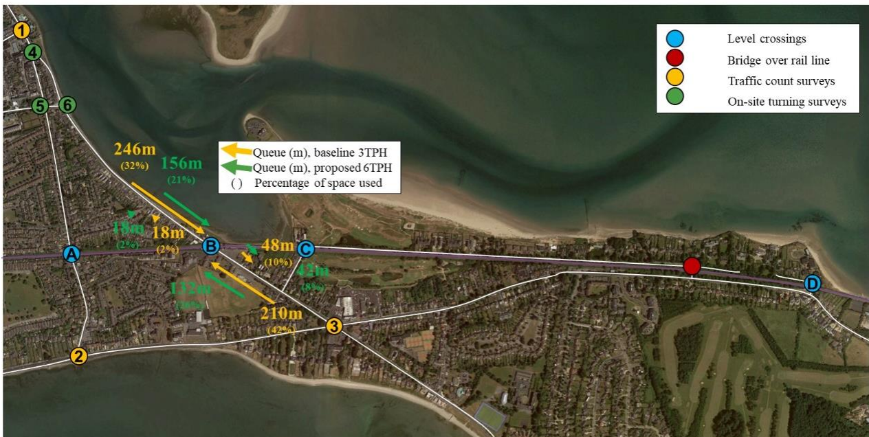
Figure 4-13 Comparison – Sutton (916) Level Crossing and Sutton Cross Junction SB Arm Queue Length Modelling Results – AM Peak
