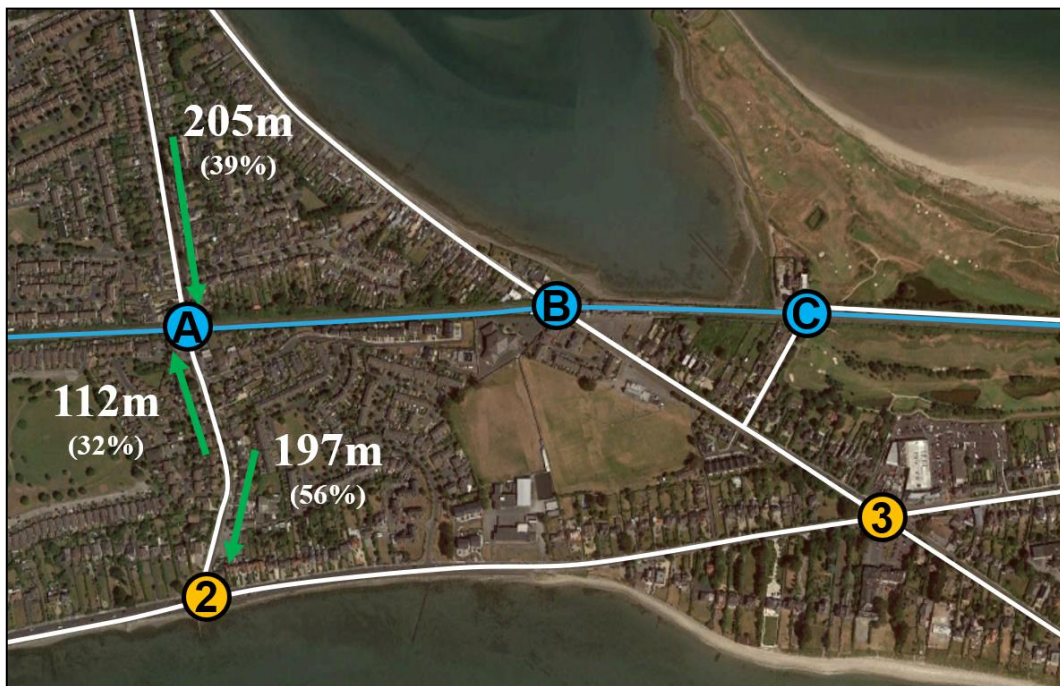
Figure 6-7: Proposed 6TPH Per Direction MMQ Results
