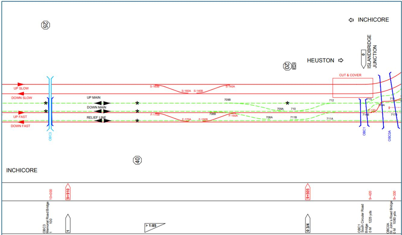
**Figure 7-8 Memorial Road Bridge (OBC3) to South Circular Road Bridge (OBC1)– Track Plan Layout**
