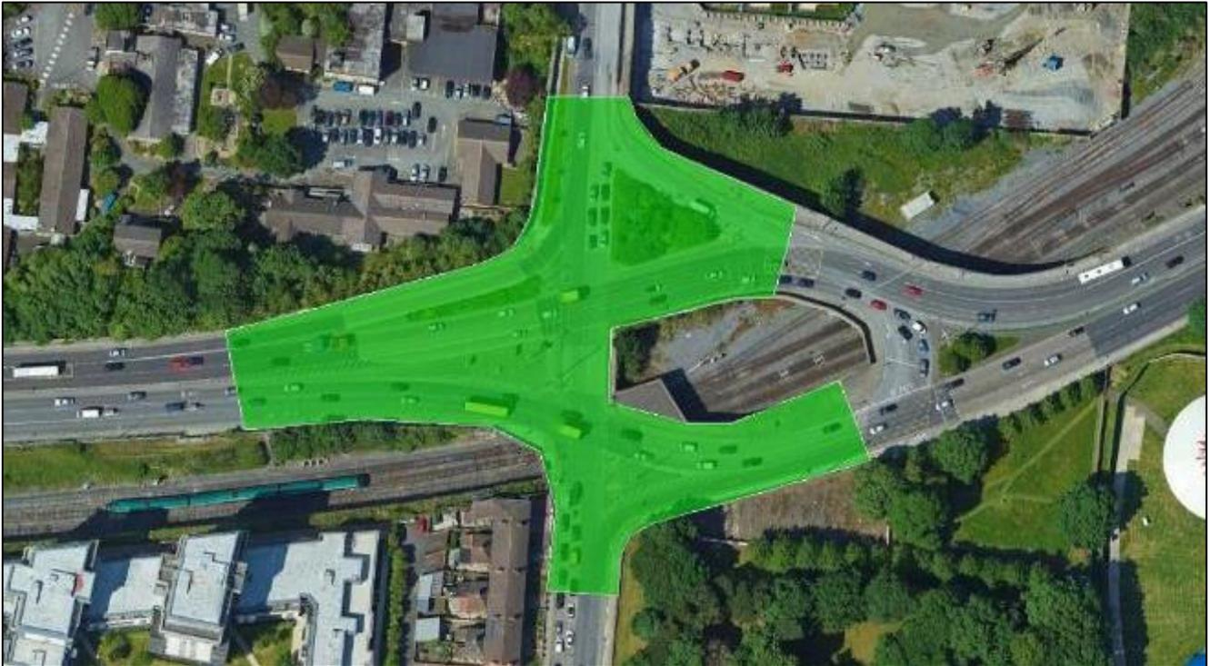
**Figure 5-4 Pavement construction impact for new road levels >0.6m above existing levels**
