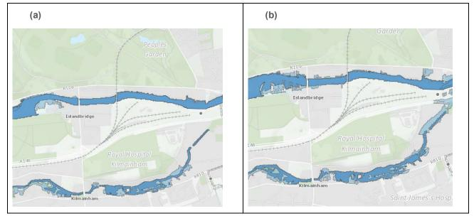
Figure 2.3: Present (a) & Future (mid-range) (b) Fluvial Flood extents - Liffey\_190 [Liffey]
