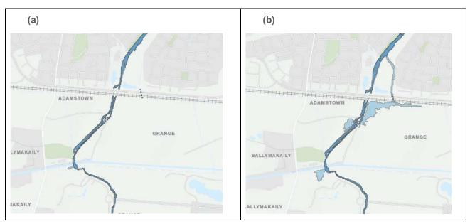
Figure 2.4: Present (a) & Future (mid-range) (b) Fluvial Flood extents - Liffey\_170 [Griffeen]
