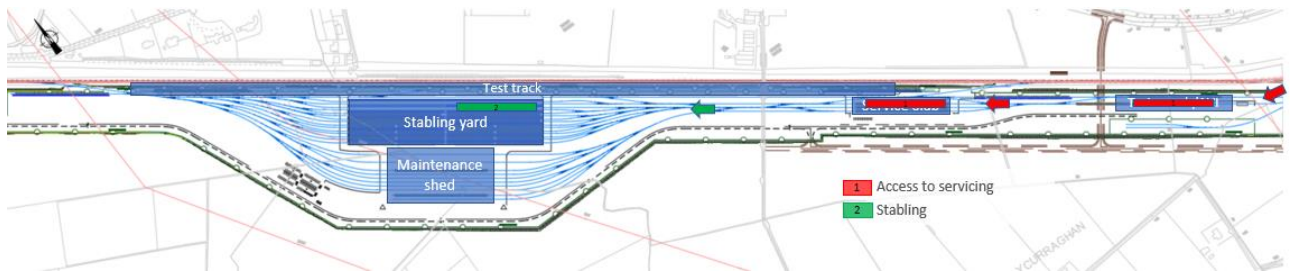
Figure 57: Movement 2: main line → service/washing → stabling (Alternative 3)
