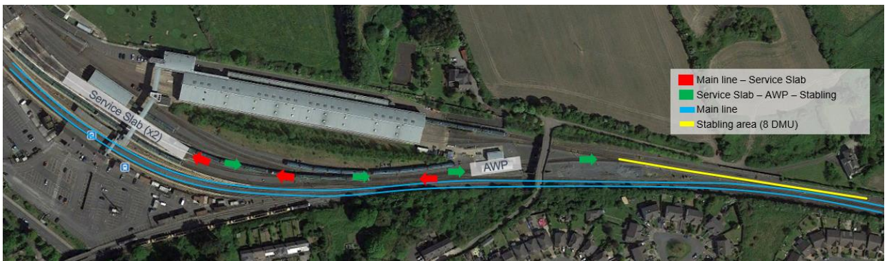
Figure 98: Main Line – Service Slab – AWP – Stabling
