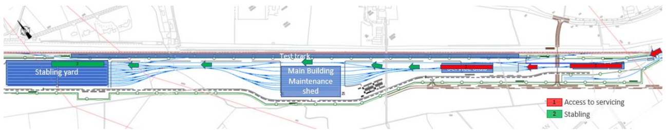
Figure 64: Movement 2: main line → service/washing → stabling (Alternative 4)
