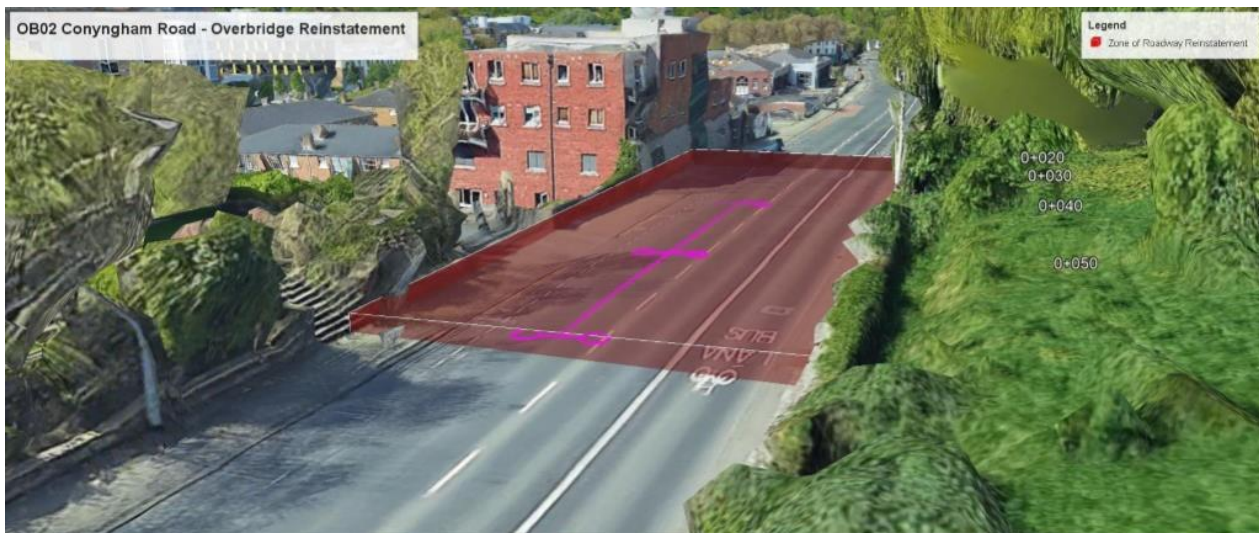
Figure 5-2 Extent of Roadworks Reinstatement at Conyngham Road Bridge (OBO2)
