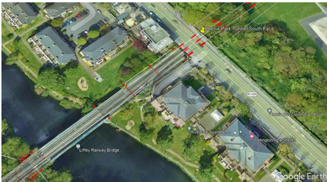
Figure 7-5 OHLE Mast position for Liffey Bridge and OBO2
