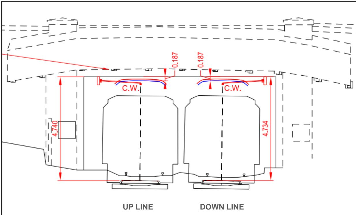
**Figure 7-16 Example cross section for fitted OHLE system in twin area.**
