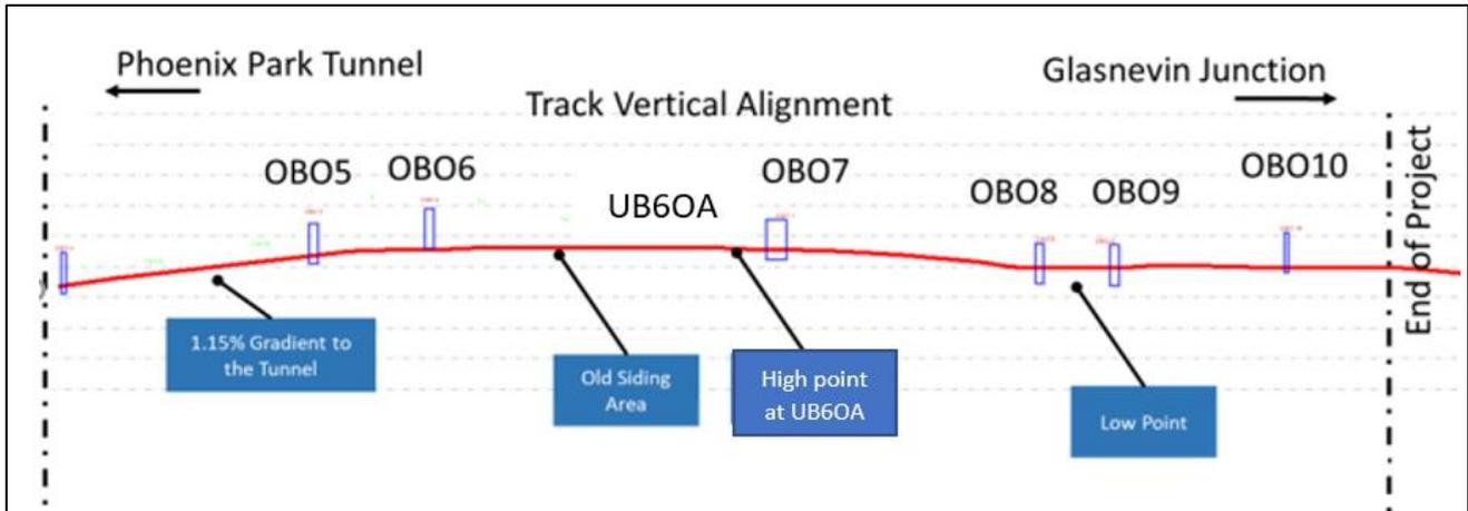
**Figure 2-15** Track vertical alignment
