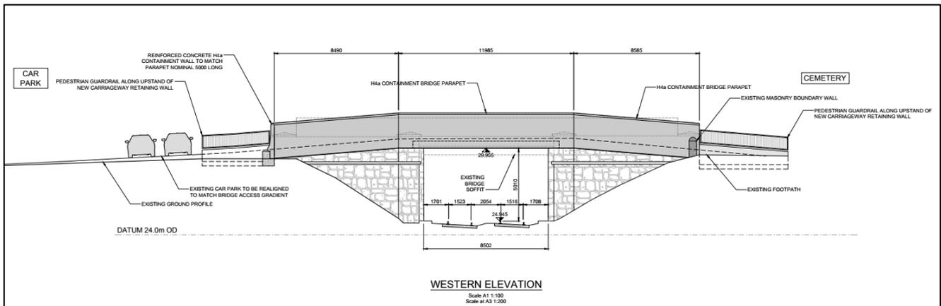
**Figure 7-2 Glasnevin Cemetery Bridge (OBO10) Longitudinal Section – Facing East**
