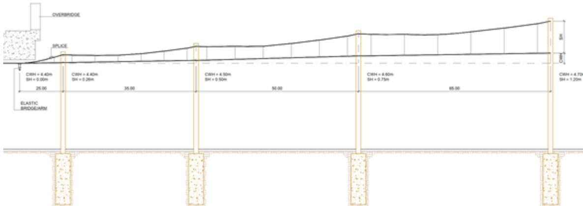
**Figure 3-3 Typical arrangement on approach to a low bridge**
