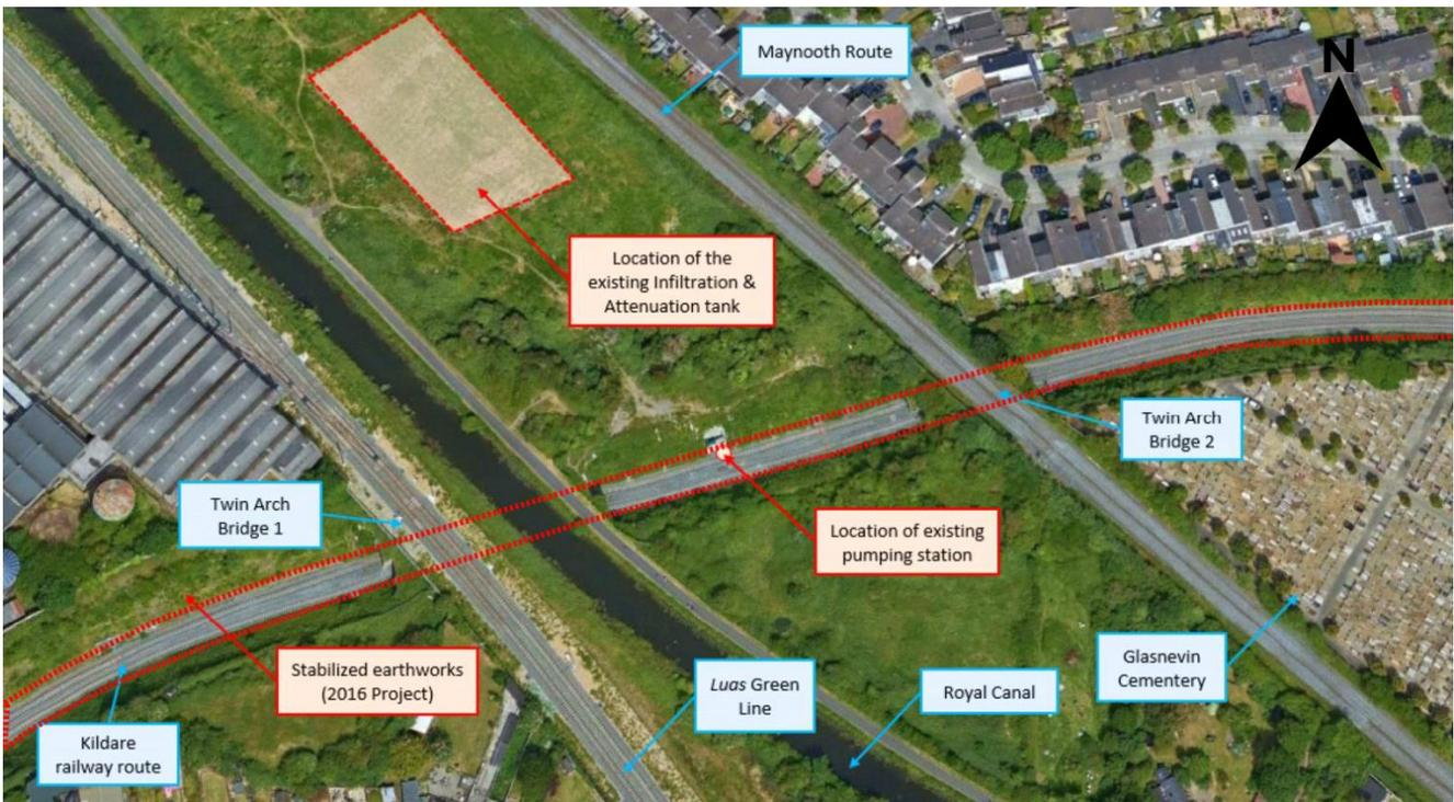
Figure 2-16 Location of drainage features and stabilization works.
