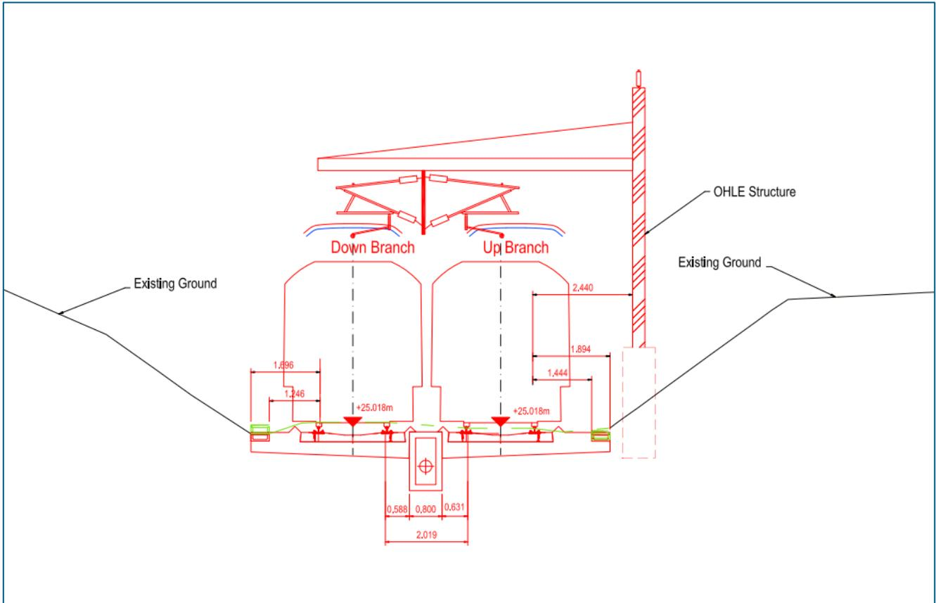
**Figure 7-9 Typical Cross section west of Glasnevin Cemetery Bridge (OBO10), view from Glasnevin Junction**
