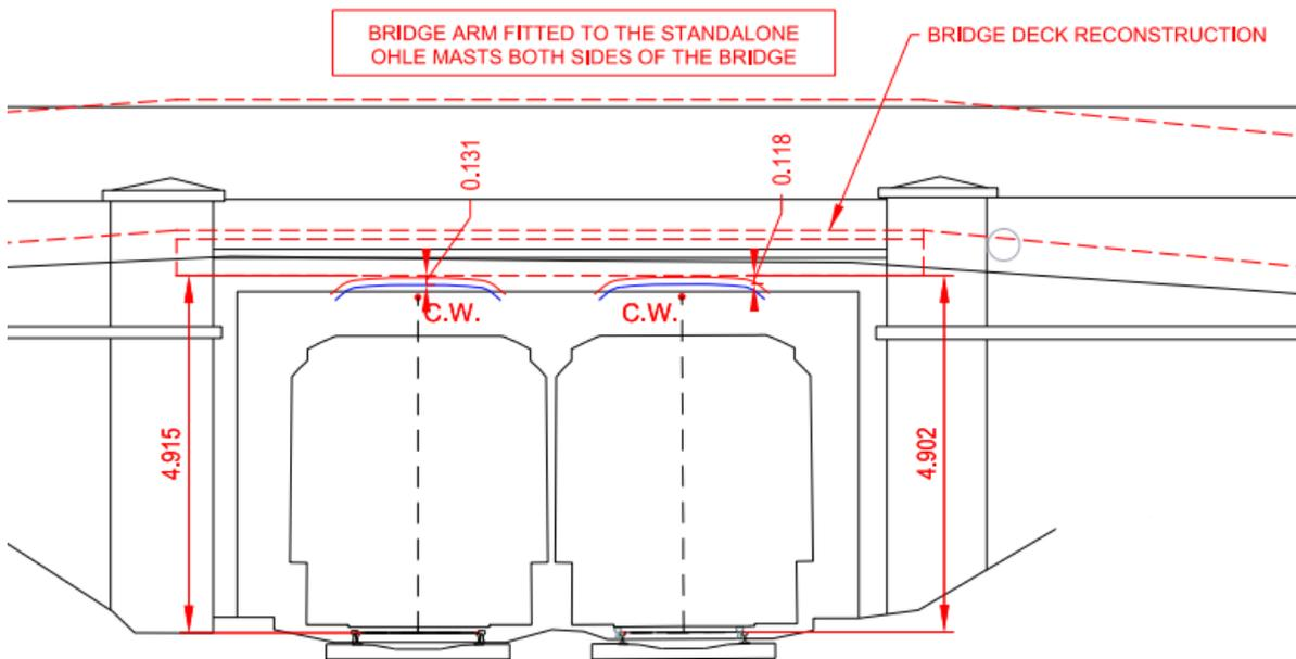
**Figure 7-18 Example cross section for fitted at each side of bridge**
