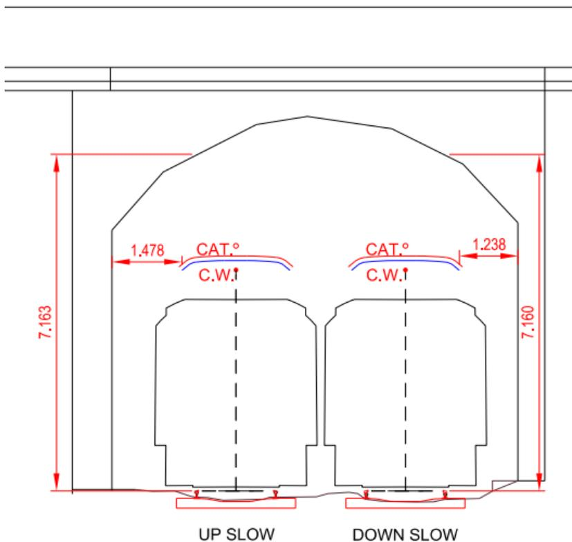
**Figure 7-15 Example cross section for free running OHLE system in twin area.**
