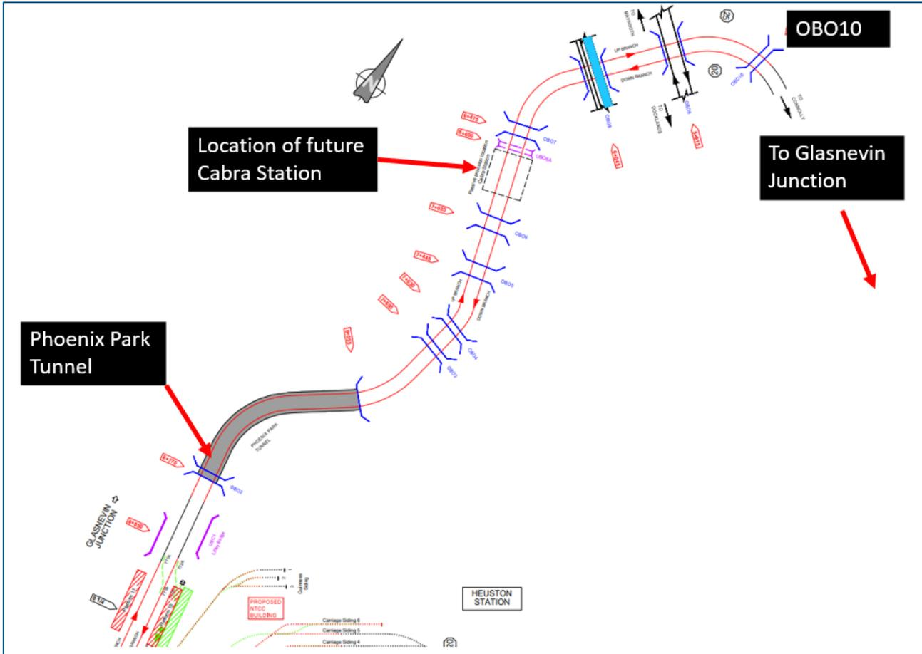
**Figure 7-8 Phoenix Park Tunnel to Glasnevin Cemetery Road Bridge (OBO10) – Track Plan Layout**
