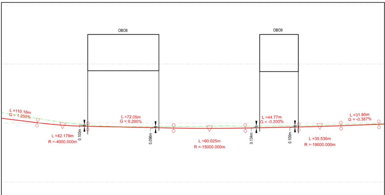
**Figure 2-4 Longitudinal profile between Royal Canal and LUAS Twin Arch Bridge (OBO8) and Maynooth Line Twin Arch Bridge (OBO9).**
