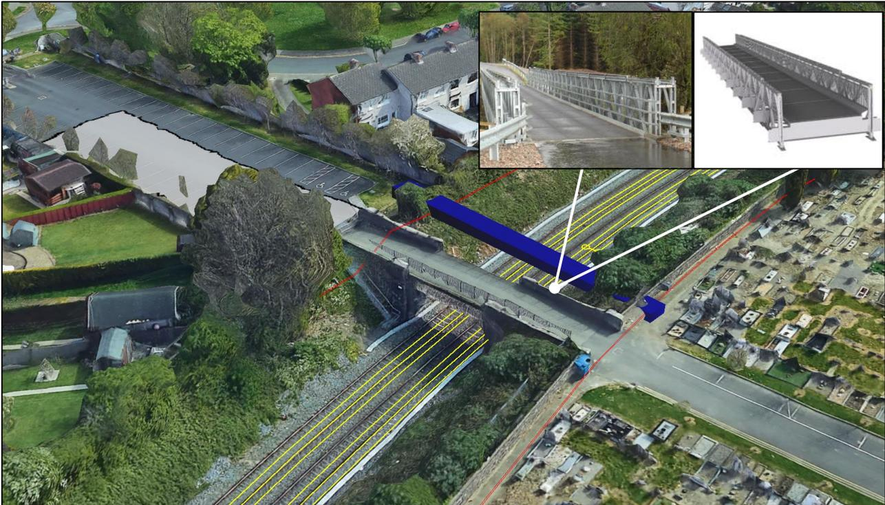
**Figure 8-5 Proposed temporary vulnerable user diversion (incl. bridge)**
