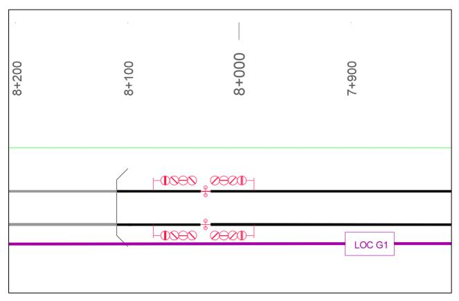
Figure 7-10 Signalling Scheme Plan (North Entrance at Phoenix Park Tunnel)
