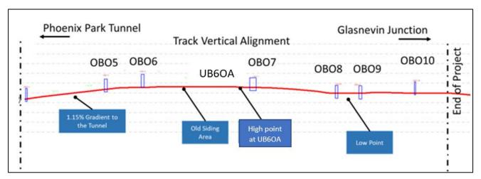
Figure 2-15 Track vertical alignment
