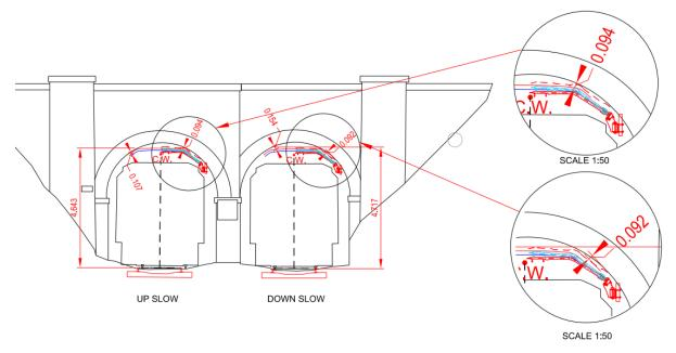
Figure 7-17 Example cross section for fitted tunnel arm OHLE system in twin area.
