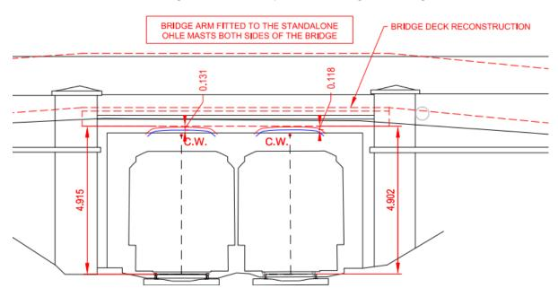
Figure 7-18 Example cross section for fitted at each side of bridge
