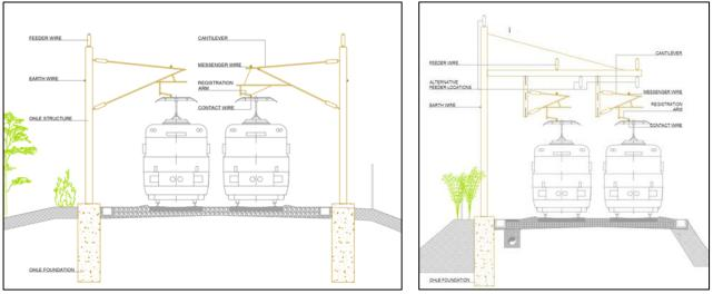
Figure 3-1 Typical OHLE arrangement in two track open route
