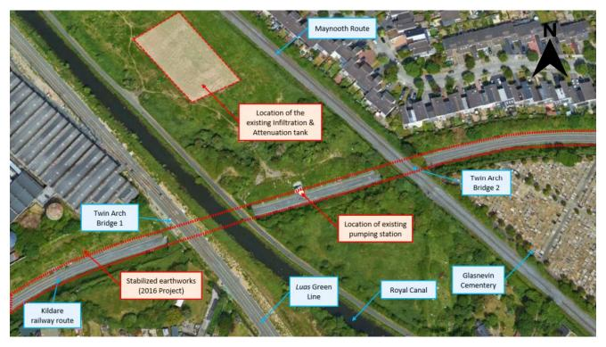
Figure 2-16 Location of drainage features and stabilization works.
