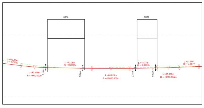
Figure 2-4 Longitudinal profile between Royal Canal and LUAS Twin Arch Bridge (OBO8) and Maynooth Line Twin Arch Bridge (OBO9).
