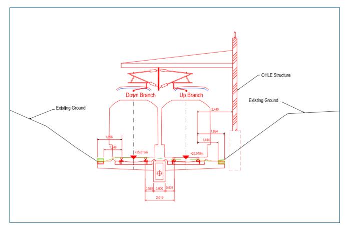
Figure 7-9 Typical Cross section west of Glasnevin Cemetery Bridge (OBO10), view from Glasnevin Junction
