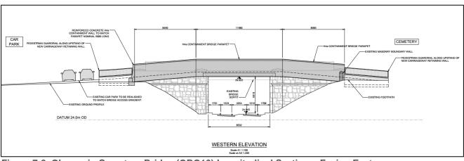
Figure 7-2 Glasnevin Cemetery Bridge (OBO10) Longitudinal Section – Facing East
