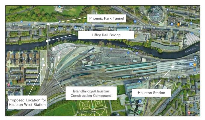
Figure 8-1 Heuston West Proposed Construction Compound Location
