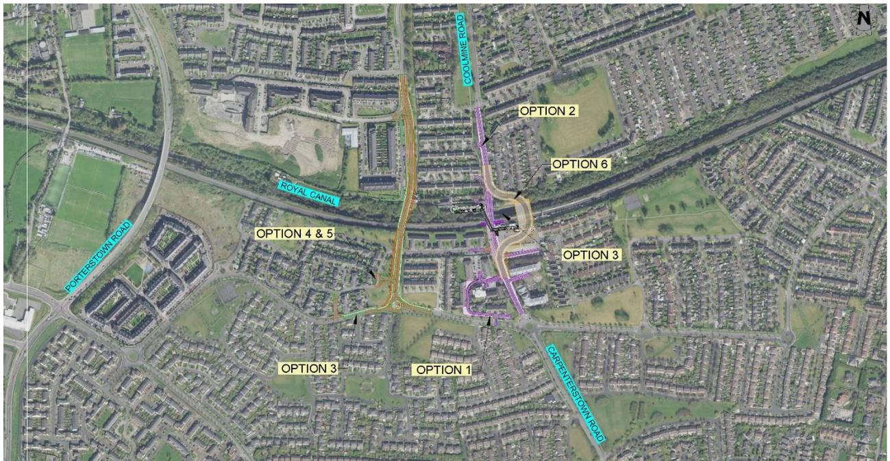
**Figure 4.2 Coolmine level crossing replacement options**
