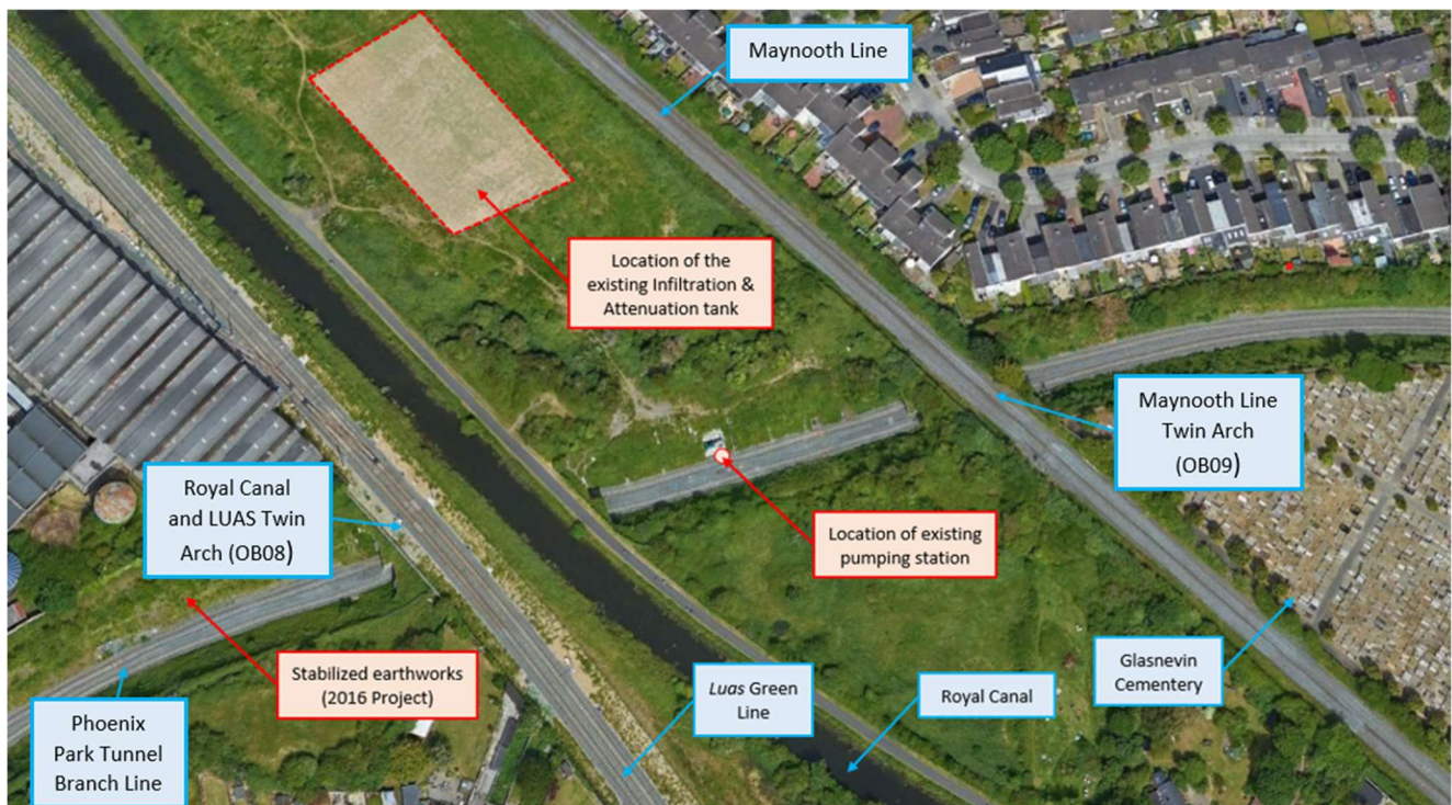
Figure 2-16 Location of drainage features and stabilization works.
