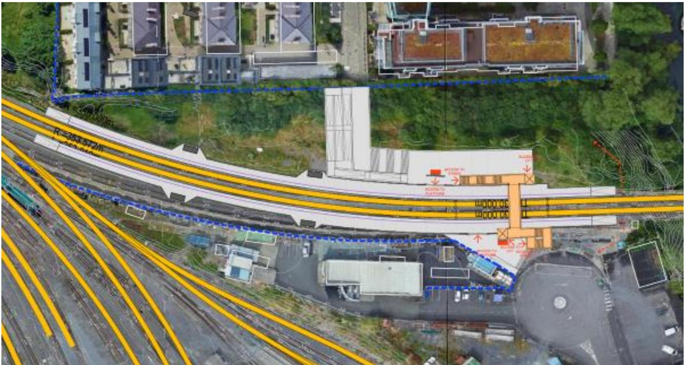
Figure 5-1 Station Option A – Footbridge with lift and stairs
