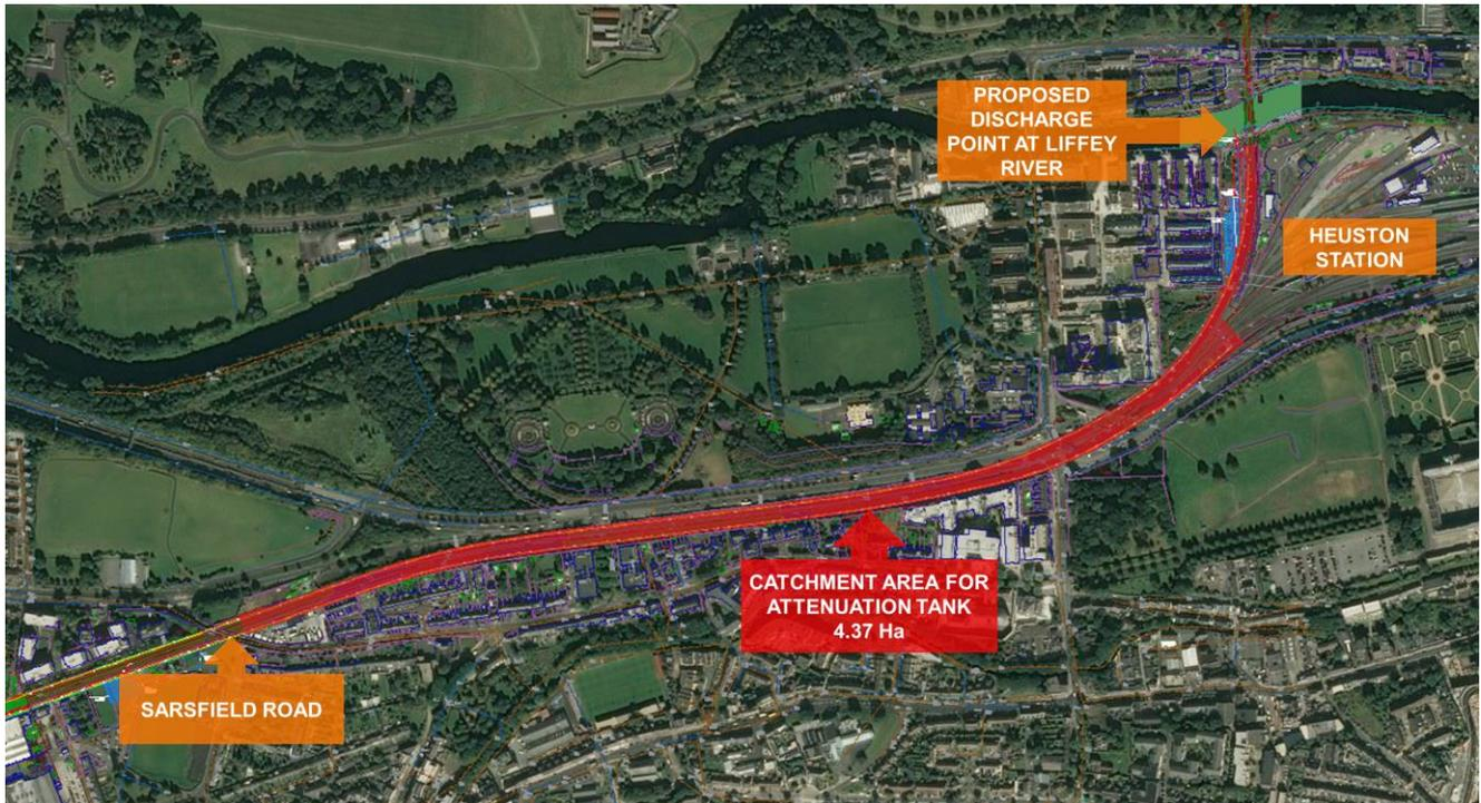
Figure 4-5:– Catchment area for the proposed attenuation tank
