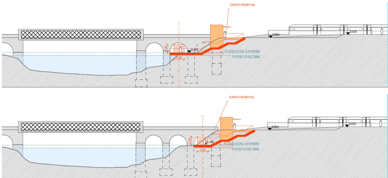
Figure 5-8 Station Option C - underpass with stairs and lifts – cross section options
