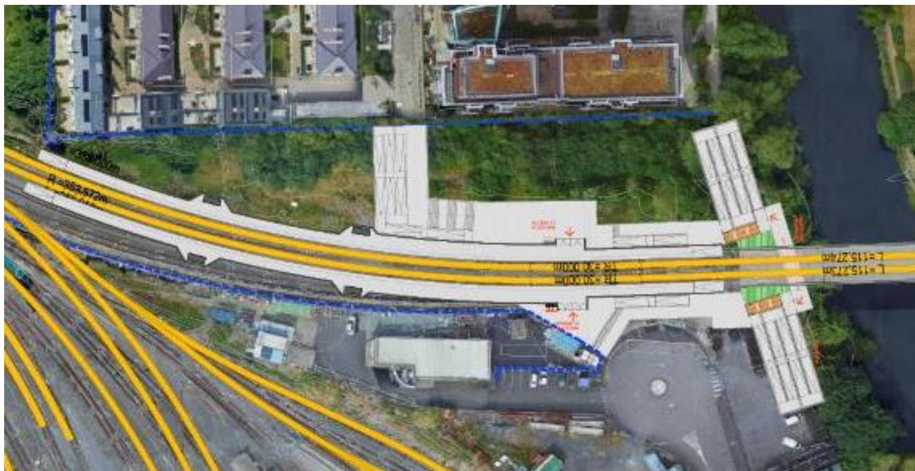
**Figure 5-9** Station Option D – underpass with ramp and stairs
