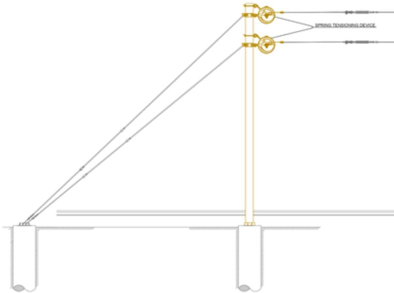
**Figure 3-2 Typical anchor structure**
