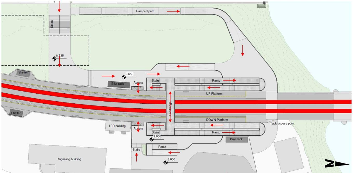
Figure 7-2 Proposed Heuston West Station Plan & Detailed Access Routes
