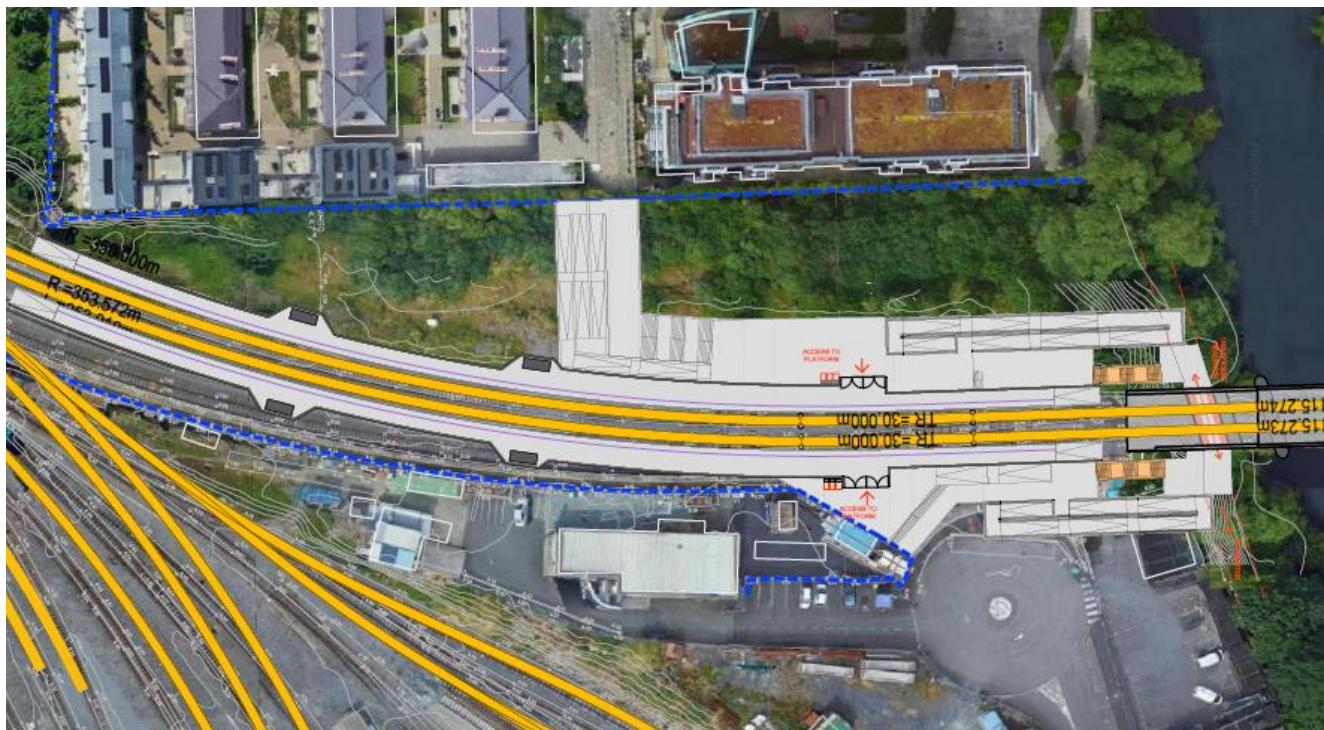
Figure 5-11 Station Option E – underpass with ramp and stairs
