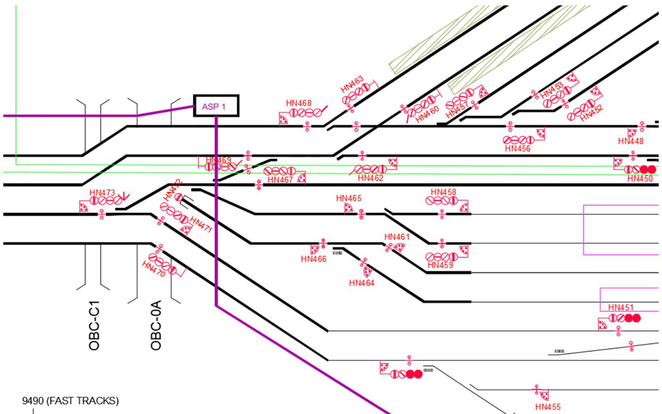
**Figure 7-8 Signalling Scheme Plan (Heuston Station)**
