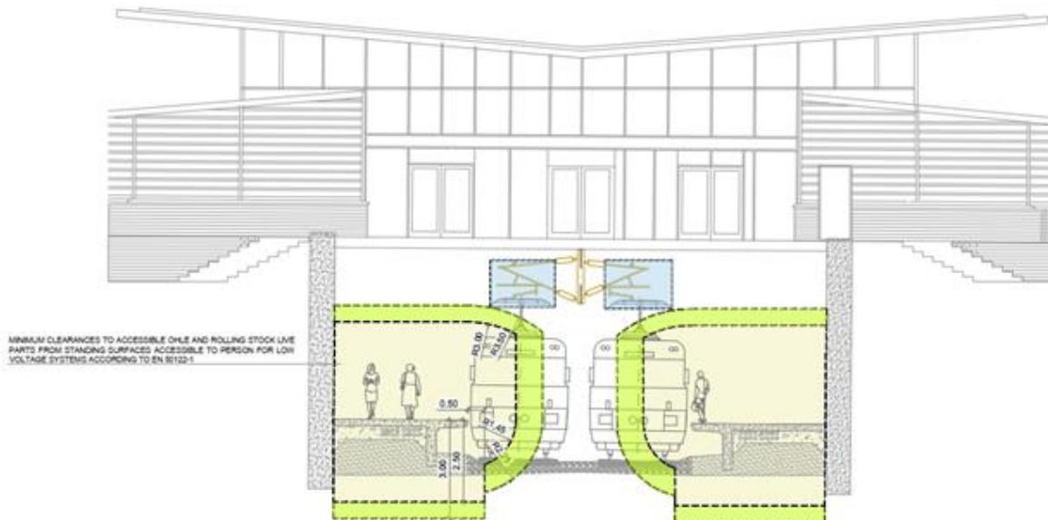
Figure 7-15 Example OHLE system in station area with clearance
