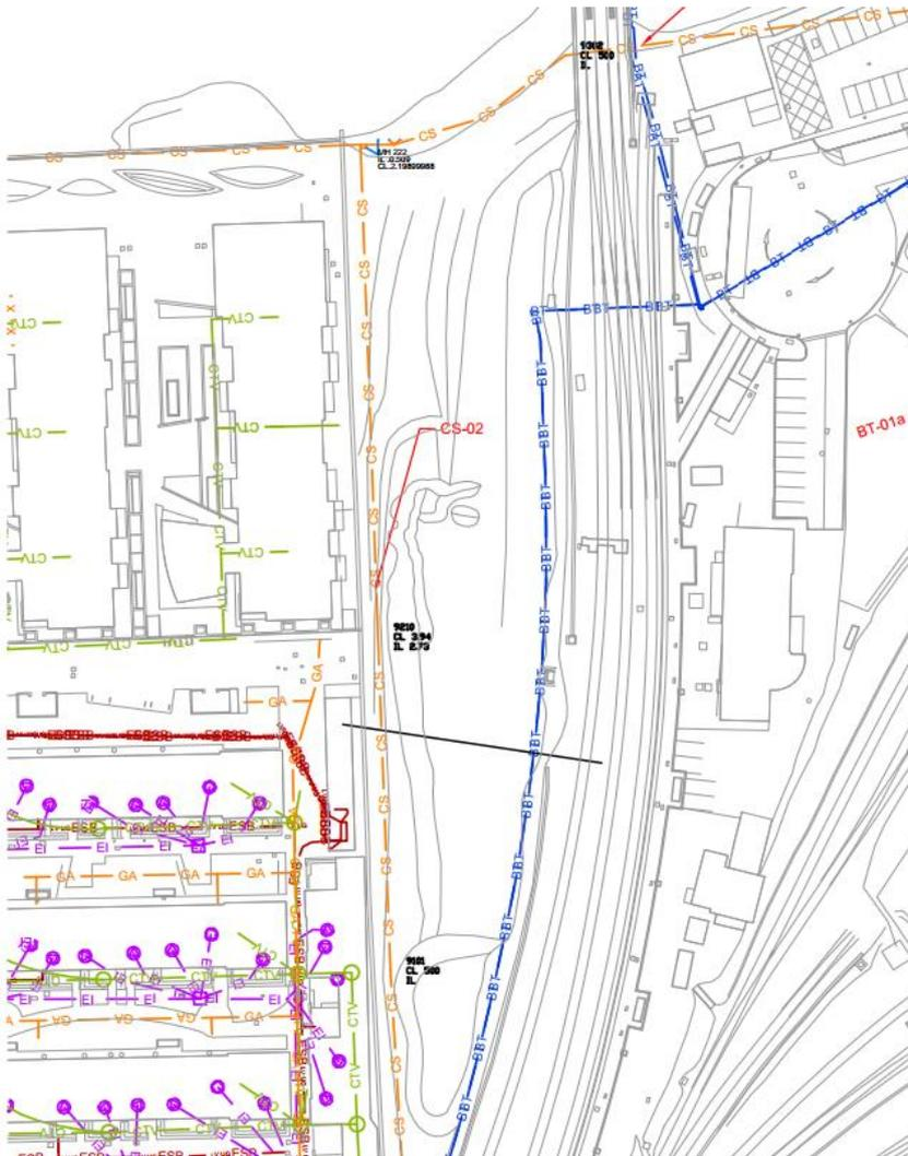
Figure 4-1 Utilities beneath Proposed Heuston West Station
