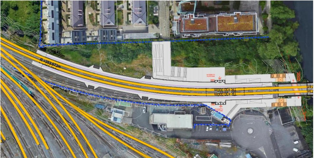
Figure 5-7 Station Option C – underpass with stairs and lifts
