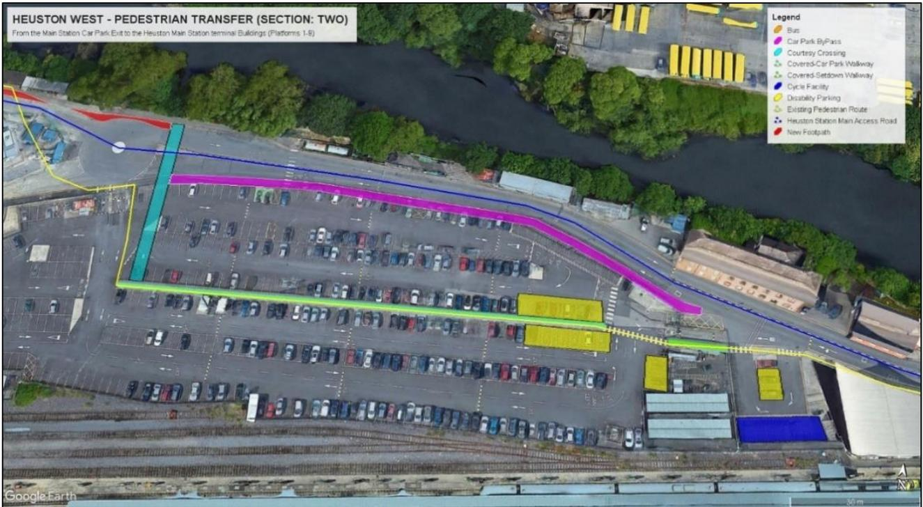
Figure 6-3 Area Two – Pedestrian Route Layout plan
