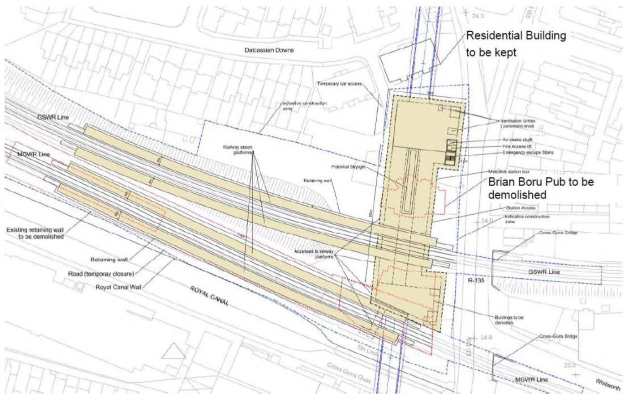
**Figure 12 Plan of proposed interchange station at Glasnevin (Jacobs and IDOM Metrolink study)**
