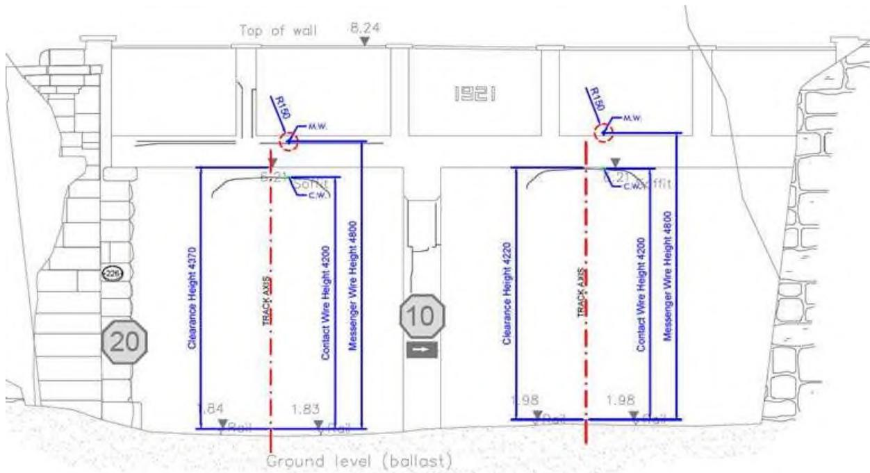
**Figure 9 Vertical clearance for the OHLE under the existing bridge**
