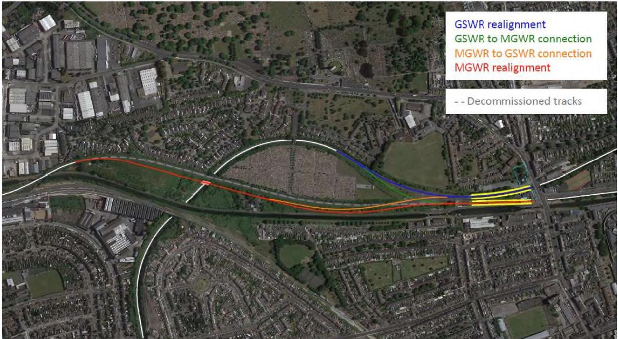
Figure 13 Lines 2 and 3 in the Glasnevin Jct. area (Jacobs and IDOM Metrolink study)
