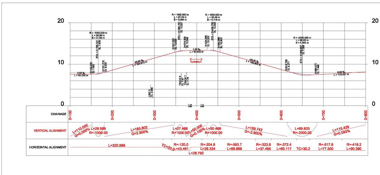
Figure 3 Connolly station – option 1 – vertical alignment
