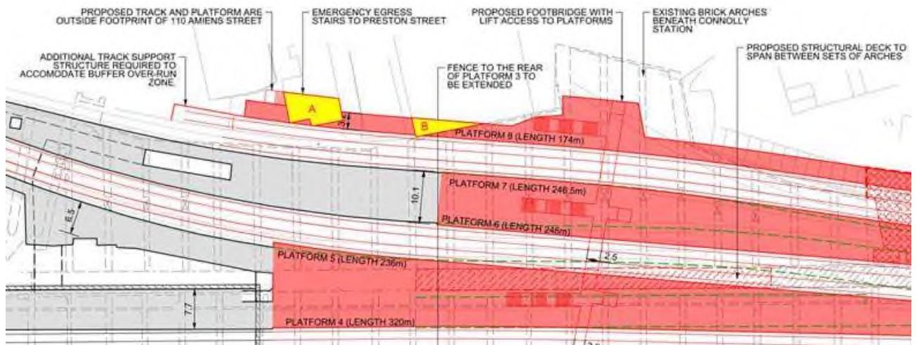
Figure 6 Connolly station – potential platform 8 layout and conflicts with existing structures
