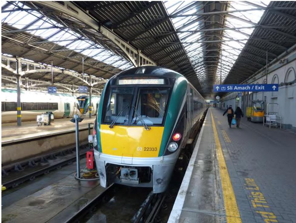
Figure 28 Train Class 22000 (DMU – ICR)
