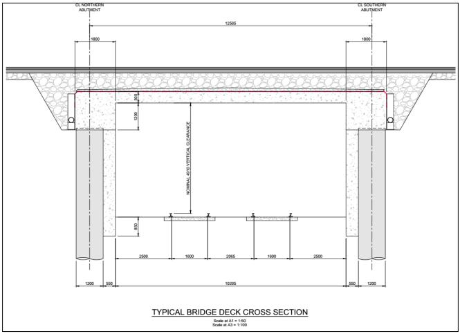
Figure 7-3 New South Circular Road Bridge (OBC1A) Cross Section (Southbound Lane)
