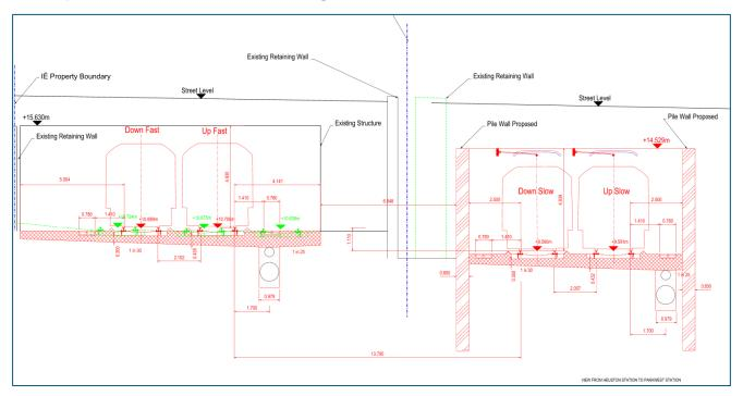
Figure 7-10 South Circular Road Bridge (OBC1) – Cross section at Ch 9+401, view from Heuston Station to Park West & Cherry Orchard Station
