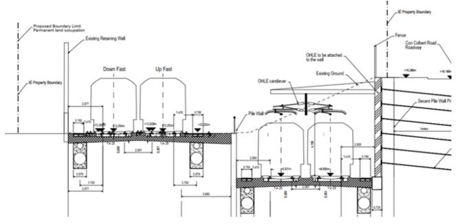
Figure 7-5 Chapelizod Bypass (Con Colbert Road) Retaining Wall & Ground Anchors – Facing West
