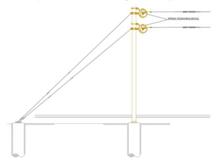
Figure 3-2 Typical anchor structure
