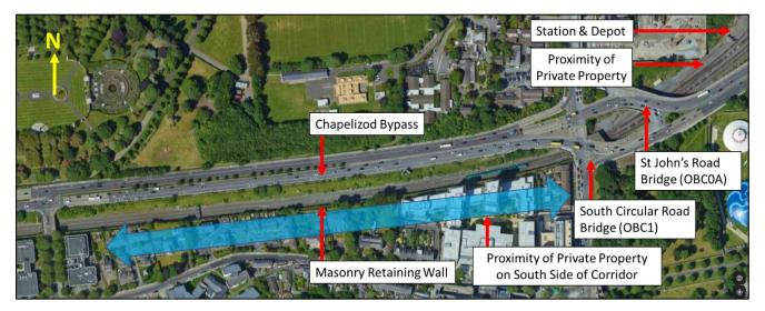
Figure 4-1 Constraints of permanent way design
