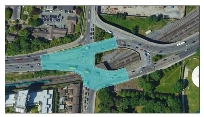
Figure 5-3 Pavement construction impact with road reinstatement at grade
