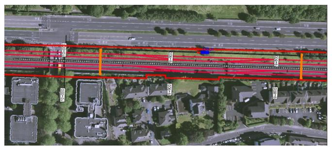
Figure 7-12 Signalling Infrastructure (Memorial Road – South Circular Road Junction)
