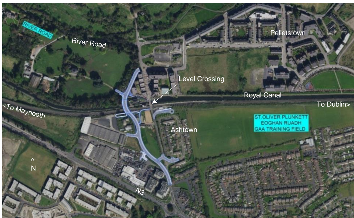
Figure ES-9 Ashtown Option 2 - Emerging Preferred Option at Ashtown Level Crossing Replacement
