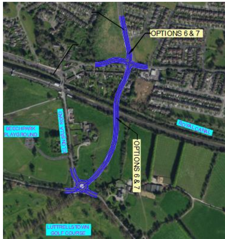
Figure 9-54 Option 6 Overbridge 200m to the East – Online of Larchgrove & Option 7 Overbridge 200 metres to the East – Online of Larchgrove with retaining walls (Copyright Ordnance Survey Ireland – 0039720)
