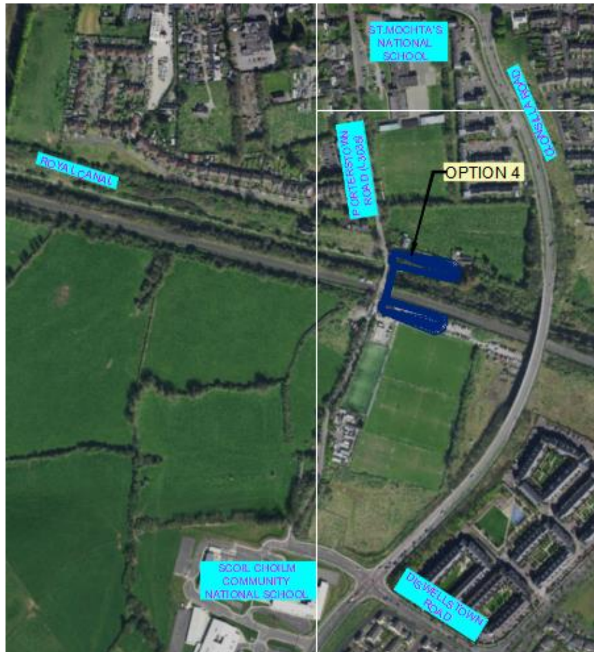
Figure 9-47 Option 4 Pedestrian and Cycle Bridge – Alternative Nested Ramp (Copyright Ordnance Survey Ireland – 0039720)
