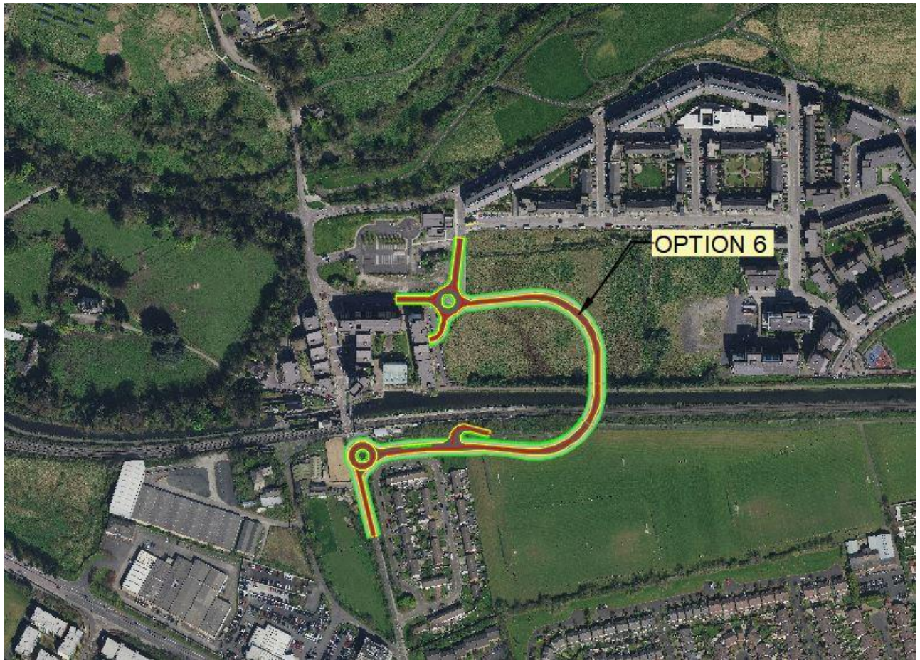
Figure 9-31 Ashtown Option 6 – Overbridge 250m east of existing crossing (Copyright Ordnance Survey Ireland – 0039720)
