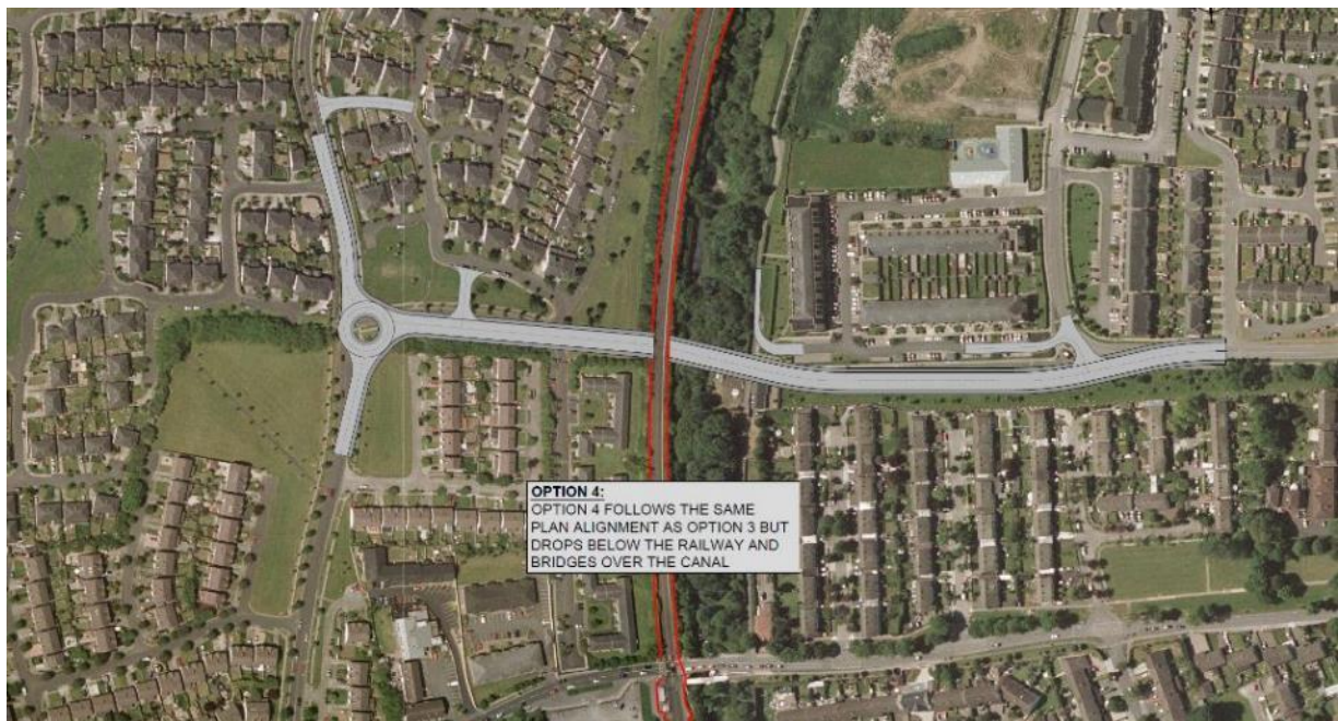
Figure 9-38 Coolmine Option 4 – New Underbridge with Opening Canal Bridge Connecting St. Mochta’s Grove to Riverwood Court (Copyright Ordnance Survey Ireland – 0039720)
