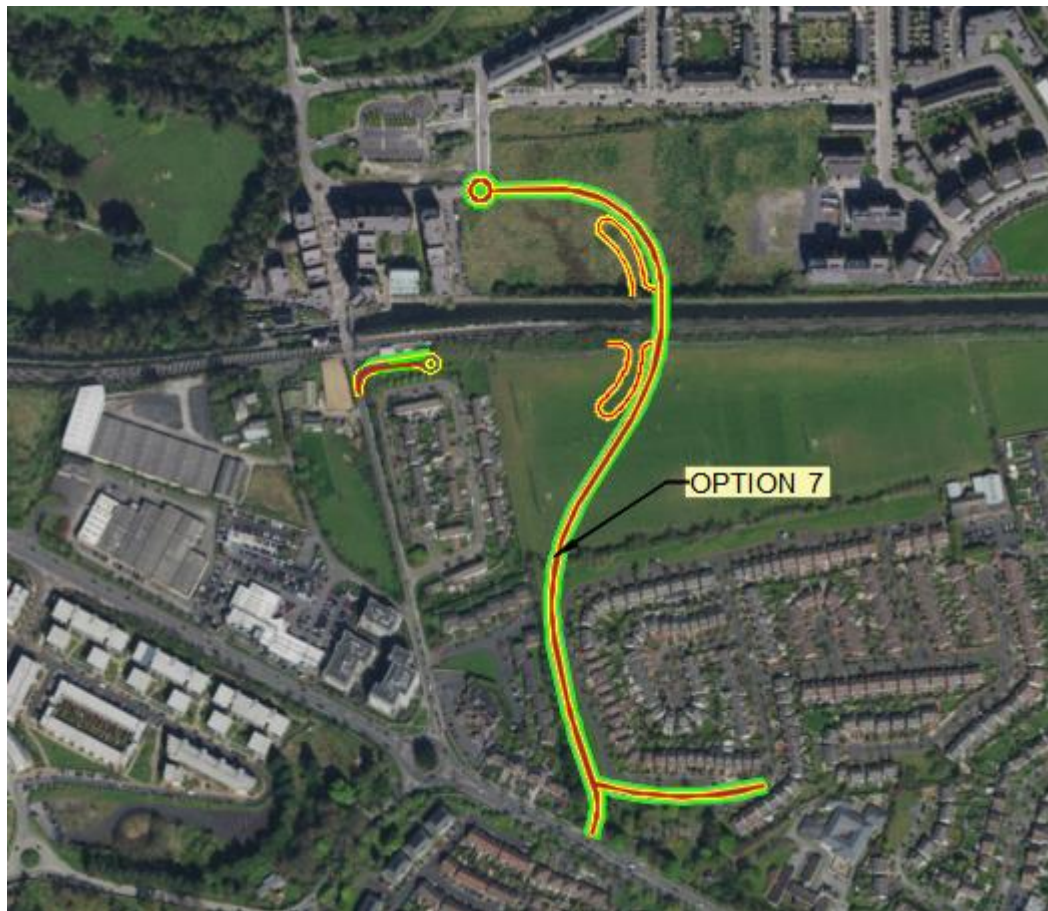
Figure 9-32 Ashtown Option 7 – Overbridge with connection to the N3 Navan Road (Copyright Ordnance Survey Ireland – 0039720)
