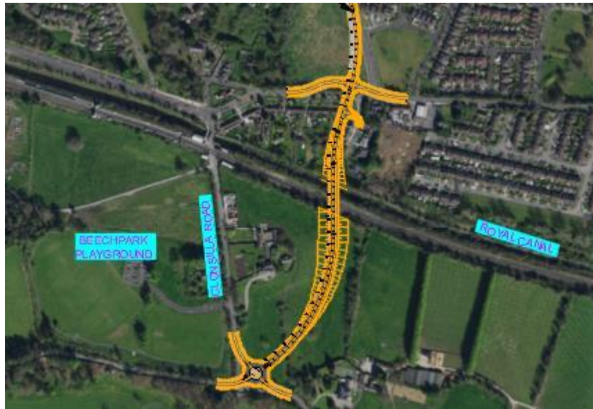
Figure 9-53 Option 5 Overbridge 200m to the East – Reduced Carriageway (Copyright Ordnance Survey Ireland – 0039720)
