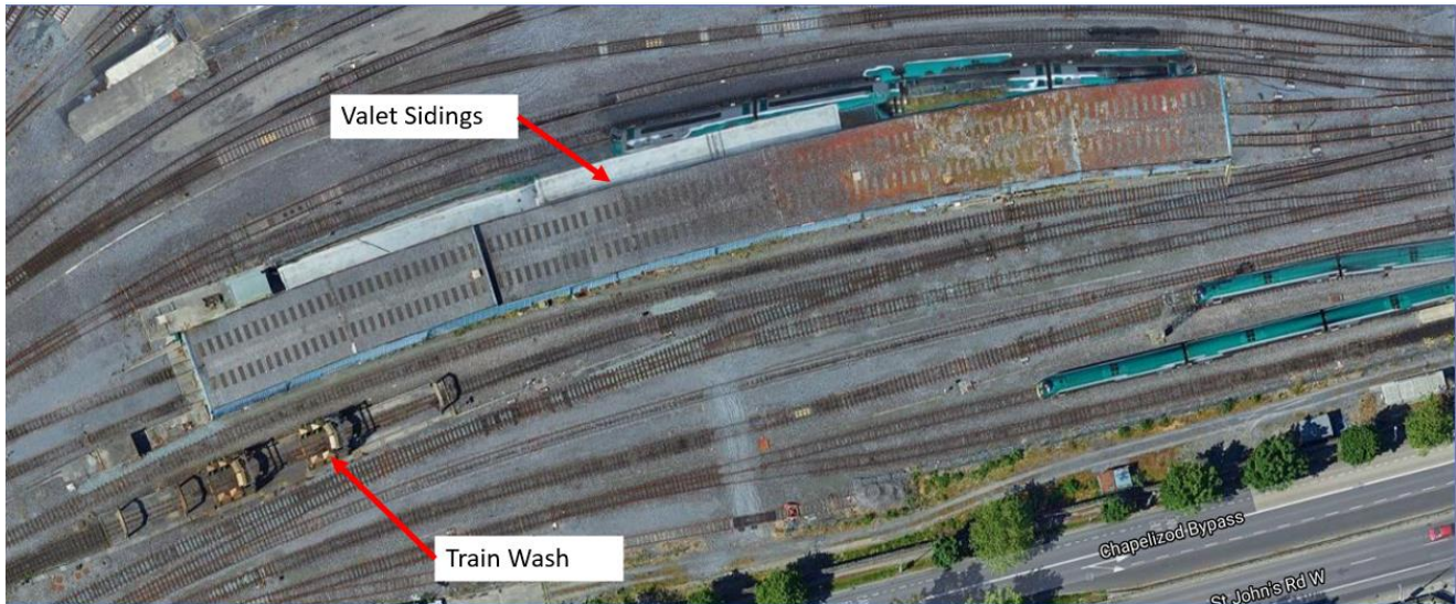
Figure 2-6 Train Wash Road and Valet Sidings
