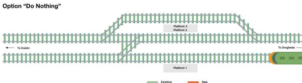
**Figure 5-1: Schematic of ‘do-nothing’ option**
