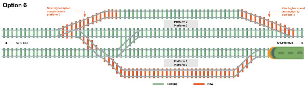
Figure 5-13: Schematic of Option 6
