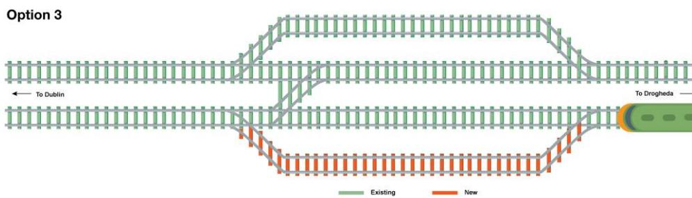
Figure 5-5: Schematic of Option 3
