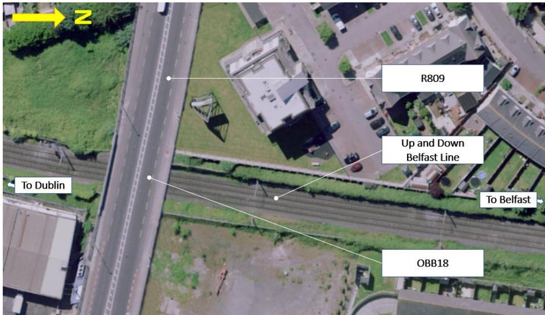
**Figure 2-2: Aerial view on OBB18 carrying the R809 over the Up and Down Belfast Lines (source: OSI aerial mapping)**
