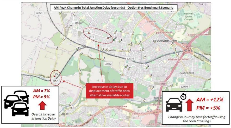
Figure 6.23 AM Change in Junction Delay - Option6 vs Benchmark Scenario
