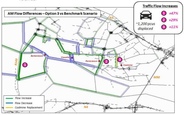
Figure 6.12 AM Flow Difference Plot - Option3 vs Benchmark Scenario
