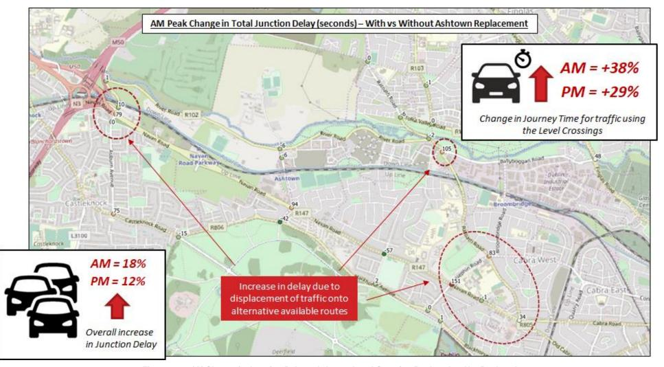
Figure 6.26 AM Change in Junction Delay – Ashtown Level Crossing Replaced vs Not Replaced
