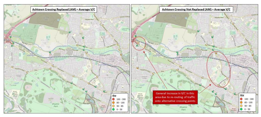
Figure 6.25 AM Average V/C – Ashtown Level Crossing Replaced vs Not Replaced
