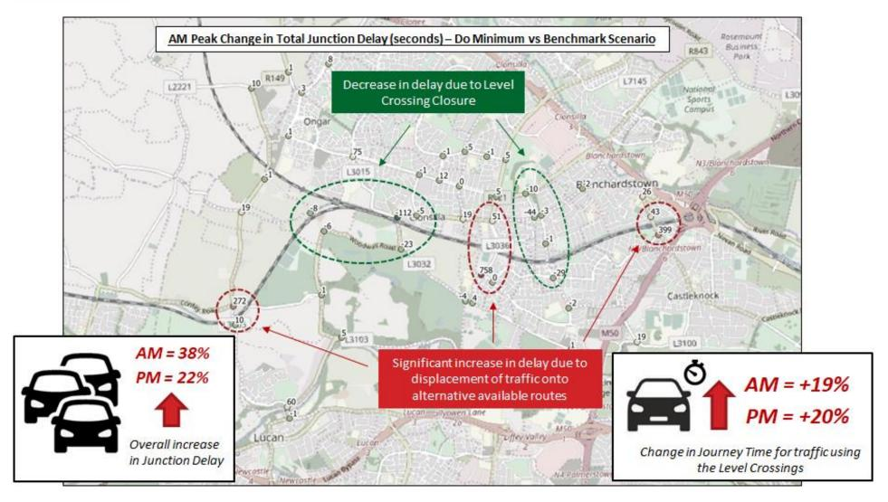
Figure 6.5 AM Change in Junction Delay – Do Minimum vs Benchmark Scenario
