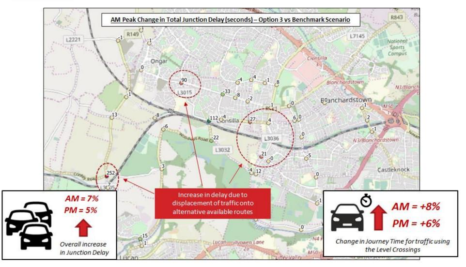
Figure 6.14 AM Change in Junction Delay - Option3 vs Benchmark Scenario
