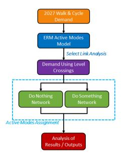
Analysis of Results/Outputs: Key outputs from the active assignment were assessed to identify the impact on travel time, and distance, for pedestrian and cyclists if the level crossings are closed.
