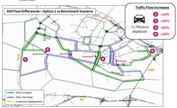
Figure 6.6 AM Flow Difference Plot - Option1 vs Benchmark Scenario
