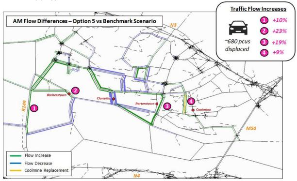
Figure 6.18 AM Flow Difference Plot - Option5 vs Benchmark Scenario
