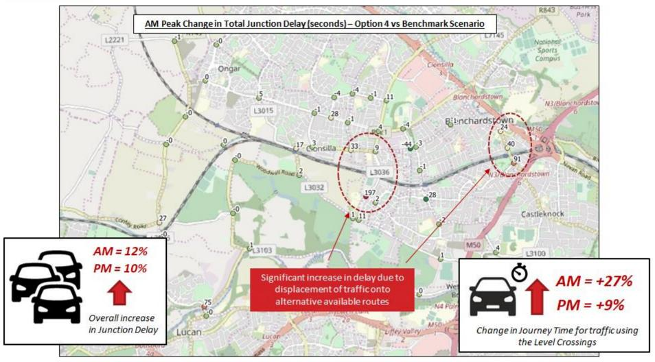
Figure 6.17 AM Change in Junction Delay – Option4 vs Benchmark Scenario
