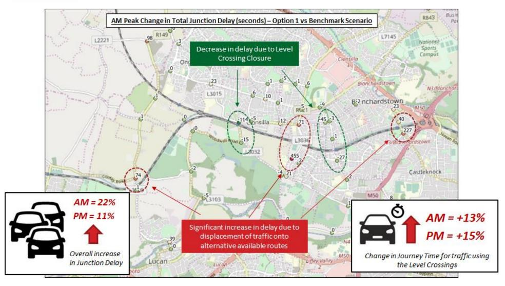
Figure 6.8 AM Change in Junction Delay – Option1 vs Benchmark Scenario
