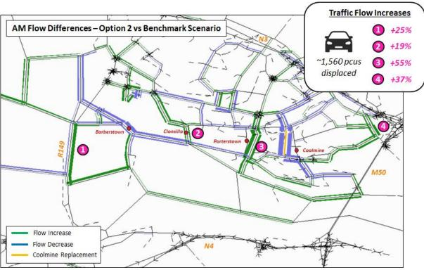
Figure 6.9 AM Flow Difference Plot - Option2 vs Benchmark Scenario
