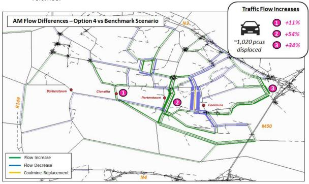
Figure 6.15 AM Flow Difference Plot - Option4 vs Benchmark Scenario
