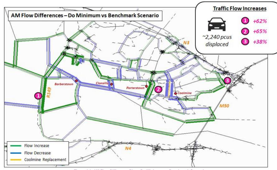
Figure 6.3 AM Flow Difference Plot – Do Minimum vs Benchmark Scenario
