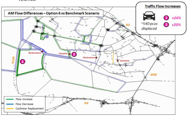
Figure 6.21 AM Flow Difference Plot - Option6 vs Benchmark Scenario
