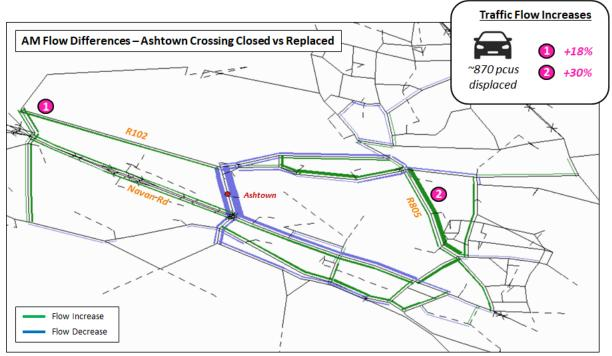
Figure 6.24 AM Flow Difference Plot - Option7 vs Benchmark Scenario
