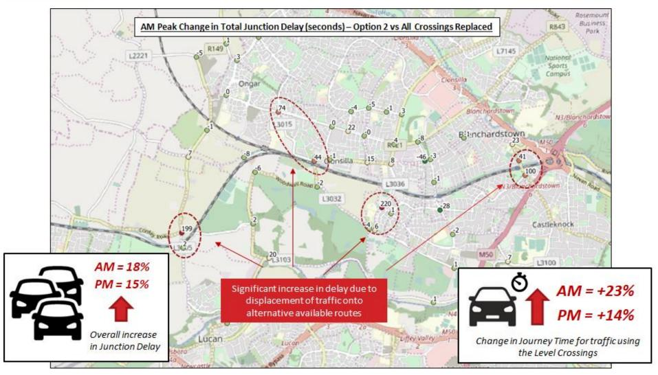
Figure 6.11 AM Change in Junction Delay - Option2 vs Benchmark Scenario
