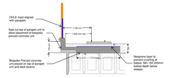
Figure 4-11: UBB36 Proposed Option A
