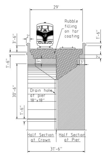
Figure 8-2: Boyne Viaduct typical cross-section
