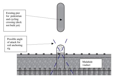
Figure 3-21: UBB30 Ground anchors option (Plan)
