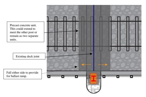
Figure 3-17: UBB30 – Proposed precast unit option (plan)
