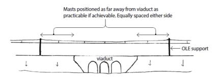
Figure 2-1: Approach to longitudinal frame arrangement for underbridges with lengths < 60m
