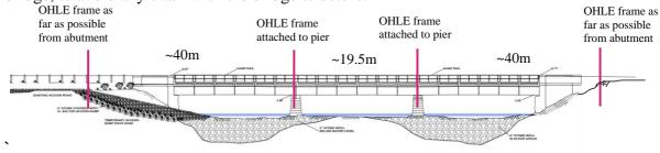
Figure 4-10: UBB36 OHLE longitudinal arrangement – Arrangement 2
