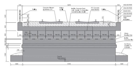
Figure 3-3: UBB30 Typical section for spans 4 and 5 (spans replaced following collapse)
