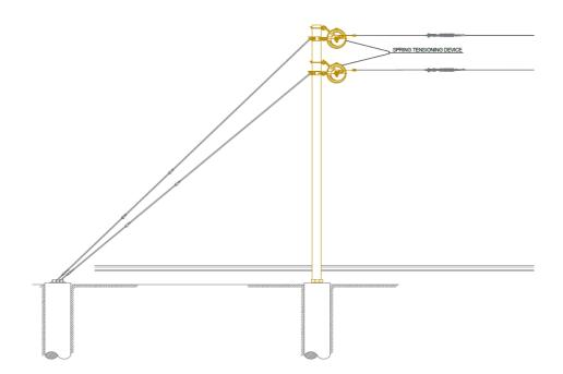
**Figure 2-3: Tensioning Device**
