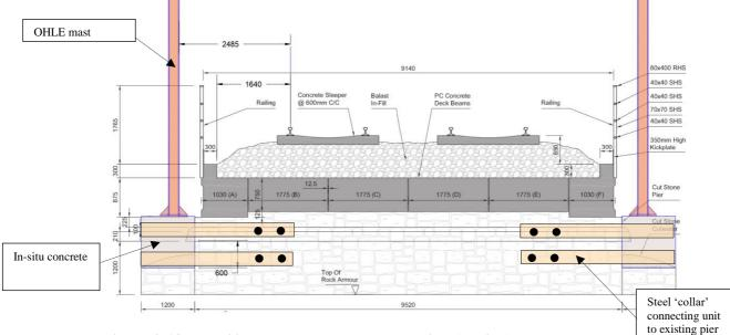
Figure 3-18: UBB30 – Proposed steel collar option (section)
