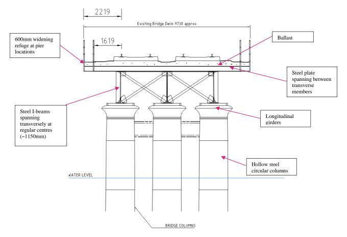
Figure 7-2: UBB72 Cross-section
