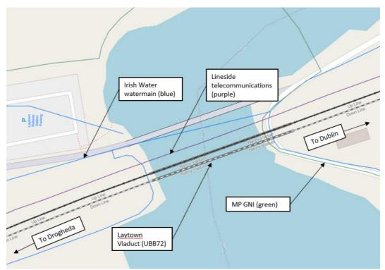
Figure 7-8: Plan of Laytown Viaduct (UBB72) showing existing utilities. (Map data © OpenStreetMap contributors, Map layer by Esri)
