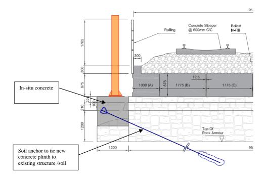
Figure 3-20: UBB30 - Ground anchors option (section)
