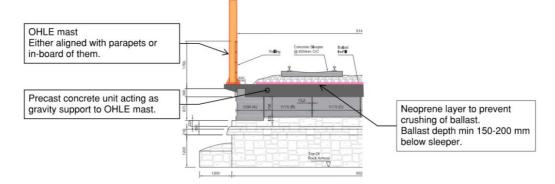
Figure 3-16: UBB30 – Proposed precast unit option (section)
