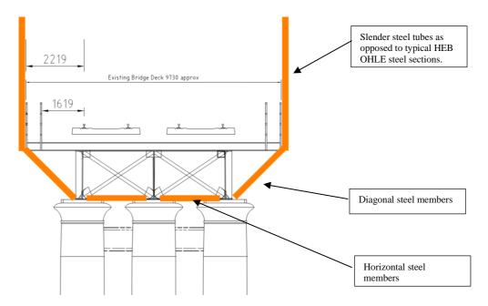
Figure 7-14: Proposed OHLE option - cross-section
