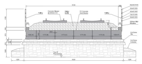
Figure 3-2: UBB30 Typical section for spans 2, 3 and 6 to 11
