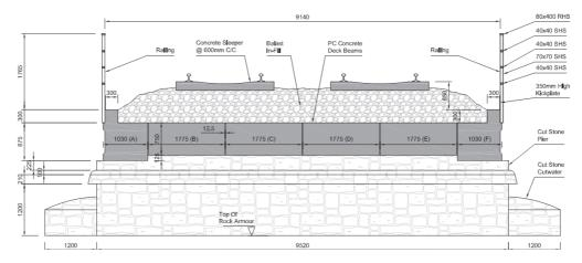
Figure 3-1: UBB30 Typical section for spans 1 and 12 (end spans)
