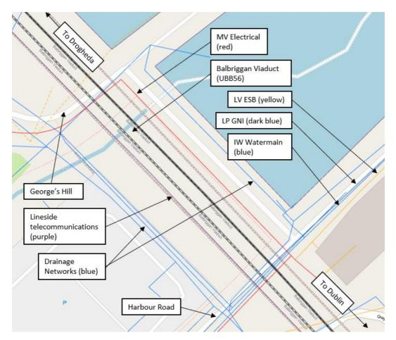
Figure 5-6: Plan of Balbriggan Viaduct (UBB56) showing existing utilities. (Map data © OpenStreetMap contributors, Map layer by Esri)
