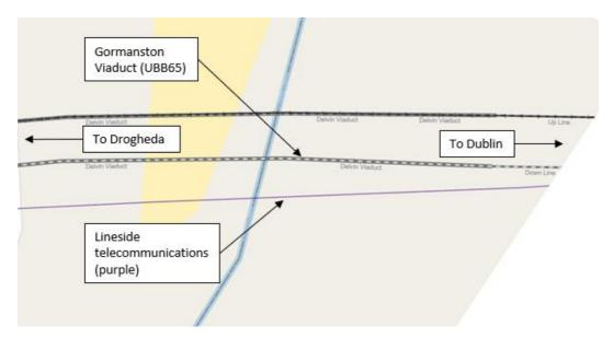
Figure 6-5: Plan of Gormanston Viaduct (UBB65) showing existing utility routes (Map data © OpenStreetMap contributors, Map layer by Esri)
