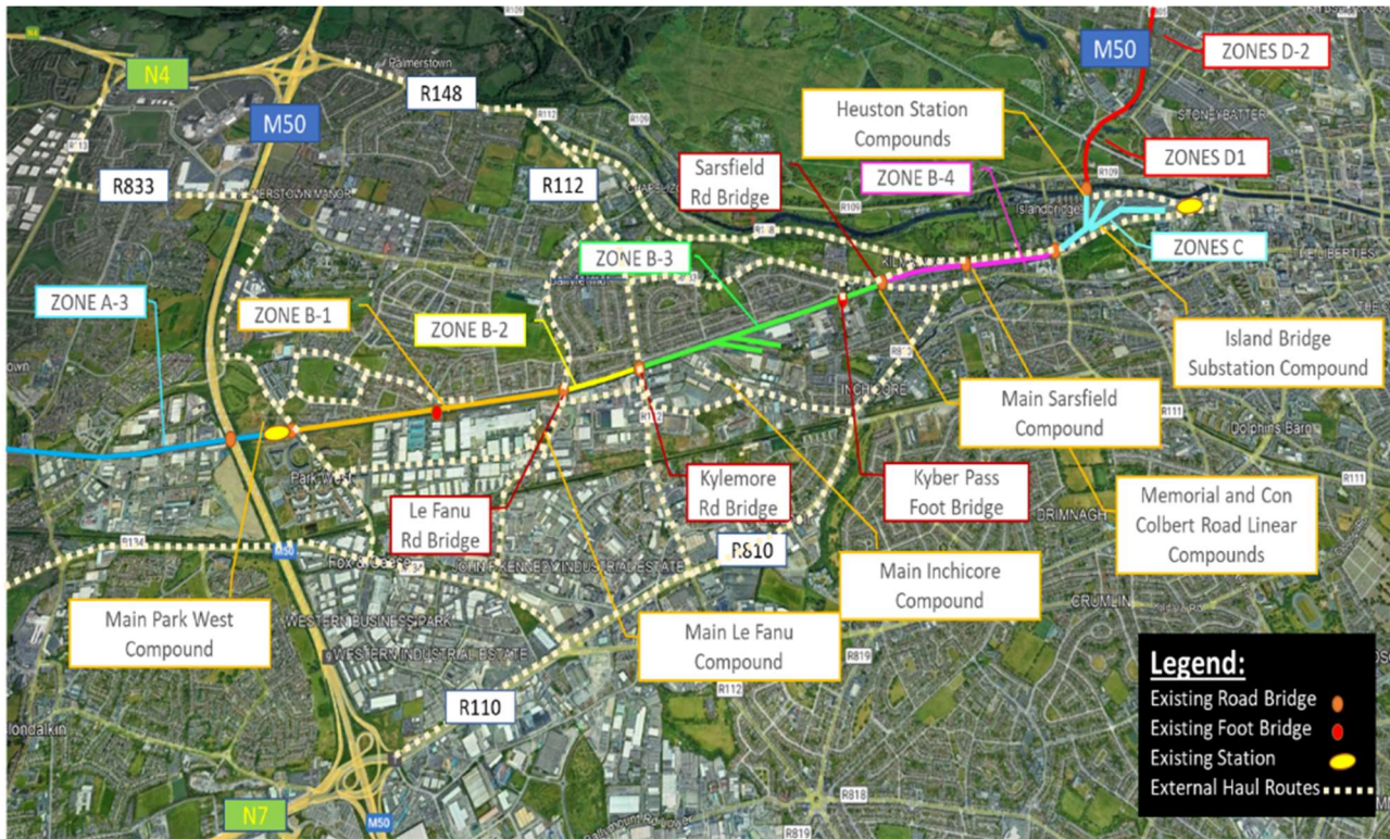
Figure 5-124 Construction Zone B: External Haul Routes
