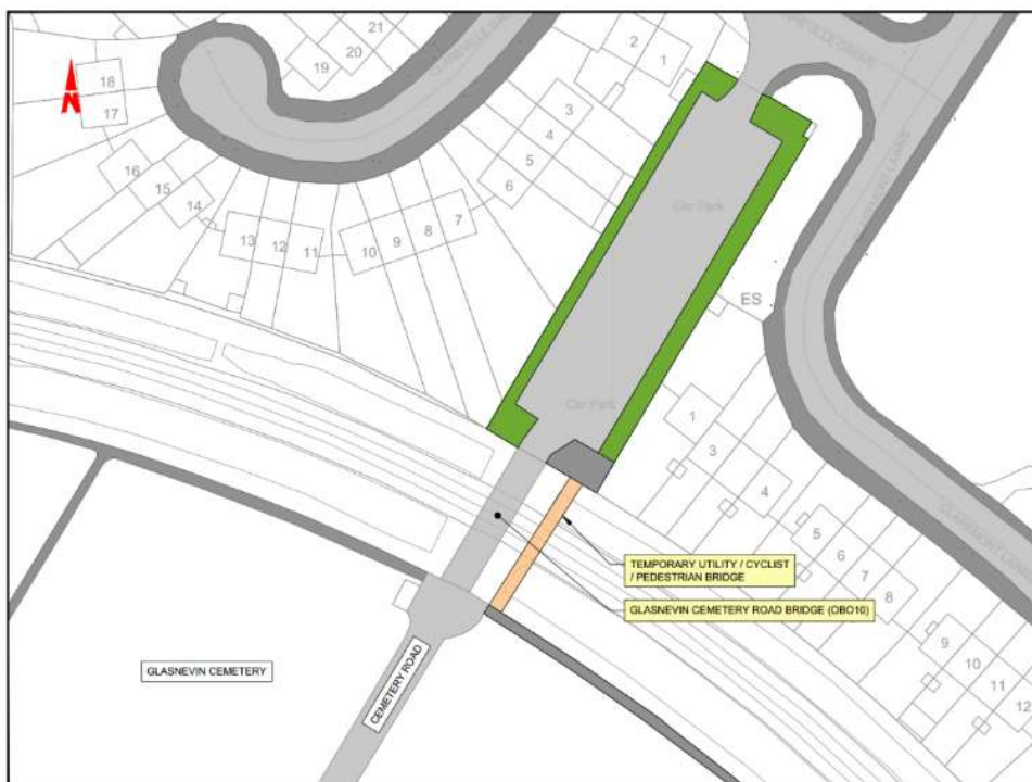
Figure 5-128 Cemetery Road Bridge Works Showing Temporary Utility/ Footbridge
