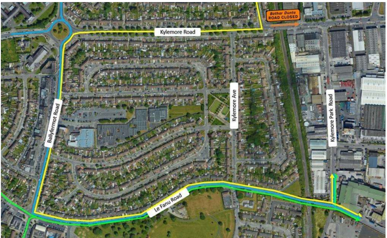
Figure 5-58 Kylemore Southbound Traffic Diversions – Heavy Good Vehicles
