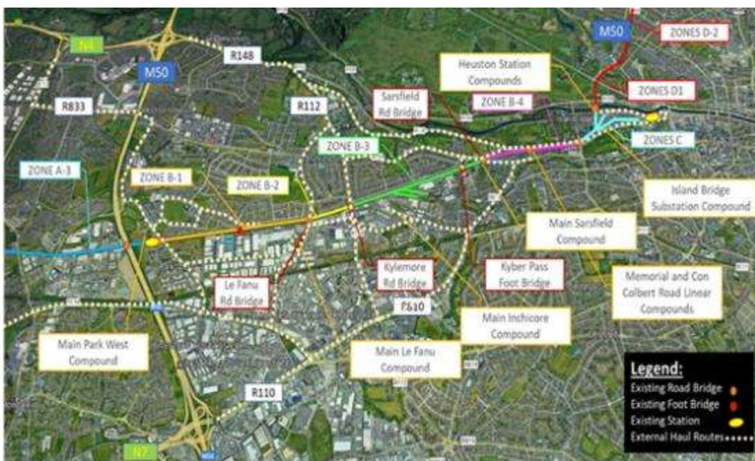
Figure 5-41 Construction Zone B: External Haul Routes
