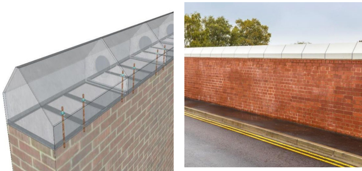
Figure 4-2 Typical Parapet Extension
