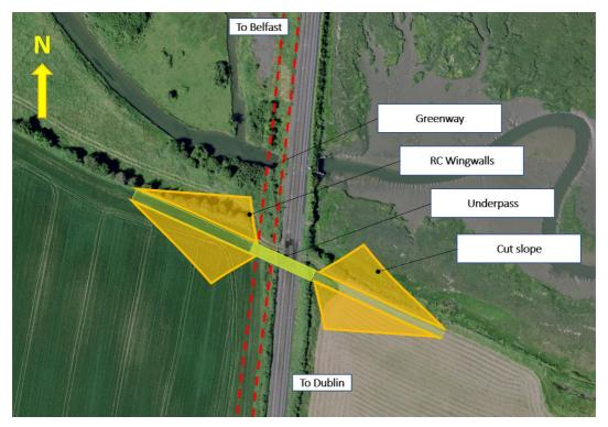
Figure 5-3: Level crossing option 6 underpass layout sketch (Source: OSI aerial mapping)
