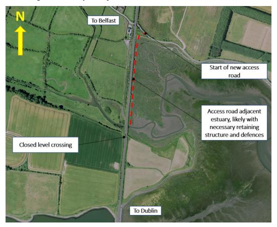
Figure 5-1: Level crossing option 3 access road sketch (Source: OSI aerial mapping)
