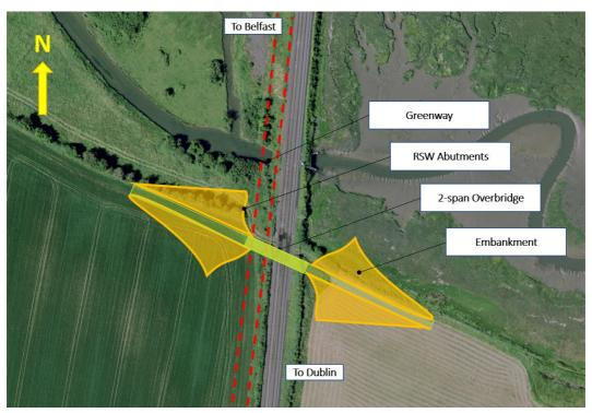
Figure 5-2: Level cross option 5 overbridge layout sketch (Source: OSI aerial mapping)
