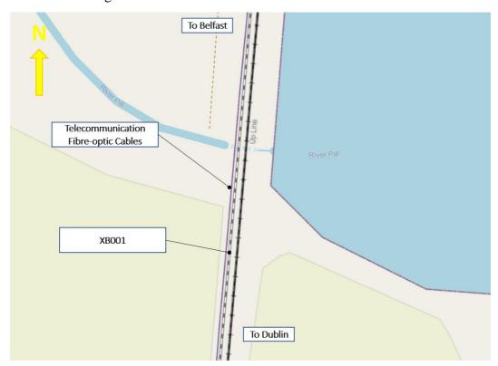
Figure 2-13: Location of utilities close to level crossing XB001
