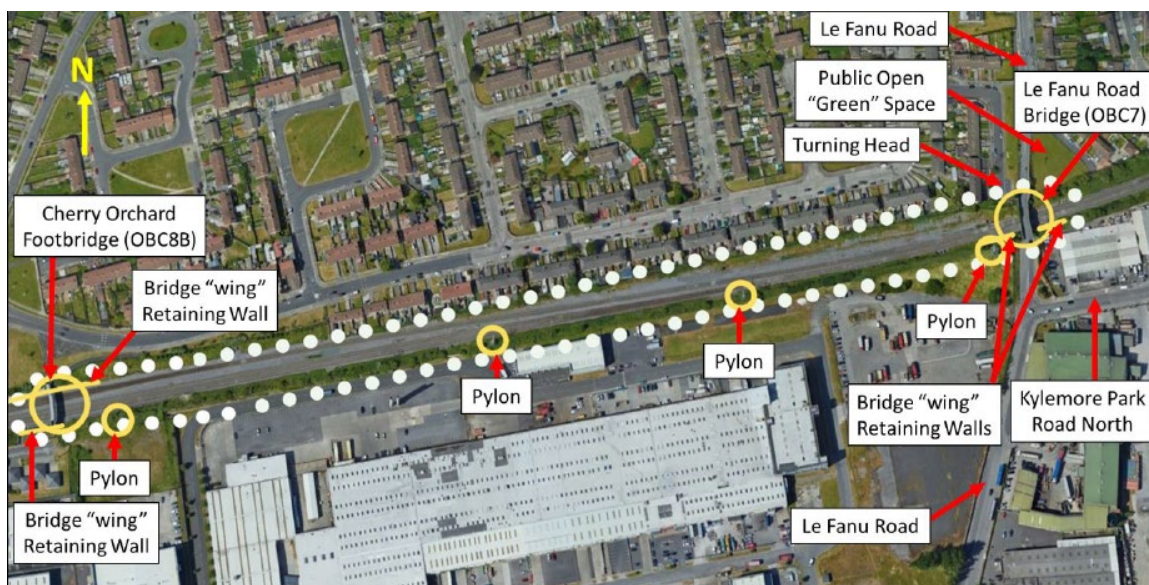
Figure 3-8 Infrastructure Features between Park West & Cherry Orchard Station to Le Fanu Road Bridge
