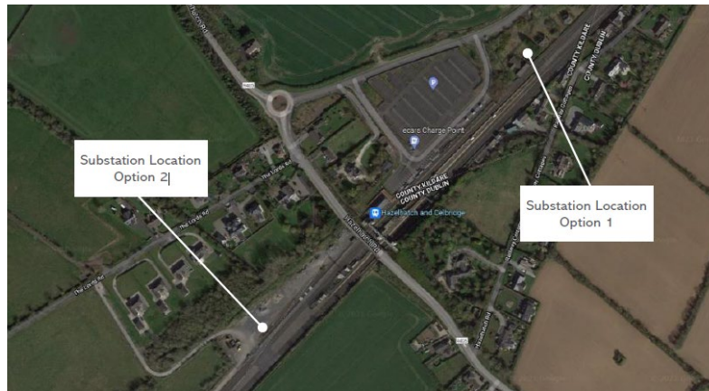
Figure 3-4 Proposed Hazelhatch Substation Locations
