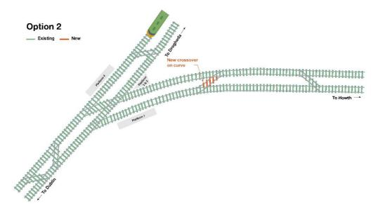
Figure 5-4: Schematic view of Option 2
