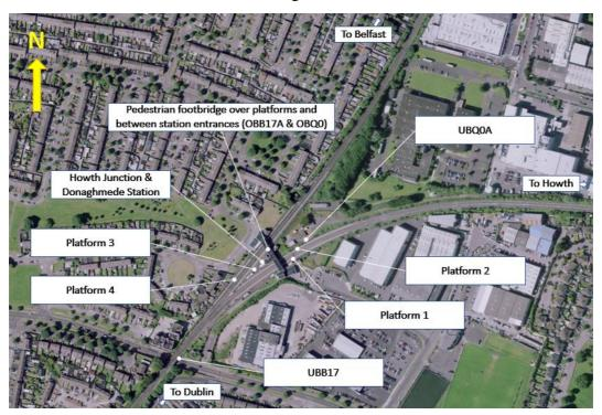
Figure 2-1: Aerial view on Howth Junction & Donaghmede Station (source: OSI aerial mapping)
