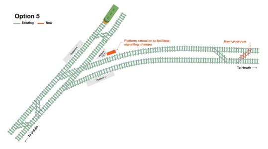
Figure 5-10: Schematic view of Option 5
