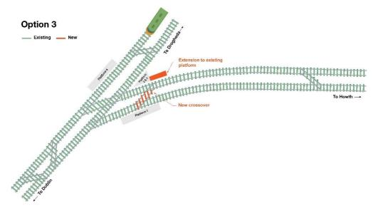
Figure 5-6: Schematic view of Option 3
