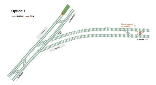
Figure 5-2: Schematic view of Option 1
