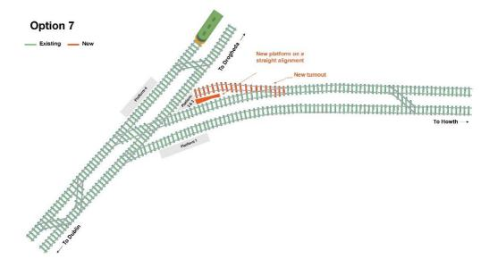
Figure 5-14: Schematic view of Option 7
