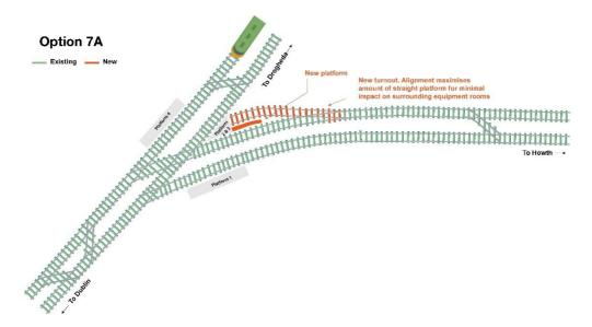
Figure 5-16: Schematic view of Option 7a
